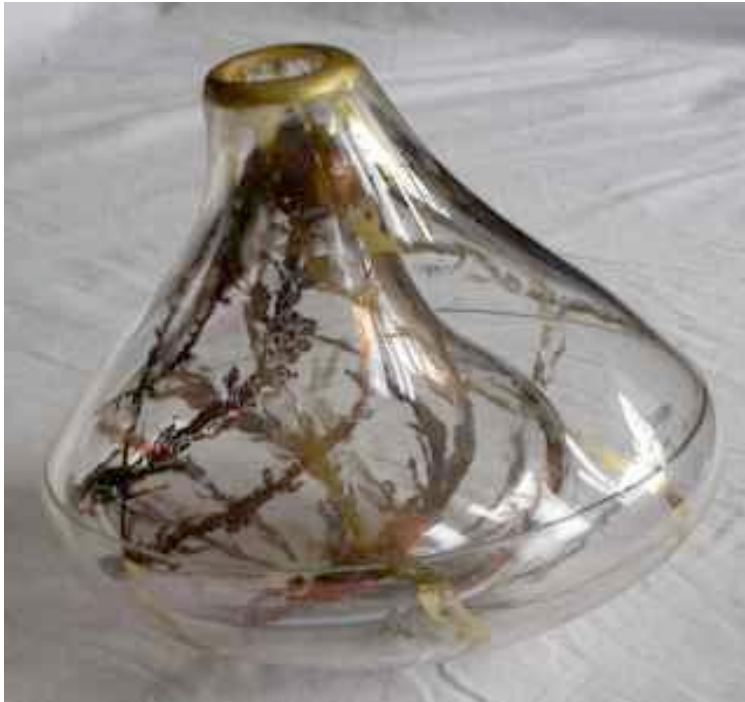
Figure 9 Outer vessel cut open and reassembled to allow placement of smaller one
