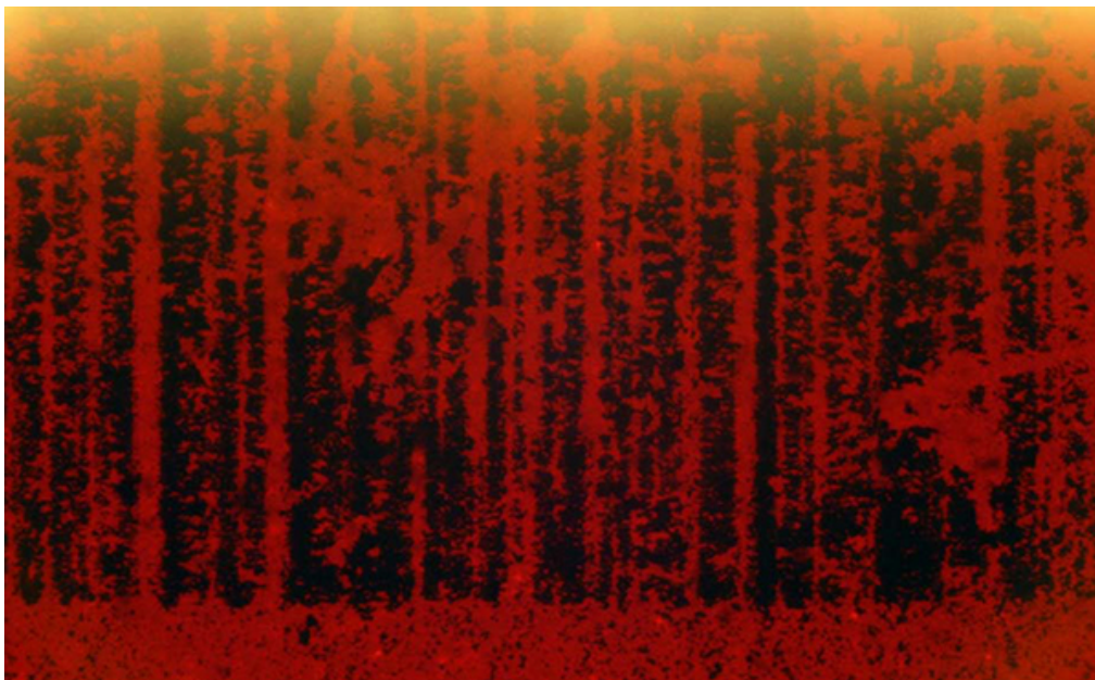
Fig.21. Susan Schuppli, assisted by Christopher Glazowski, PhD, optical engineer, Memorial Sloan-Kettering Cancer Center, New York, June 2011, ‘A magnetic developer containing iron oxide particles was applied to the surface of a copy of the 18 ½ minute gap of Tape 342. This technique, in which sensitized particles cling to residual magnetic traces, replicates one of the original tests performed in 1973, and can reveal the original recording patterns, enabling them to be photographed and analyzed.’, Susan Schuppli, ‘Tape 342: That dangerous supplement’, Cabinet , Issue 43: Forensics (Fall 2011) p.88.
