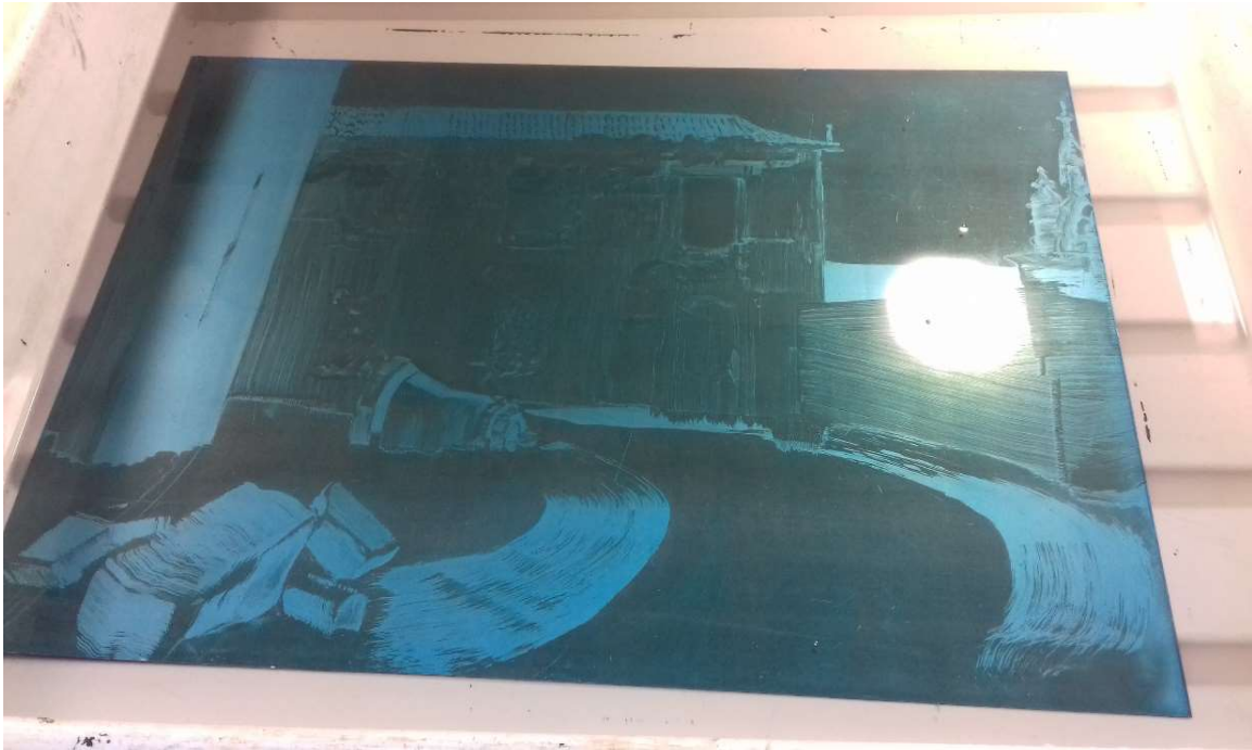
Photoetching. Image appearance on the zinc plates through the acid
