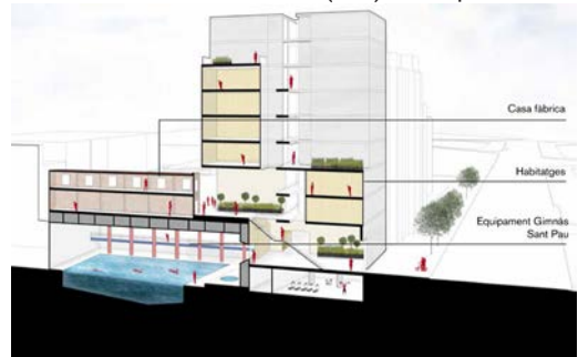
Left: Sant Pau Community Gym's swimming pool was built under the existing house factory in a structural effort. Right: Section of ATRI Sant Pau.
