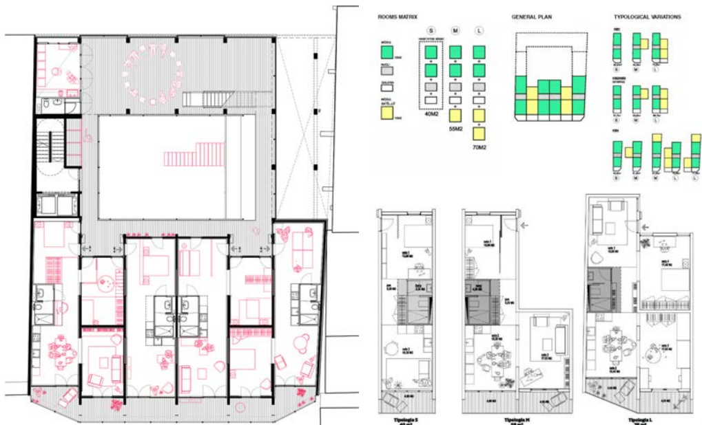
La Borda typical plan and housing units system. Bottom right: housing units layout as derived from consensus co-design workshops: S, M, L sizes.
