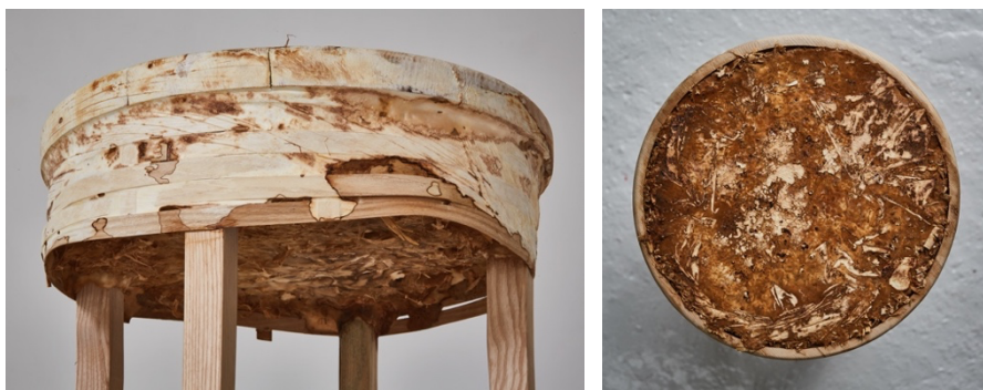
Figure 27. Two mycelium stools made using green wood waste bound with mycelium to a wooden base and legs. © Petr Krejci
