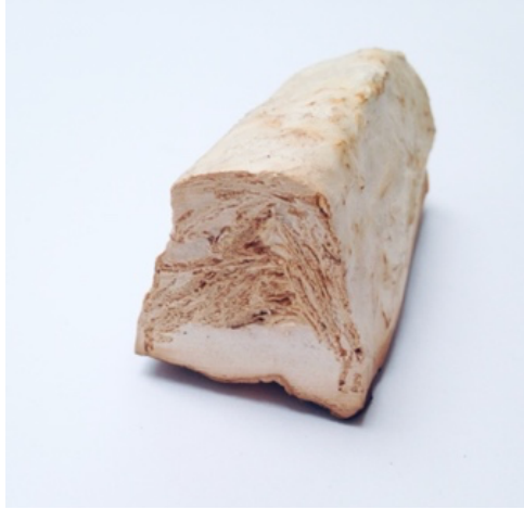
Figure 25. A cross-section of moulded component illustrating different properties of the composite material. © Author's archive
