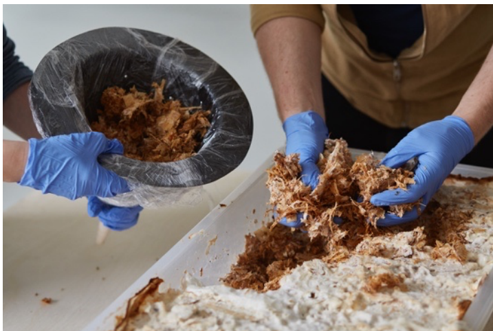
Figure 24. Preparation of light shade formers filled with 'myceliated' wood for a second growth phase. © Petr Krejci
