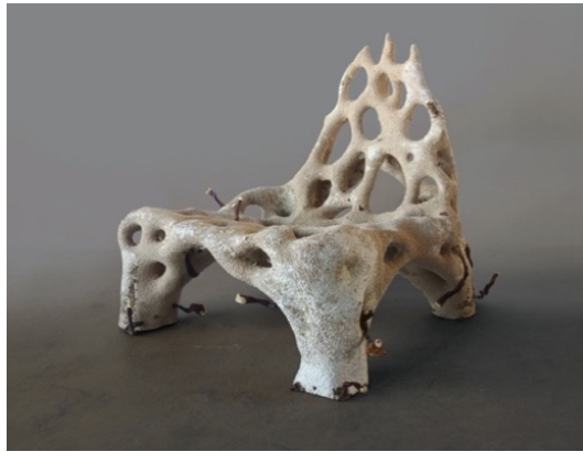
Figure 14. Mycelium chair made using the improved 3D printing process, exhibited at the Centre Pompidu, Paris (2019). © Klarenbeek & Dros
