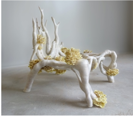
Figure 13. Mycelium chair made using an adapted 3D printing process by Eric Klarenbeek. © Klarenbeek & Dros
