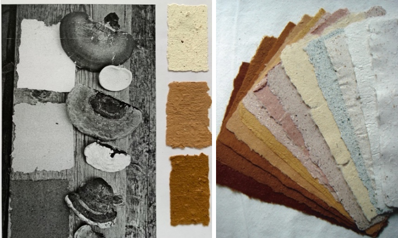
Figure 6. Paper swatches produced from Piptoporus betulinus , Fomitopsis pinicola and Fomes fomentarius . © Johansson, 2002 (left) and Mushroom paper created from various species © Johansson, 2016 (right)
