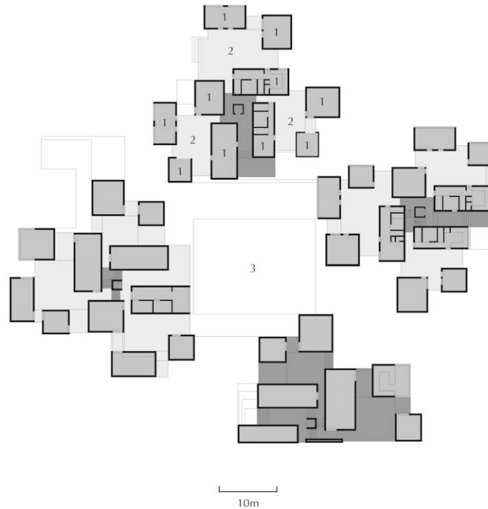
Fig. 9: Typical neighbourhood plan showing the relationships between four dwelling clusters. Oswald Mathias Ungers, competition entry for Cologne Neue Stadt (1962). Key: 1 – room, 2 – living room, 3 – urban square. Redrawn by the authors.
