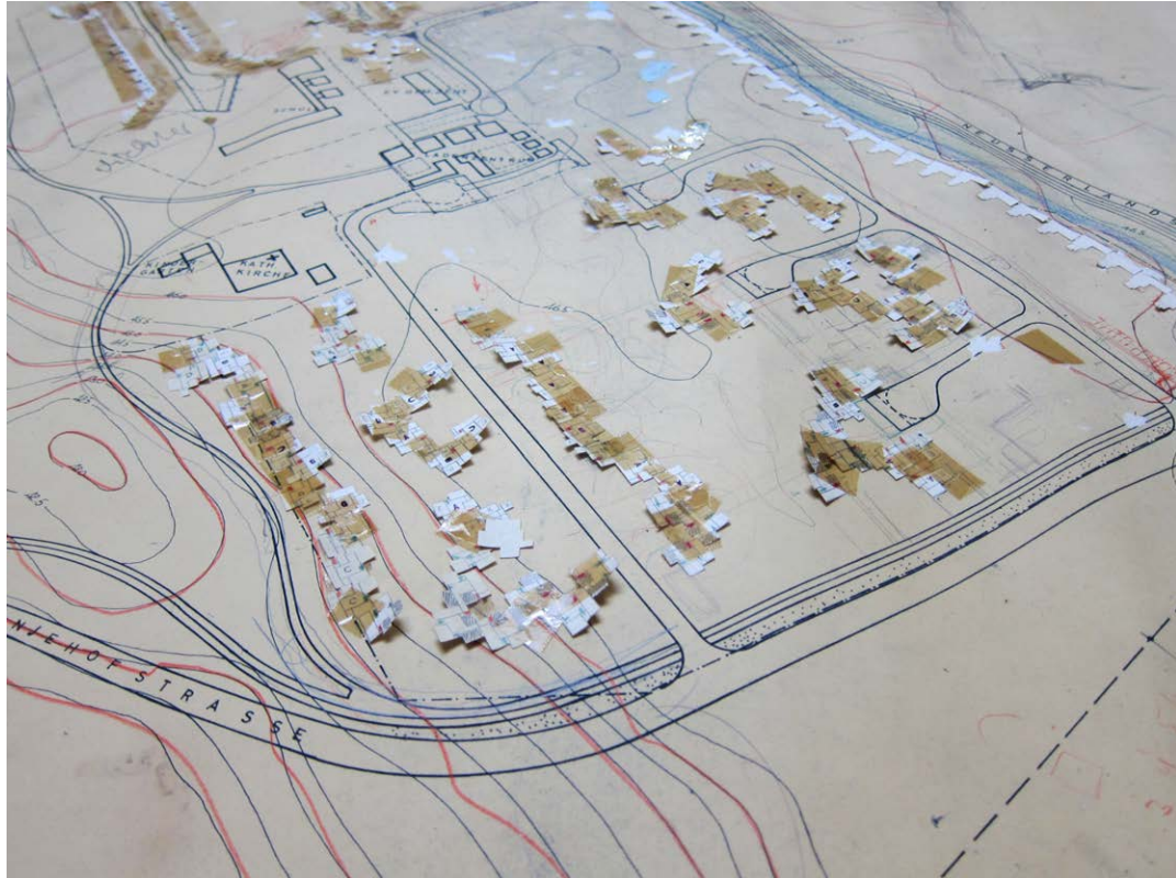
Fig. 7: Urban plan studies. Cut-out dwelling plan clusters provisionally taped to a typographic plan of the development site (including streets and structures to be retained). Oswald Mathias Ungers, competition entry for Cologne Neue Stadt (1962).
