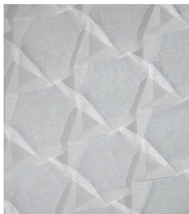
Fig 61. Moulded hexagonal fold coated silk- organza, sample 17.
