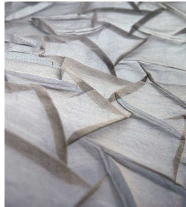
Fig 57. Moulded polyester, using Alex Bateman's pattern '3.6.3.6 tessellation 22.5 degrees 3 scaling', sample 14.
