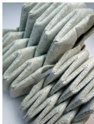
Fig 104. Laser scored filtration felt, sample 43, 2008.
