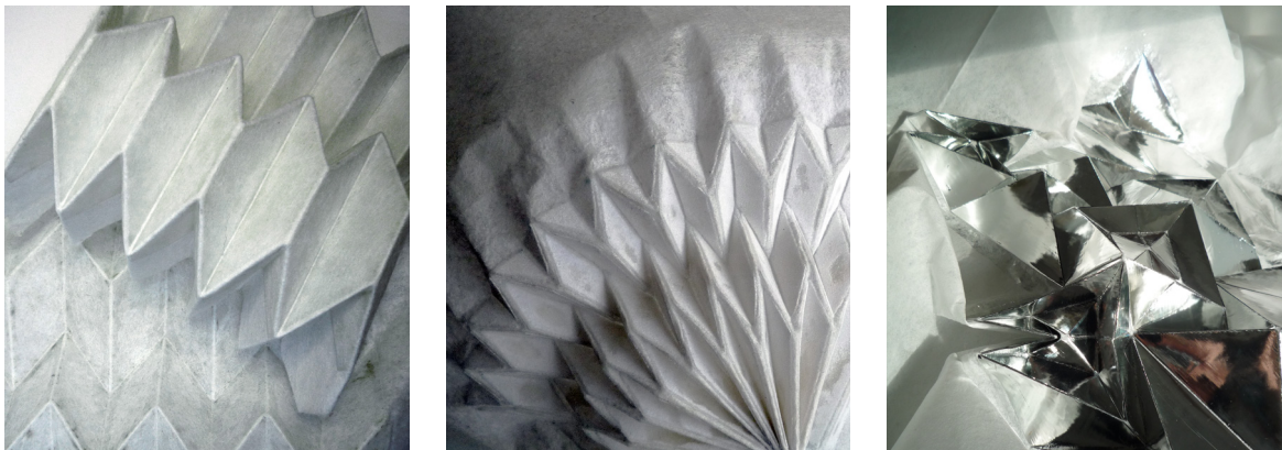
Fig 107. Immobile and mobile 'Ha ori' fold samples, fused polypropylene and polyester, samples 47 & 52, 2008.
