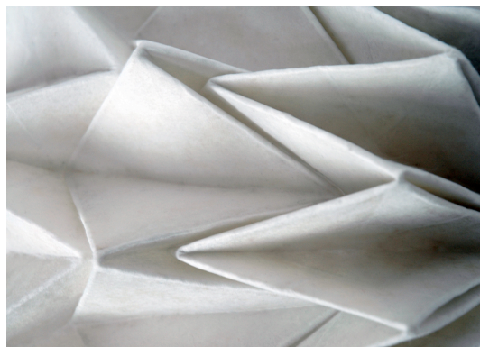
Figure 5: Origami folded textile with laser cut, laminated areas.
