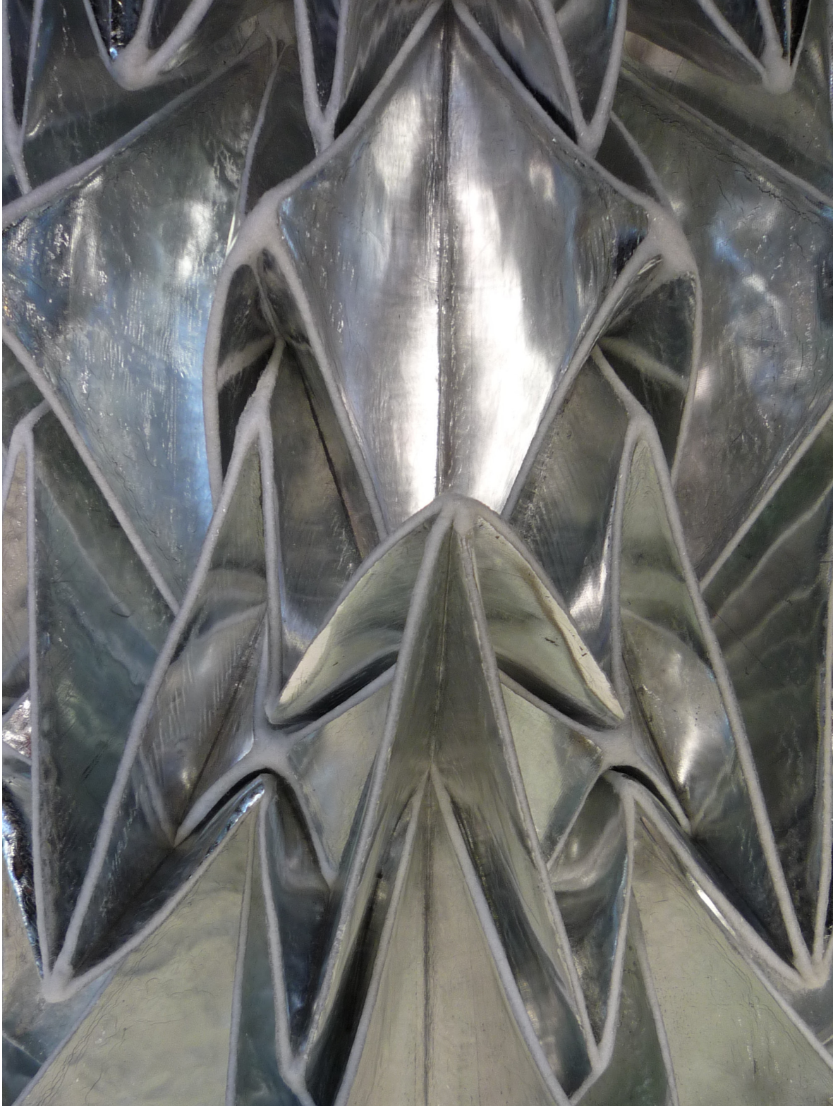
Fig 115. Foiled fused polypropylene and polyester, sample 105, 2009.
