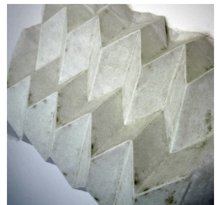
Fig 105. Laser scored filtration felt, sample 43 (bottom) and with slight misalignment in registration, sample 44 (top), 2008.
