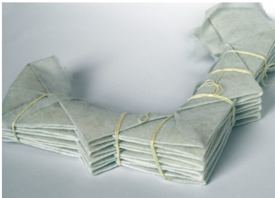
Fig 113. Polypropylene and polyester, closed sample 82 tied ready for heat setting, 2009.
