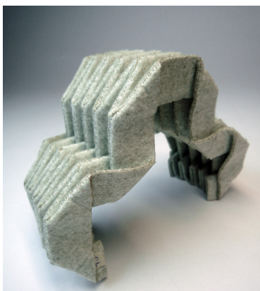
Fig 104. Laser scored filtration felt, sample 43, 2008.
