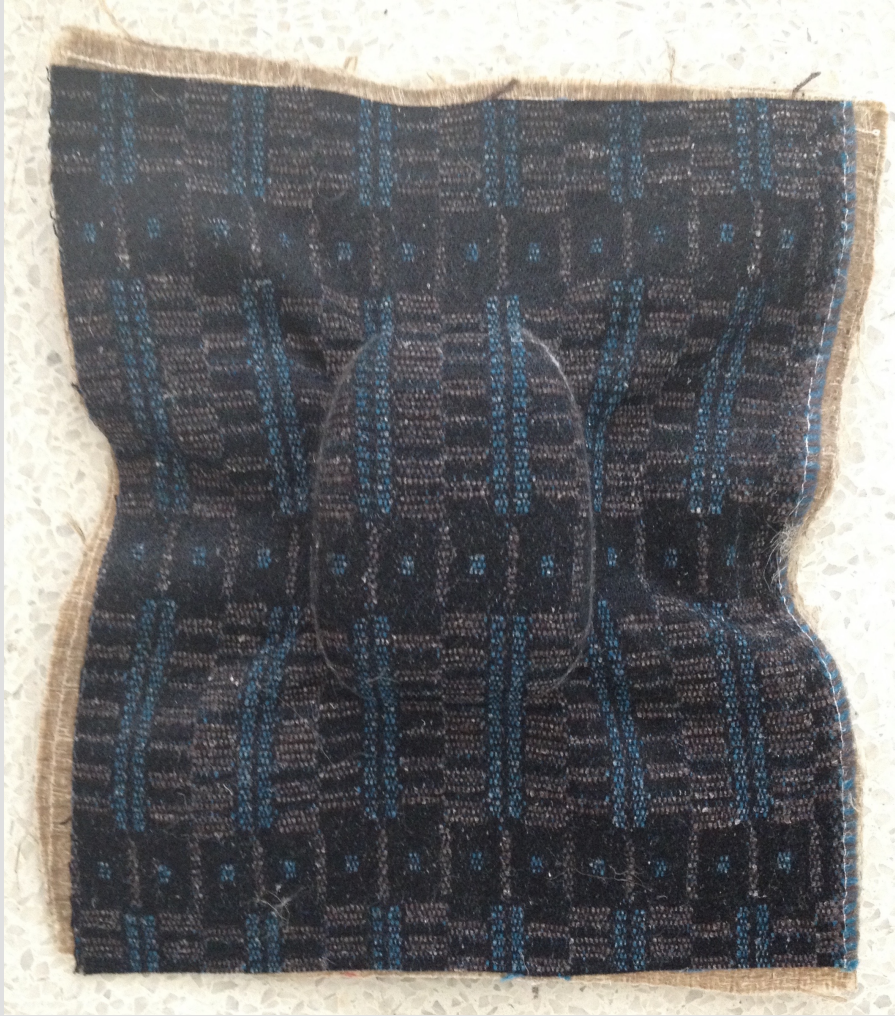
Repeat Deco design, wool/nettle woven textile with Biotex, formed in pobble mould
