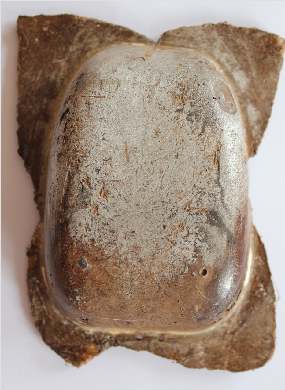
Face of bio-resin and aluminium powder with non-woven flax reinforcement, made using pobble mould
