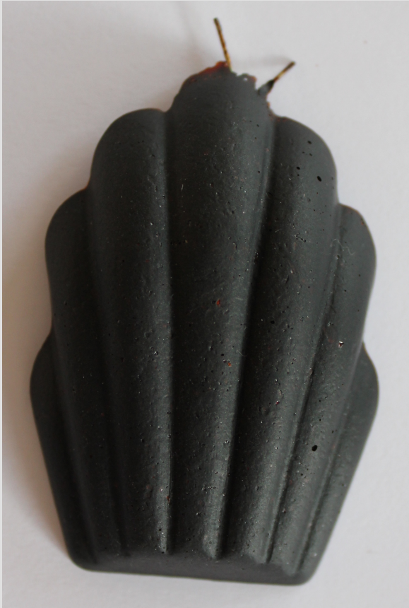
Face of bio-resin with LED, made in silicon madeleine mould
