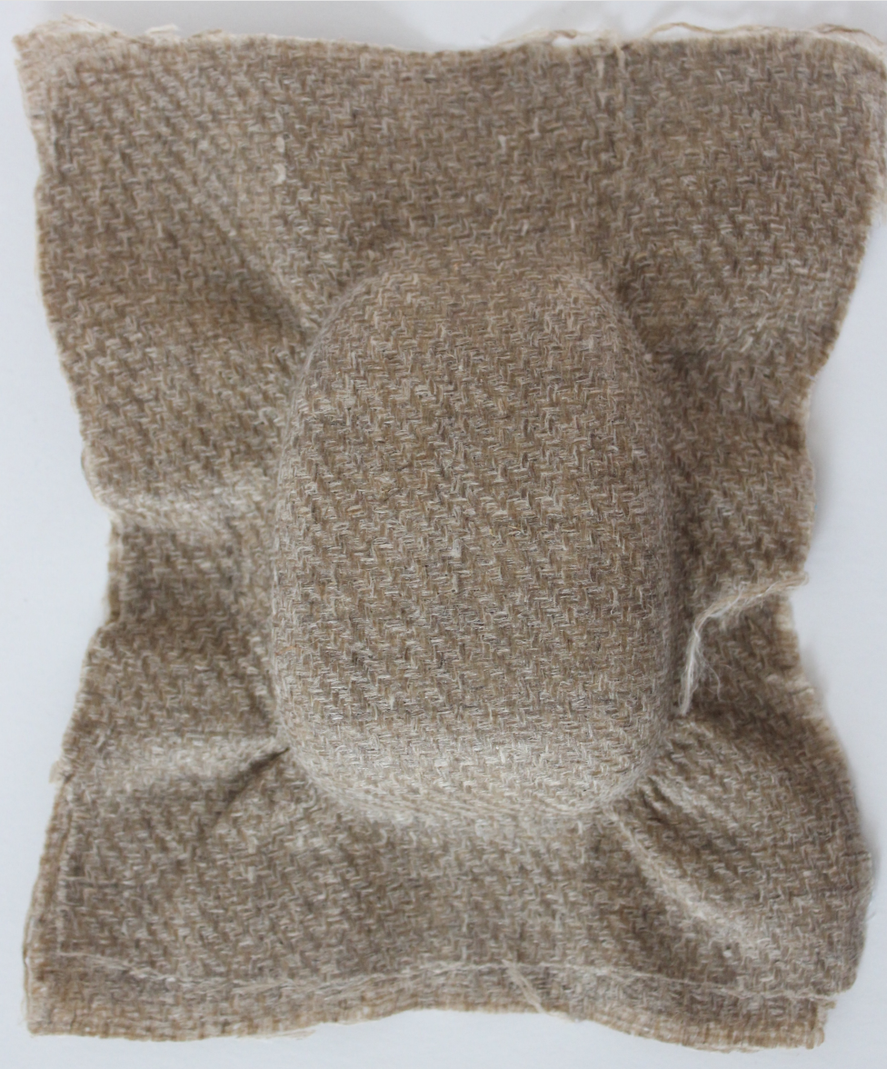
Biotex twill weave structure, formed in pobble mould
