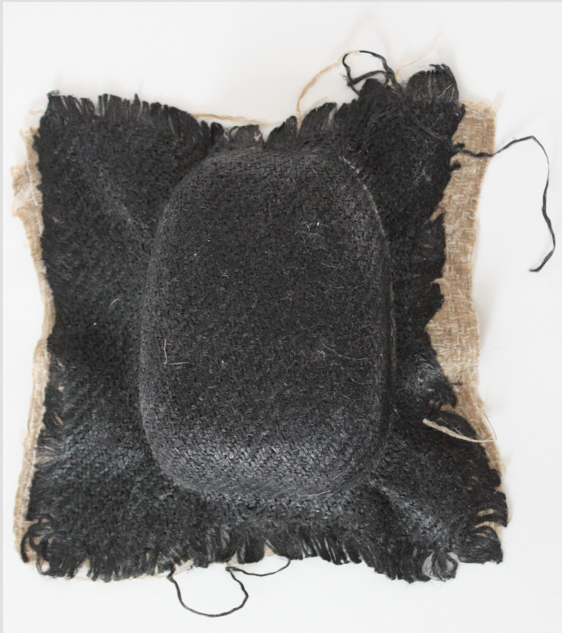
Biotex twill weave, dyed black and formed in pobbles mould
