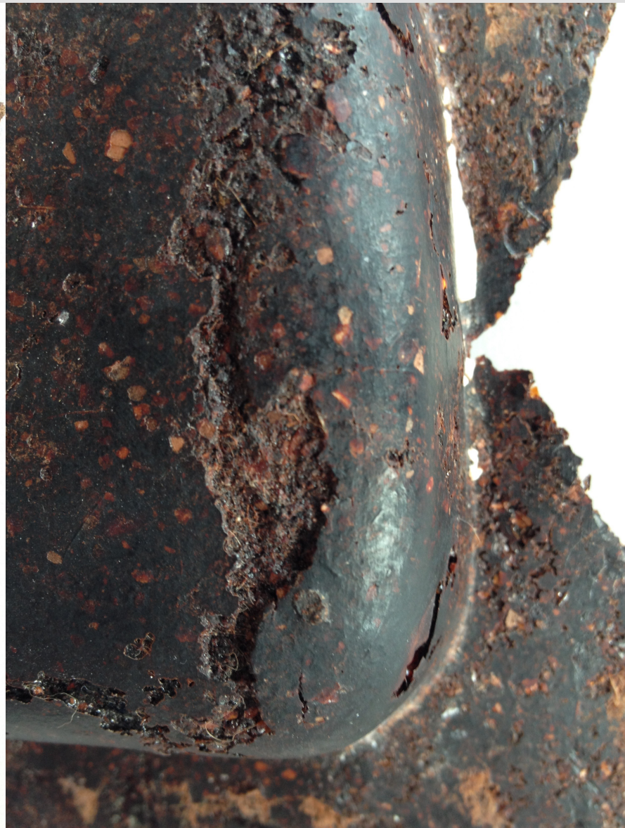
Detail of face of bio-resin with cocoa shell, made using pobble mould
