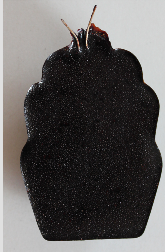
Rear of bio-resin, with LED made in silicon madeleine mould
