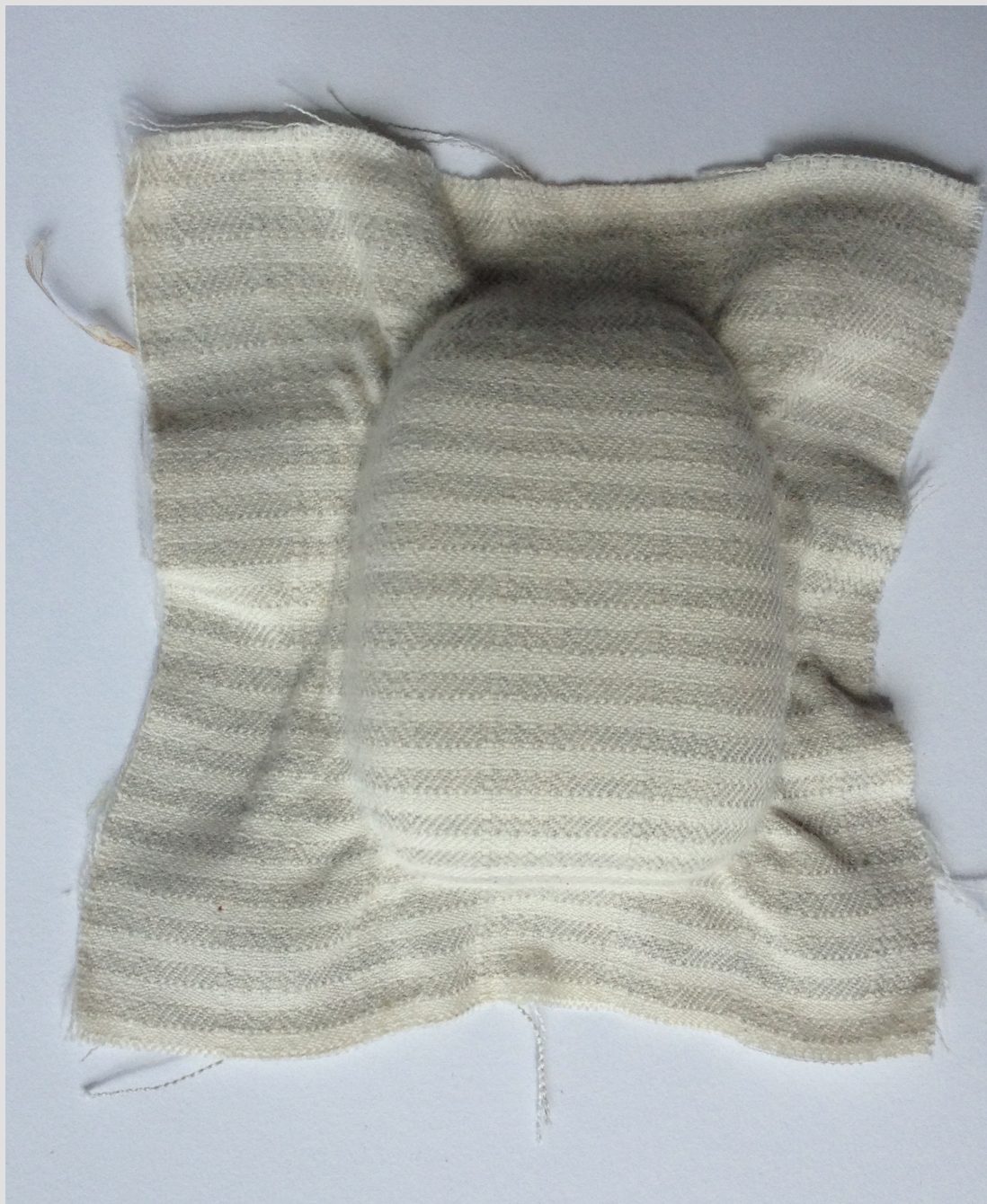
Woven wool textile and Biotex, formed in pobble mould
