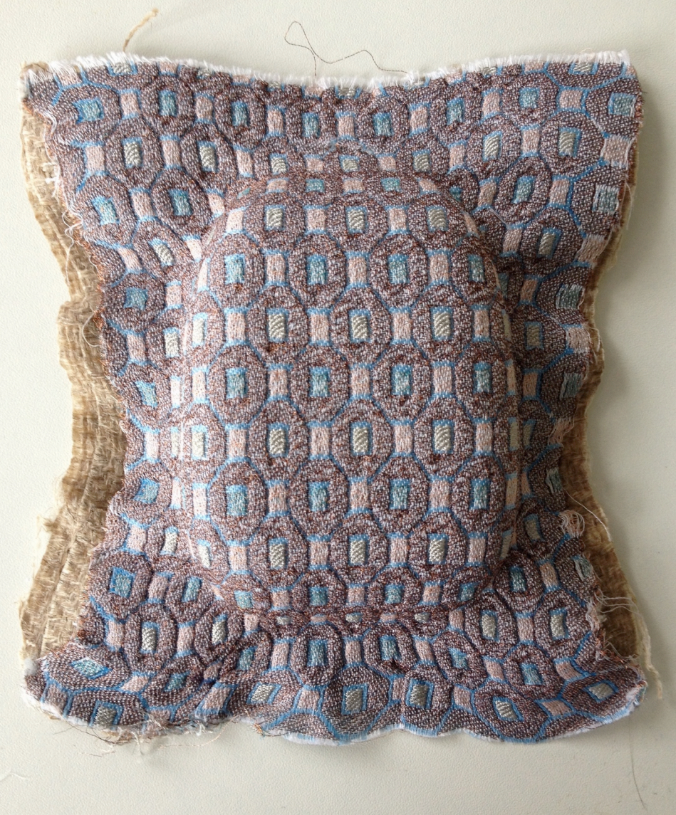
Woven metal and polypropylene textile with Biotex, formed in pobble mould
