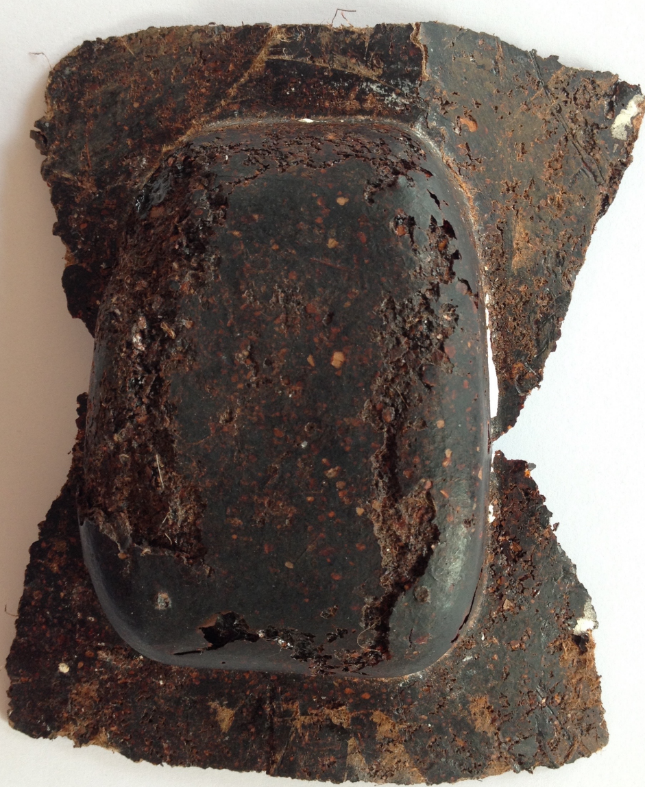
Face of bio-resin with cocoa shell, made using pobble mould
