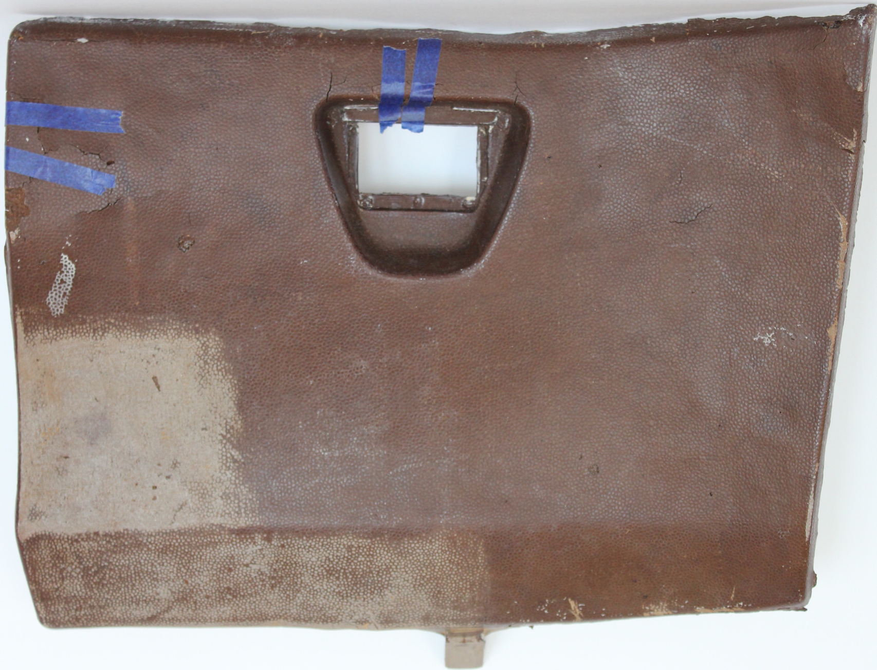
Glove-box lid made with bio-resin and aluminium powder, partly sanded in left corner
