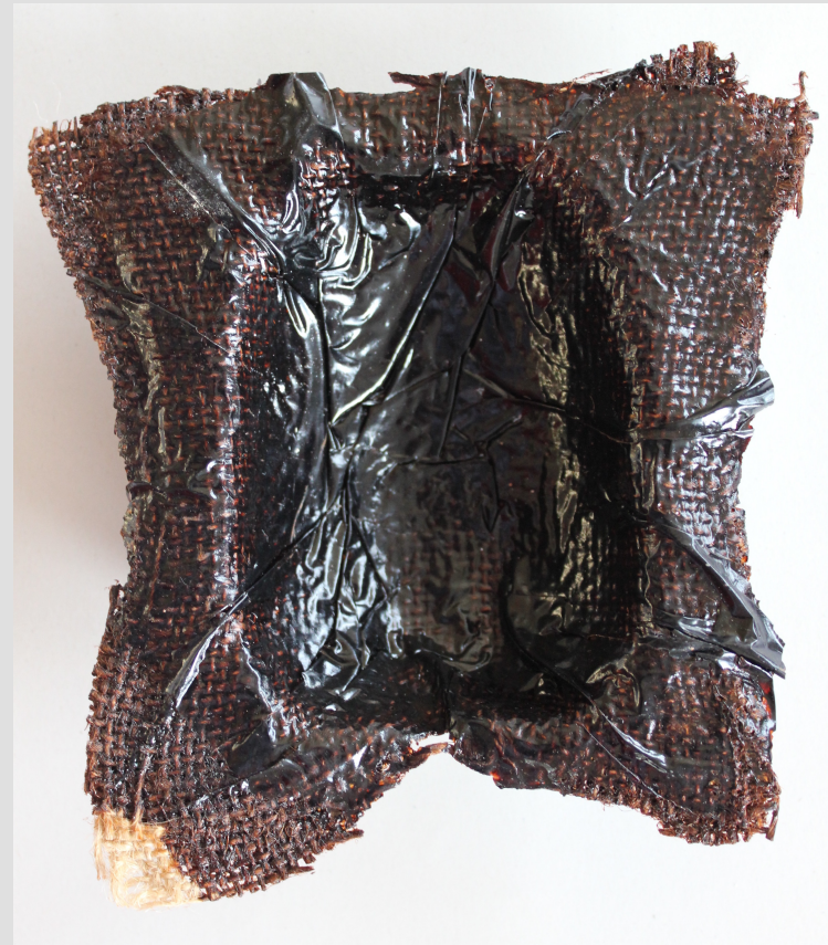
Rear face of bio-resin and jute coffee sack, made using pobble mould
