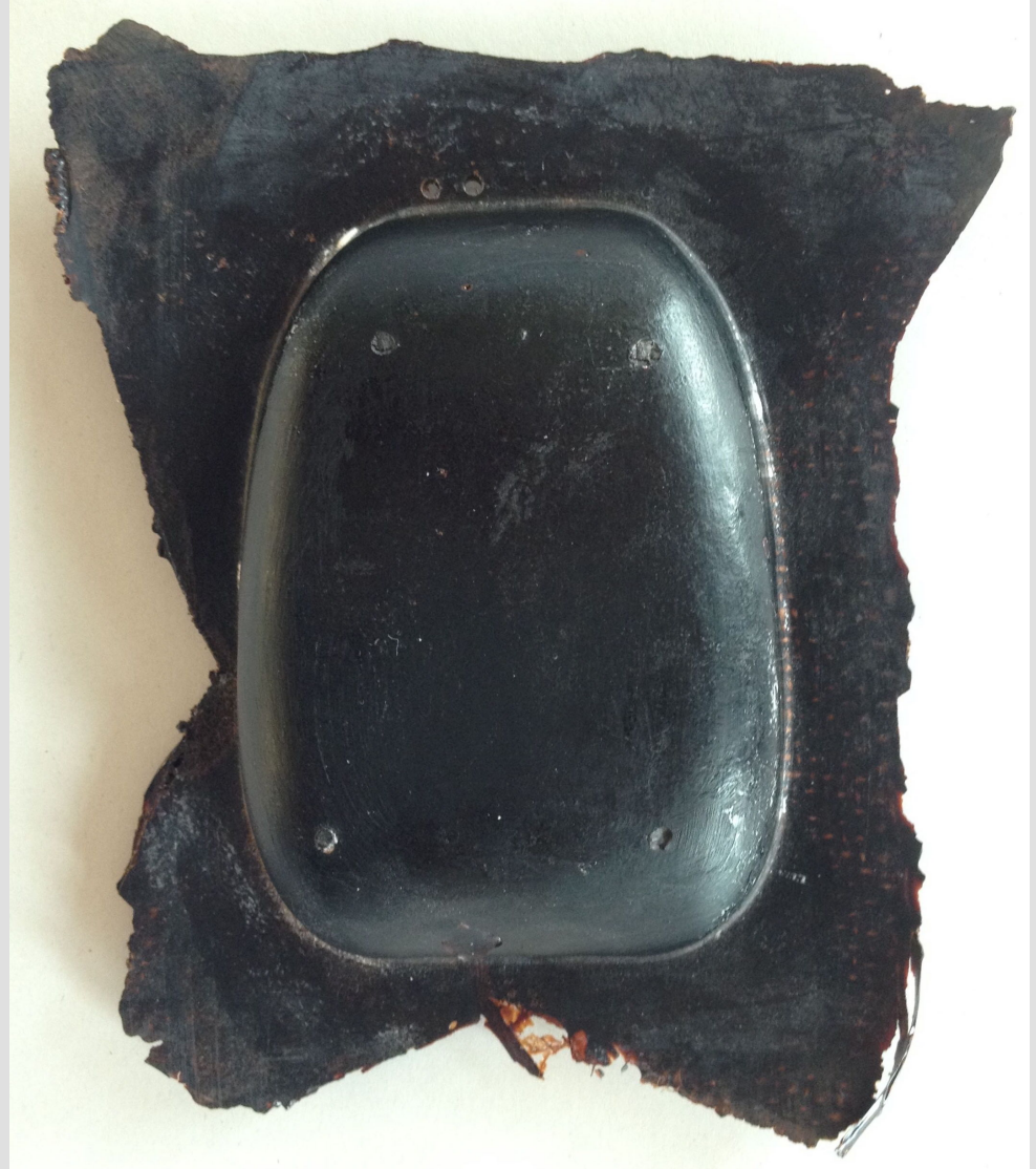
Face of bio-resin with jute sacking reinforcement, made using pobble mould
