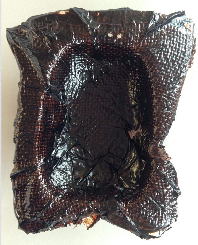
Rear side of bio-resin and jute sacking, made using pobble mould
