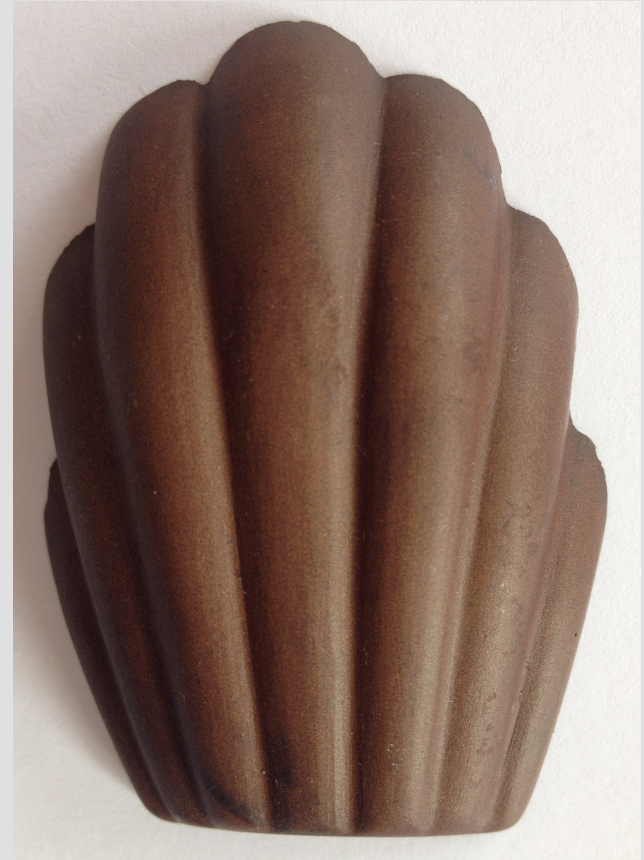
Face of bio-resin and aluminium powder made in silicon madeleine mould
