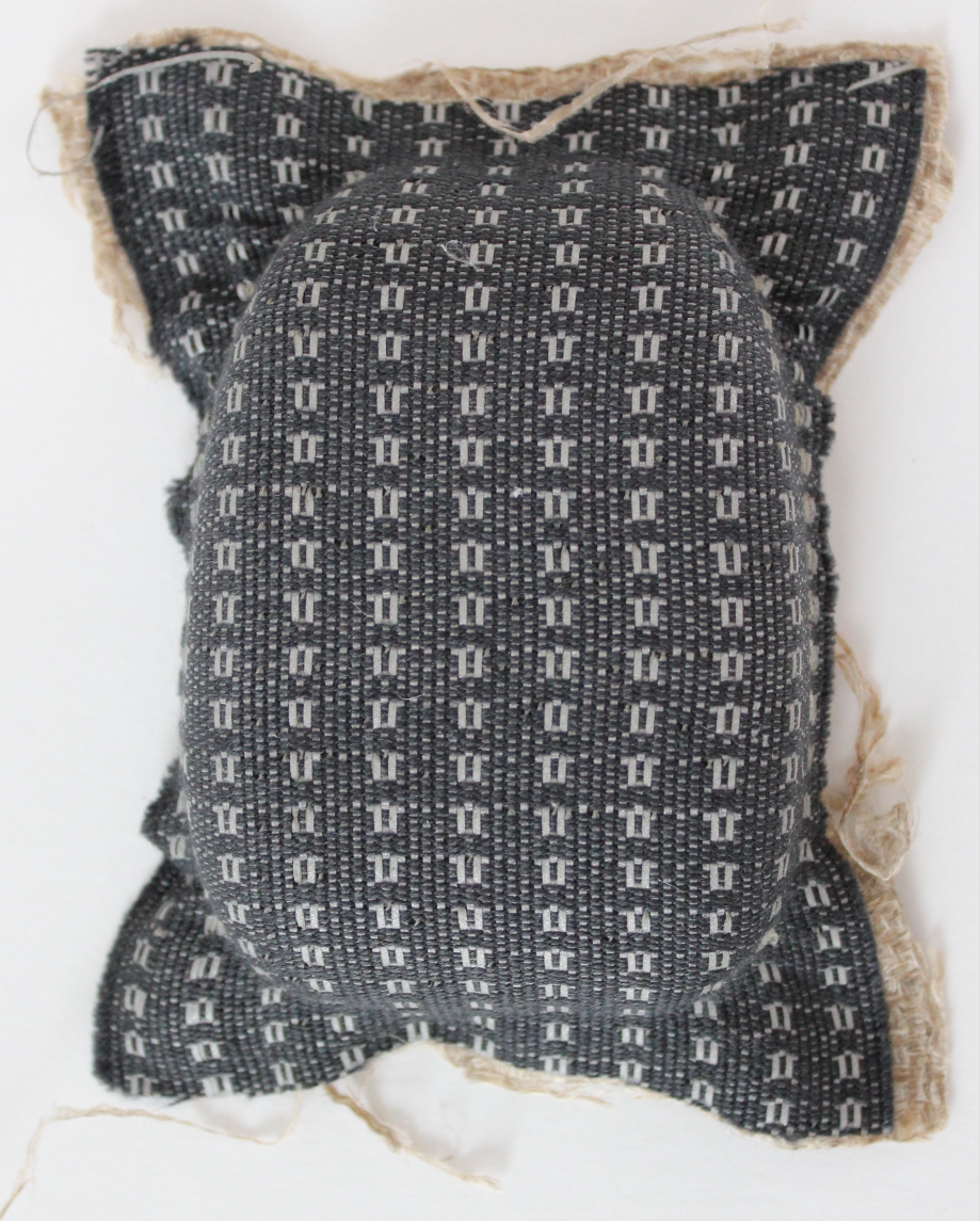
Woven reflective and wool textile with Biotex, formed in pobble mould
