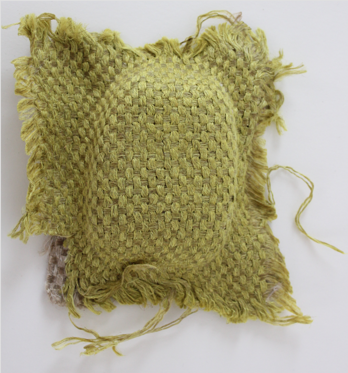
Biotex hopsack weave, dyed yellow and formed in pobble mould
