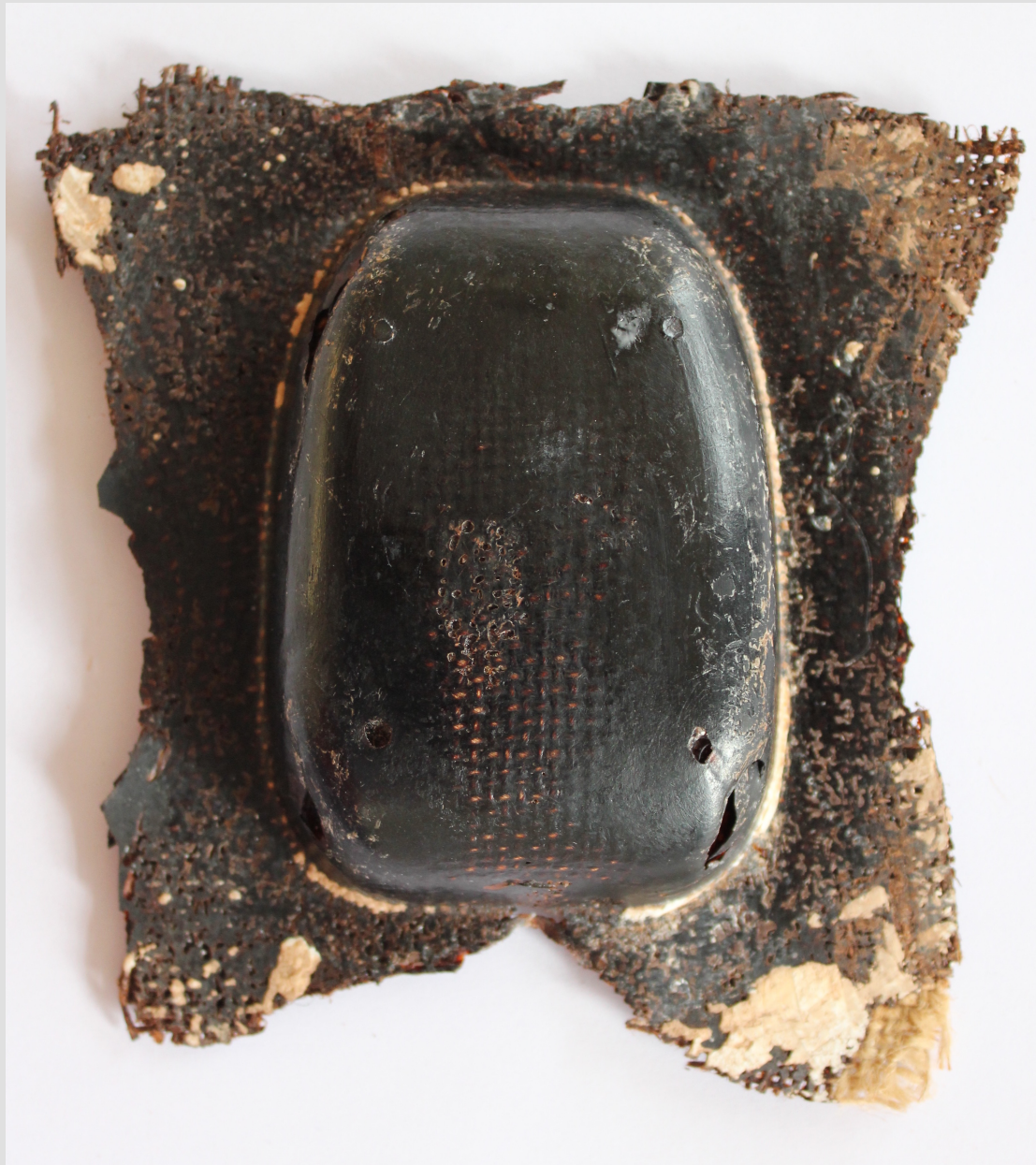
Face of bio-resin with jute coffee sack reinforcement showing plaster from mould, made using pobble mould
