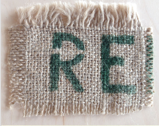
Waste jute sacking from imported coffee beans used as reinforcement material
