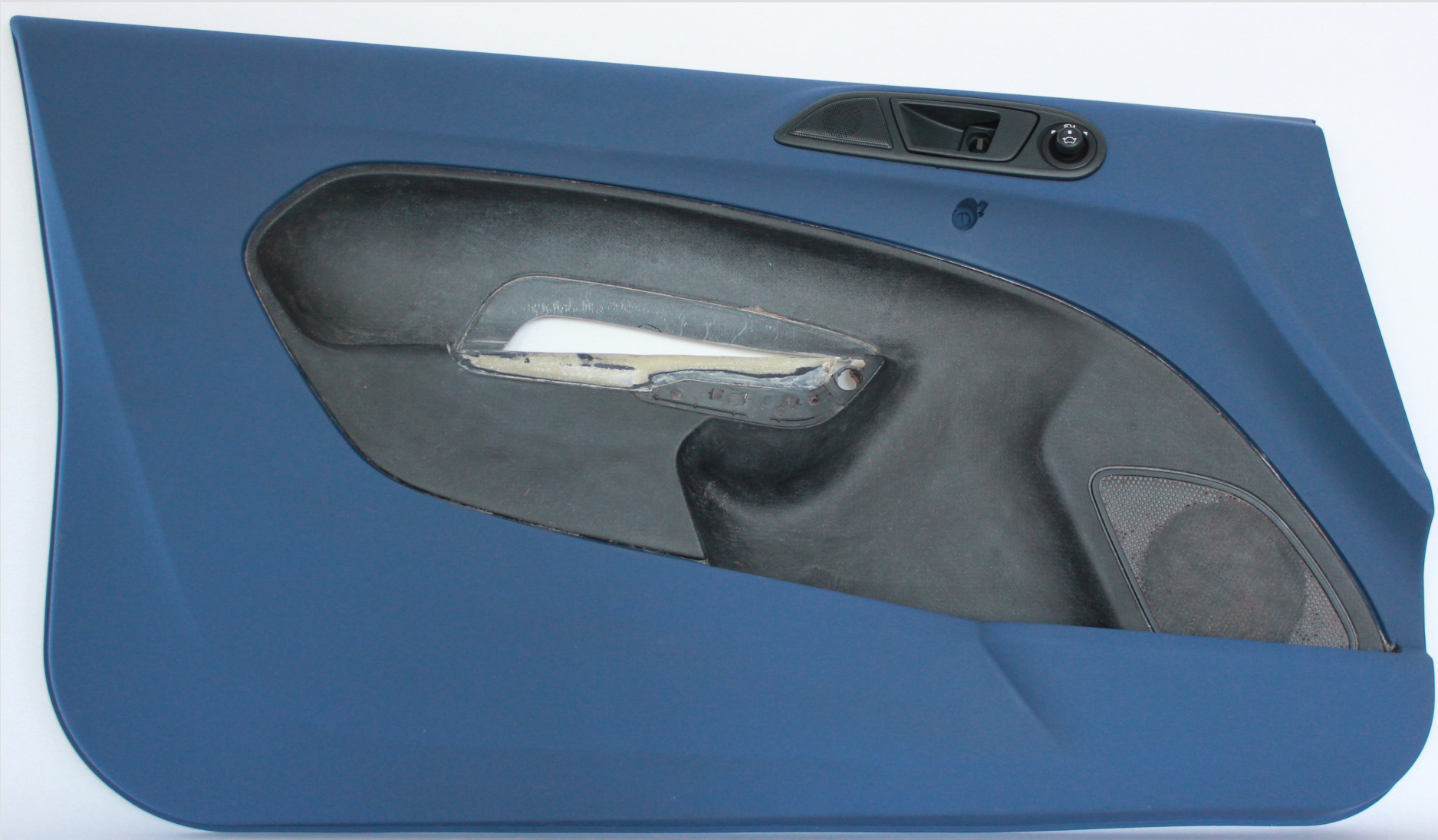
Door panel: inner part bio-resin, Nextel painted outer part
