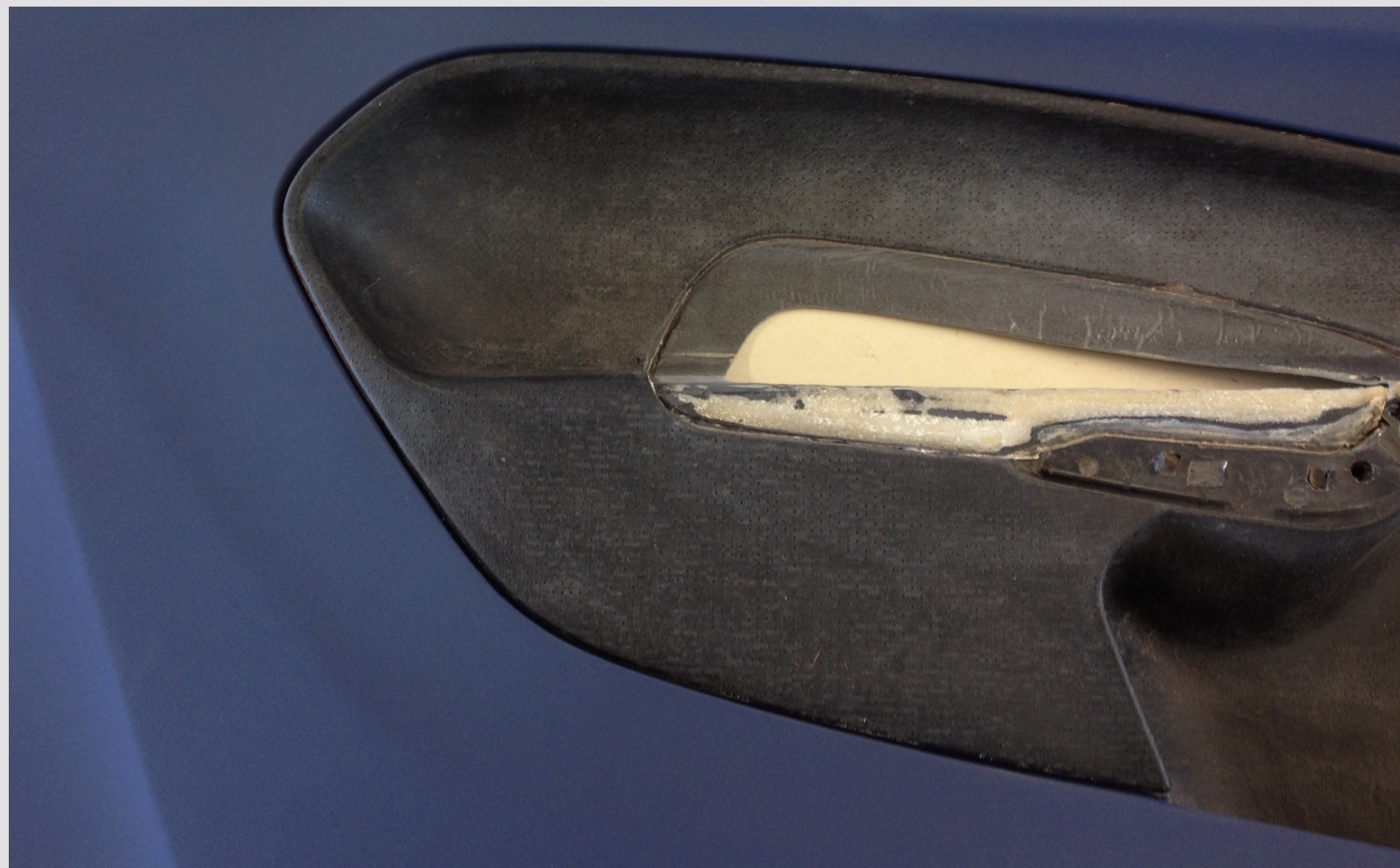
Close up of bio-resin inner inner door panel part, and Nextel painted outer door panel part
