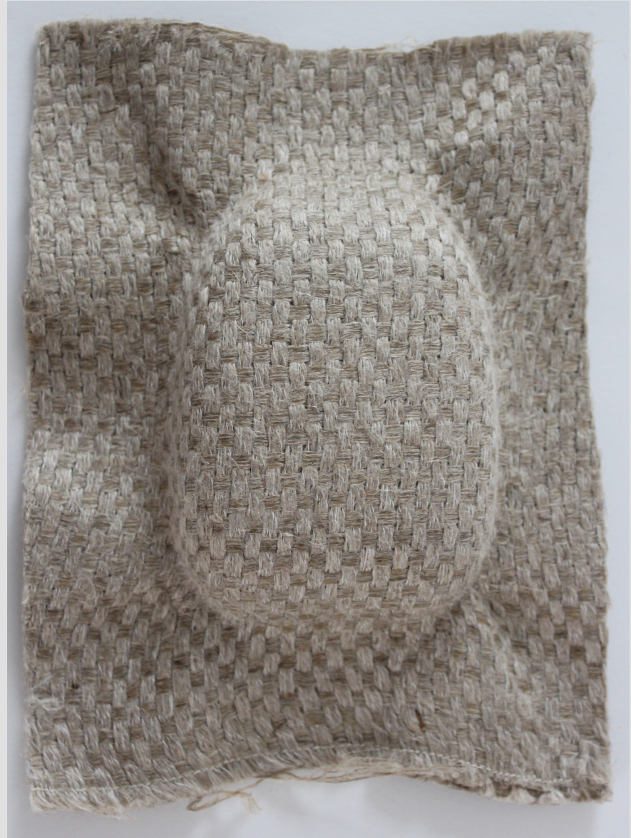
Biotex hopsack weave structure, formed in pobble mould
