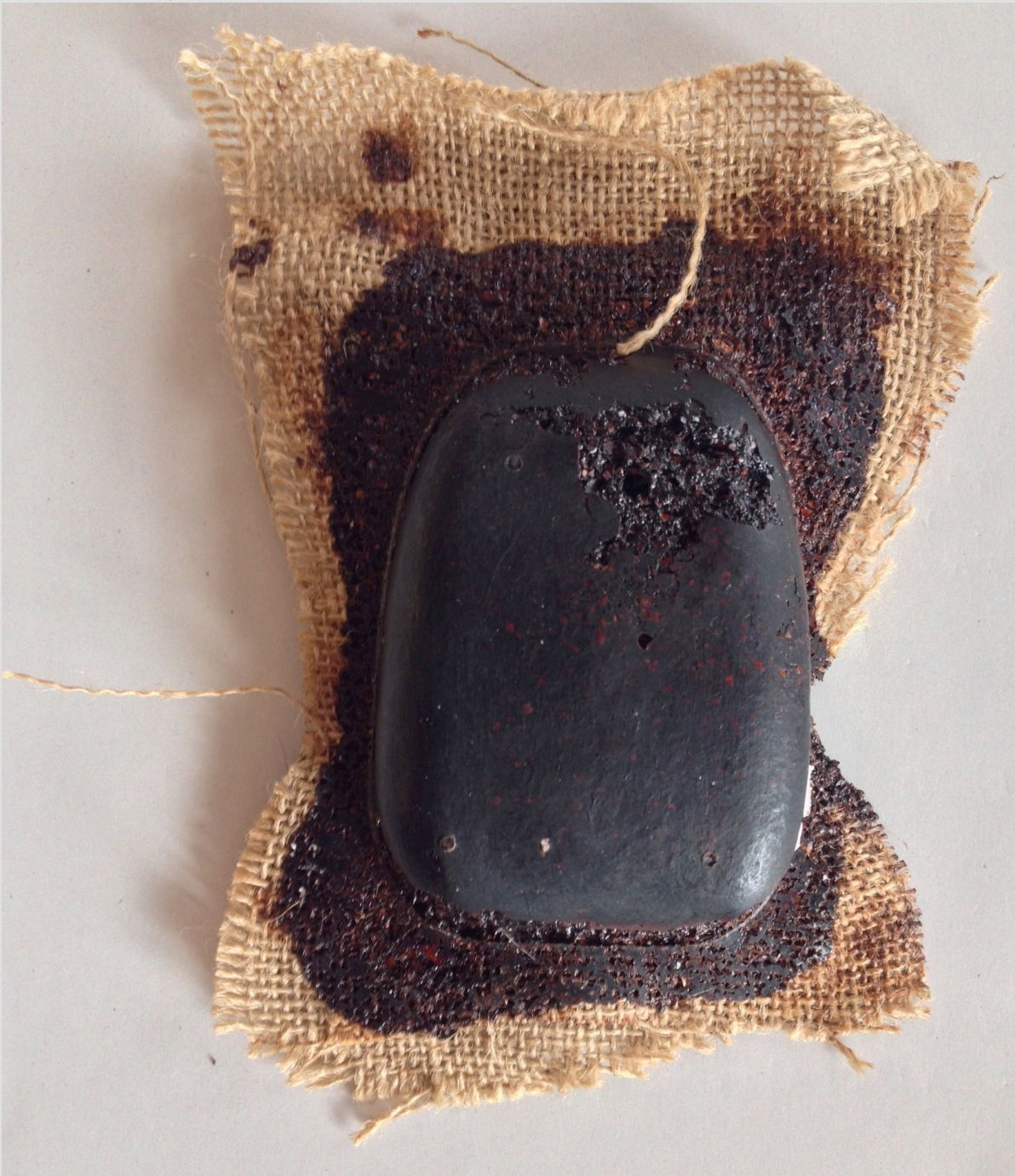
Bio-resin and jute coffee sack, made using pobbles mould
