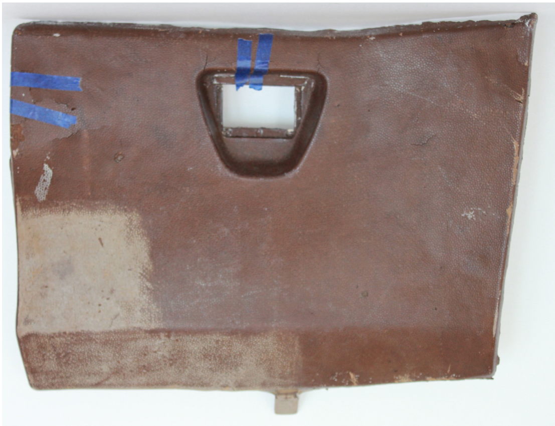
Figure 30: Glove-box lid made with bio-resin, aluminium powder, and ground cocoa shell; seen partially sanded in lower left part.
