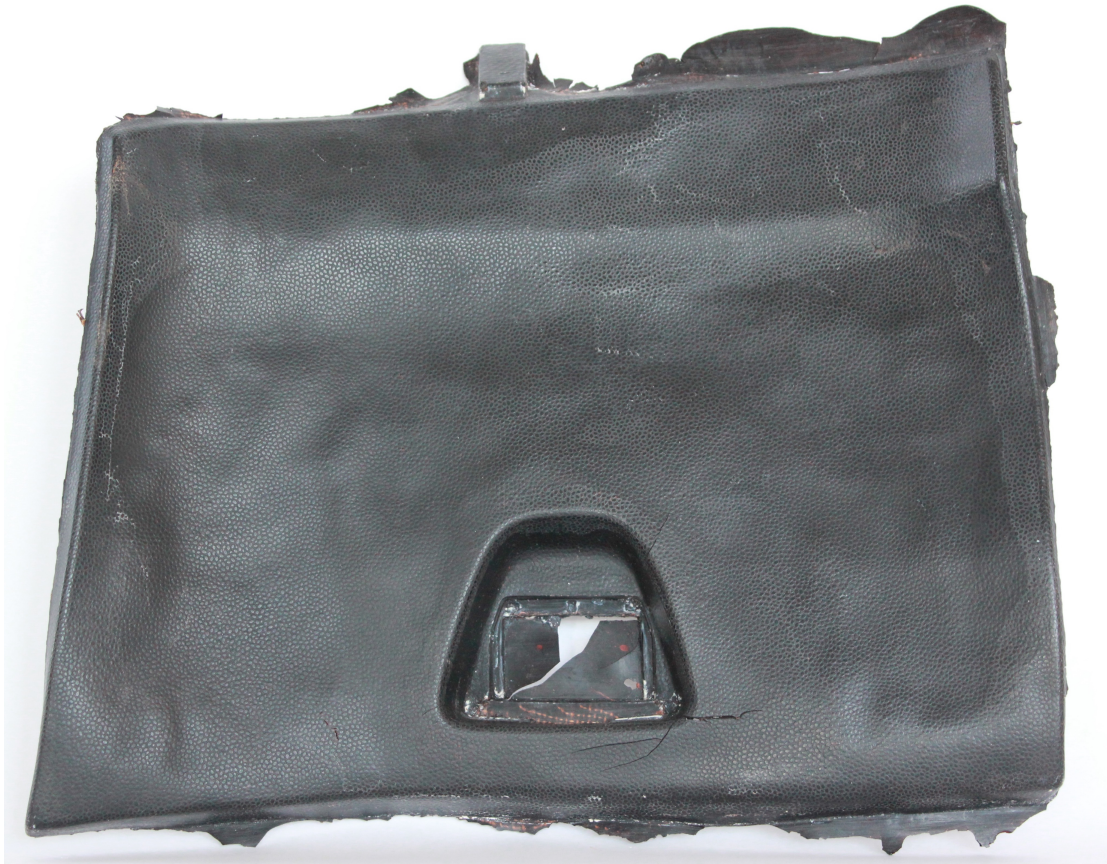
Figure 31: Glove-box lid made with bio-resin and woven jute coffee sack. Sheila Clark, 2014.
