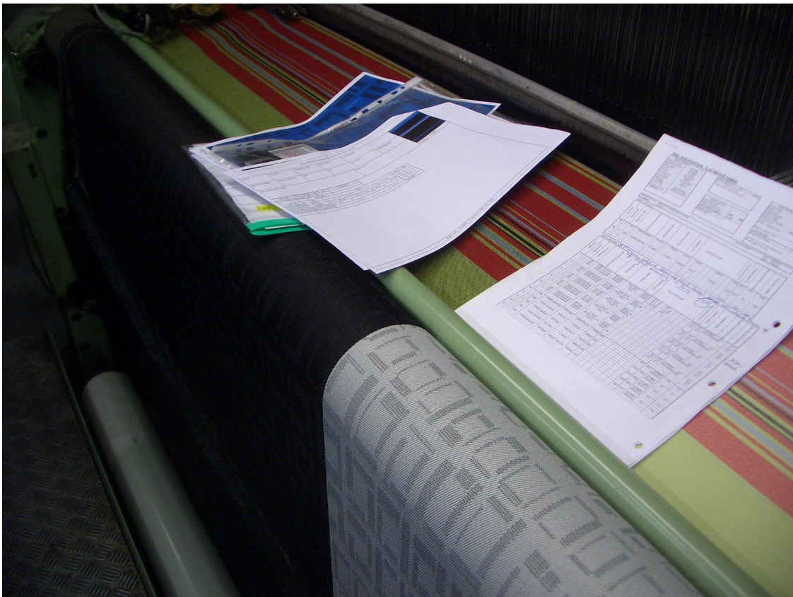
Figure 16: Stripe design being woven with the weft pick sequence pictured.
