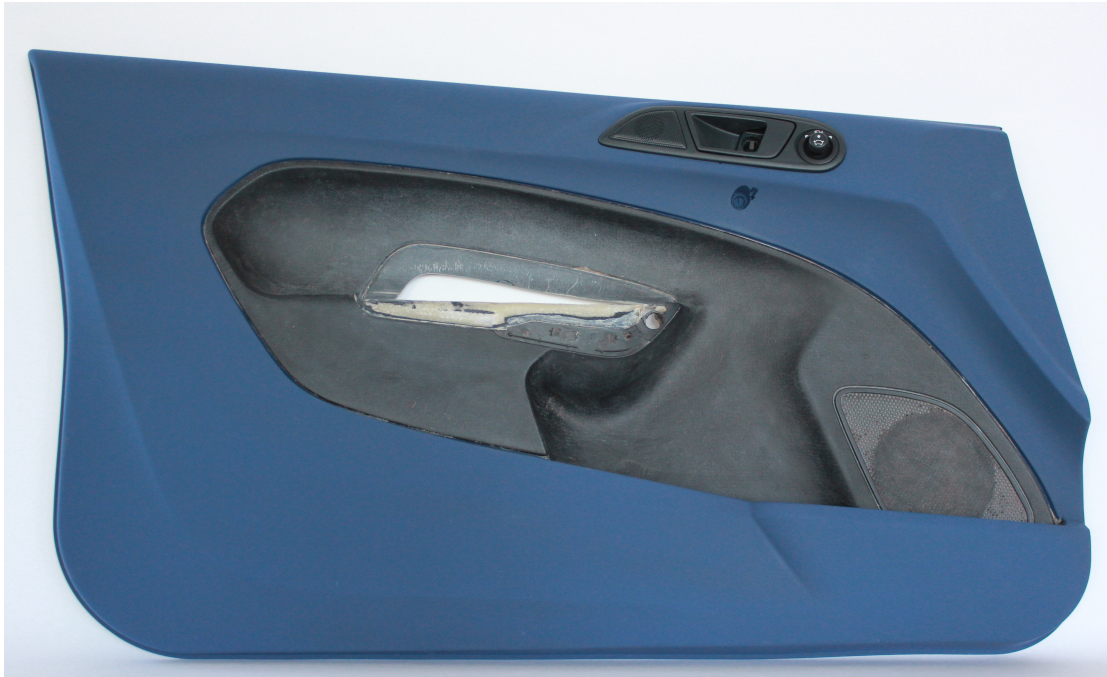
Figure 33: Painted outer door panel with Nextel paint and bio-resin inner door panel. Sheila Clark: 2015.
