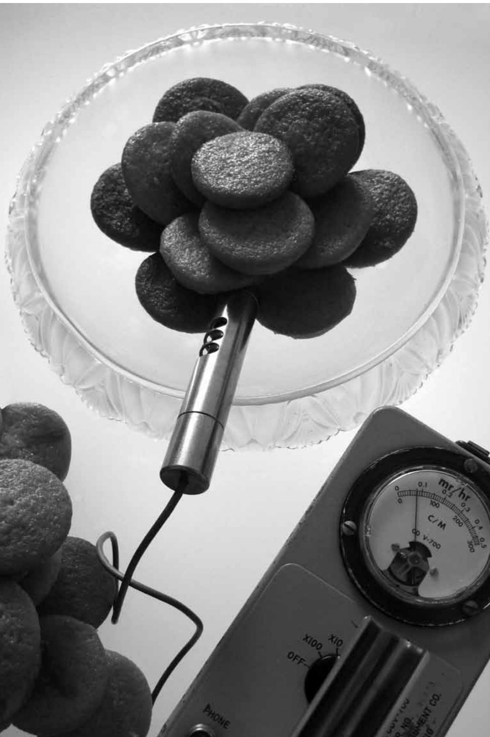
A Civil Defence V-700 Geiger counter measures radiation emitting from the 'yellowcake'.
