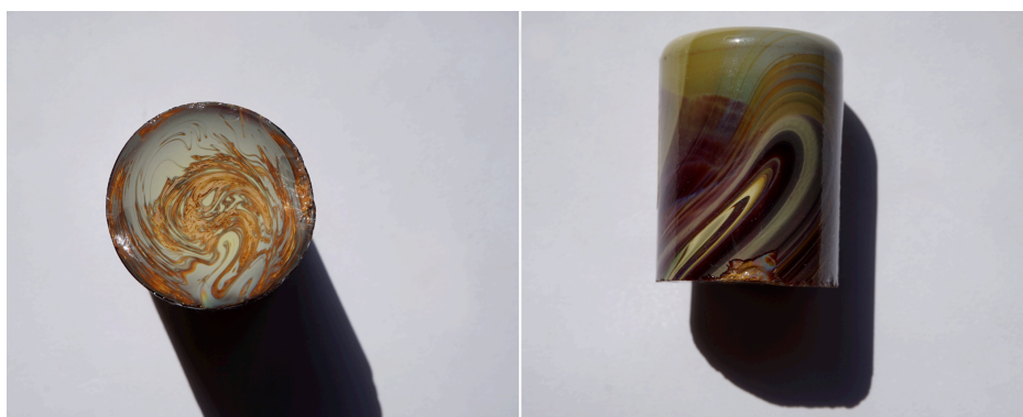
Figure 3: Sample of chalcedony glass G-109 manufactured by Gaffer shows relation between interior glass mass and its surface skin.
