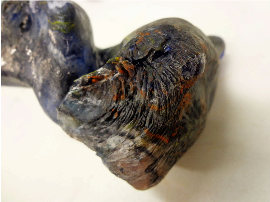
Figure 1: Glass sample with folded loops the result of coiling action.
