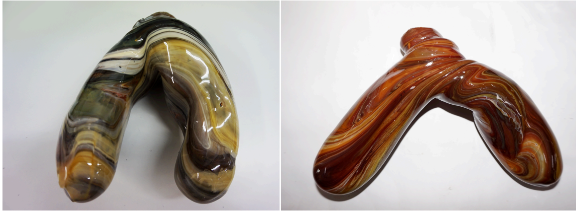
Figures 32 & 33: Unknown colour glasses (brought from Lviv, Ukraine) delivered in form of colour rods and melted together twice in glassblowing, proved incomparability - in both cases the surface had visible cracks. The maximal mass thickness is of approximately: 400 mm.
