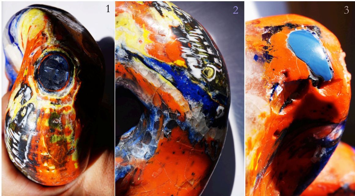
Figures 16 & 17 & 18: Aperture mark through which the inside structure can be seen - the concentric flow of the glass stream. Glass with the higher viscosity profile is accumulated closer to the surface (for instance, the lead-based glass that is `softer`) 2. Black specks of red powder colour were formed when in contact with the white one. 3. Inclusion of coloured glass pieces into the dimple shows an additional method of reconstituting a damaged glass surface during the surface treatment with UV adhesive.
