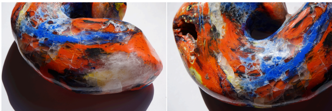
Figures 19 & 20: Sodium silicate of the Glasma glass forms a white crystal-like deposit visible at the surface.
