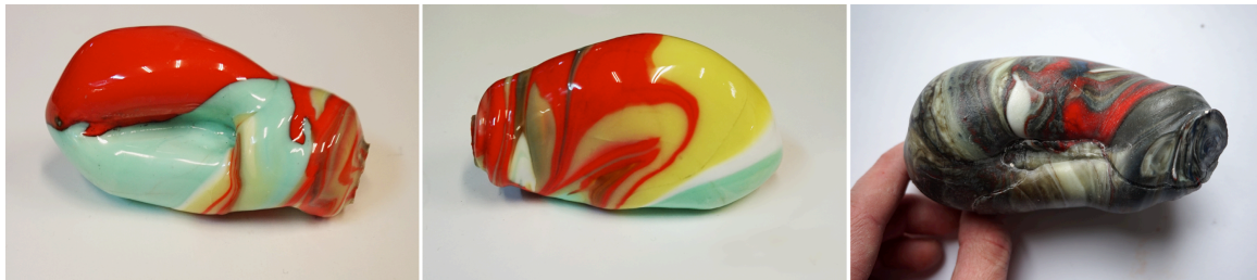
Figures 34 & 35 & 36: Sample of unknown glasses of four different colours (brought from Olomouc, Czech Republic) melted together. The colours were mixed in glassblowing once - the surface had visible cracks. After kiln firing the colours became dark grey but no visible cracks can be found (please refer to: firing cycle for kiln casting - March 2015 below).
