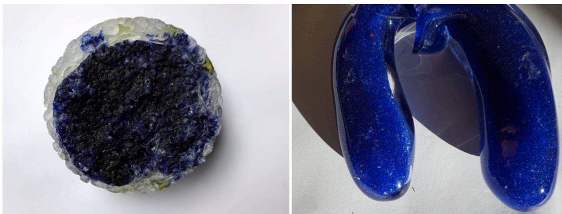
Figure 54: (from left:) Coloured glass samples - Glasma clear base with cobalt oxide 2 % and 0,2 %, Izabela Dziepak, March 2015, Royal College of Art
