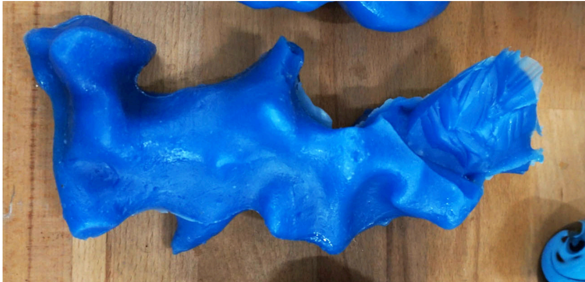
Figure 25: Wax model for lost wax casting before surface smoothing.
