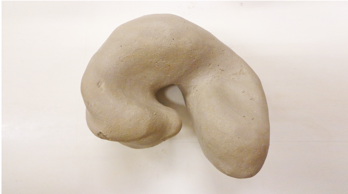
Figure 4: Clay model destined for making a double-sided casting mould.
