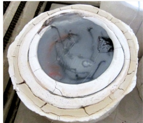
Figure 132 Hot casting Glasma glass and flameworked Gaffer cane into refractory mould, inside kiln, pre-heated to 600. Photo: Sheila Labatt
