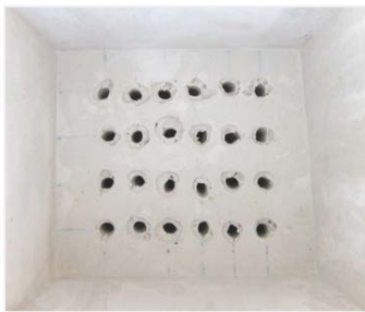
Figure 151 Deep, narrow holes in the bottom of a mould, created using the lost wax process, cause bubbles to rise when air is trapped by molten glass. Photo: Sheila Labatt
