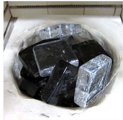
Figure 146 Custom clear and 'inky' billets [Figure 124] in conical refractory mould, ready for firing into a void at the bottom of the mould, held open by one horizontal billet. Photo: Sheila Labatt
