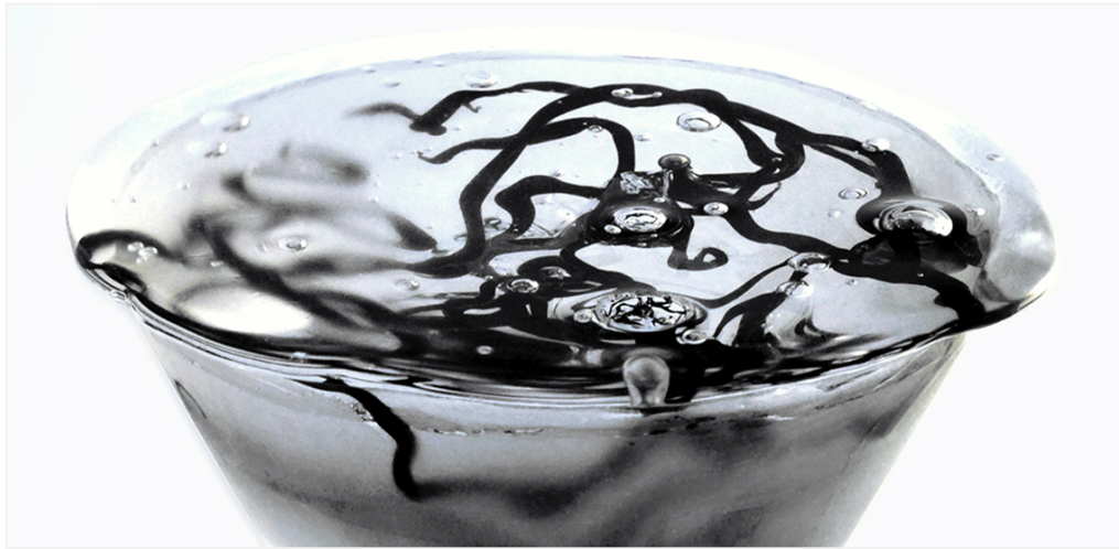
Figure 174 Surface bubbles to be ground out during coldworking. Photo: Sheila Labatt
