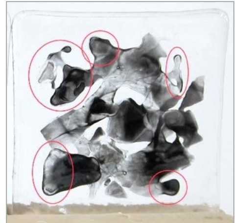
Figure 141 Fused eggshells on Tekta, red circles designate good liquid ink-like effects, 60x60x6mm. Photo: Sheila Labatt
