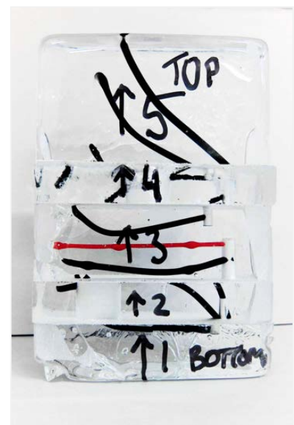
Figure 193 Arrangement of drilled segments back into a block for taping and re-firing. Photo: Sheila Labatt
