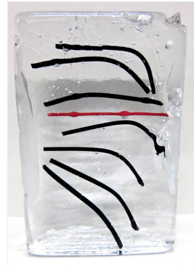
Figure 192 Block showing lengths of cane sandwiched between hot cast gathers. Photo: Sheila Labatt
