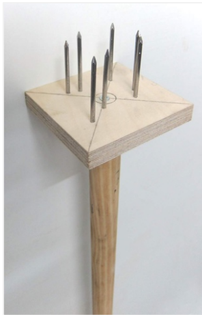
Figure 155 Wooden plunger with chilled nails quickly cools molten glass to create depressions that will become air pockets, then bubbles, when the next layer of molten glass covers them. Photo: Sheila Labatt.
