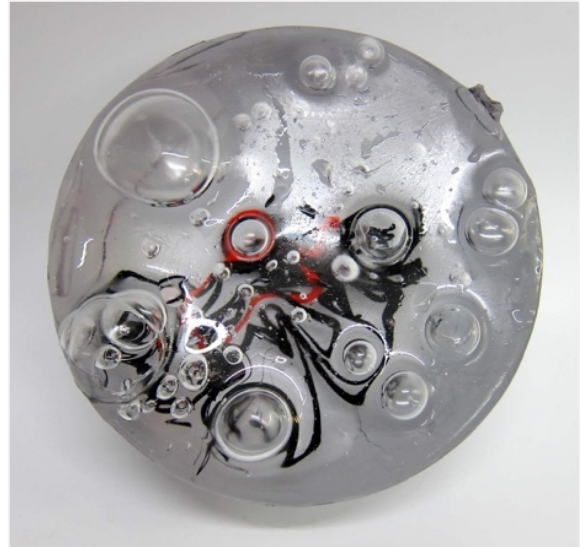
Figure 199 Bubbles showing on surface of hemisphere after hot casting and prior to grinding. Photo: Sheila Labatt
