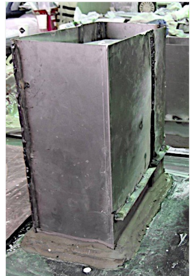
Figure 205 Welded, single-use, mild steel box used to support the mould and heavy molten lead crystal. Photo: Sheila Labatt
