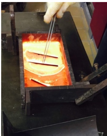
Figure 134 Adding and manipulating cane inclusions with tweezers. Photo: Sheila Labatt
