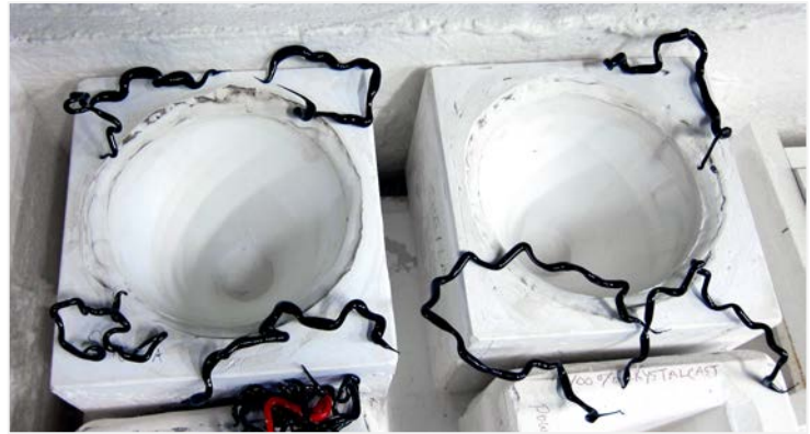
Figure 135 Frameworked inclusions, warming in a kiln, on the top surfaces of moulds, for quick inclusion into hot glass. Photo: Sheila Labatt
