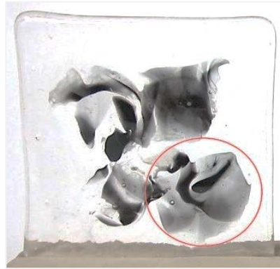
Figure 126 Good greyscale using Bullseye stringer and powder eggshells on Tekta, 60x60x6mm Photo: Sheila Labatt
