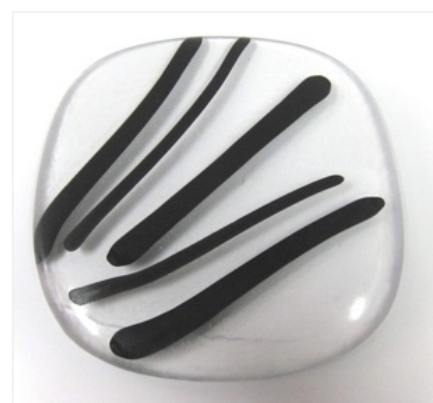
Figure 147 Clear, slumped Glastma billet with fused cane. Photo: Sheila Labatt
