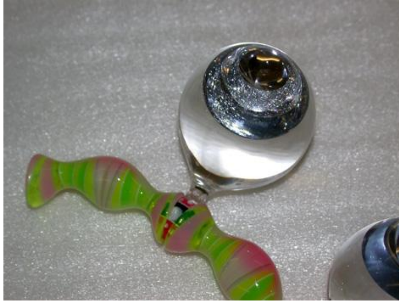
Fig 112. Spondylitis , detail of crazed PMMA
