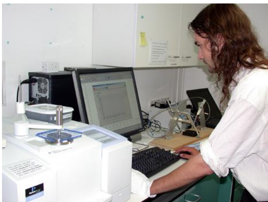
Fig 115. FTIR analysis of Grid Armpiece to confirm the material content
