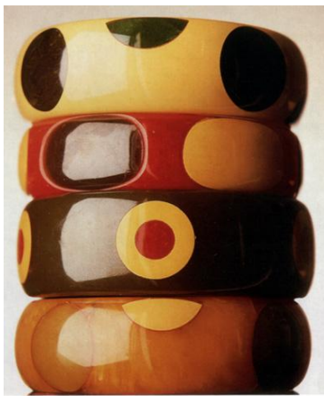
Fig 87. Phenol formaldehyde resin bangles, c. 1930s, showing a darkened surface
