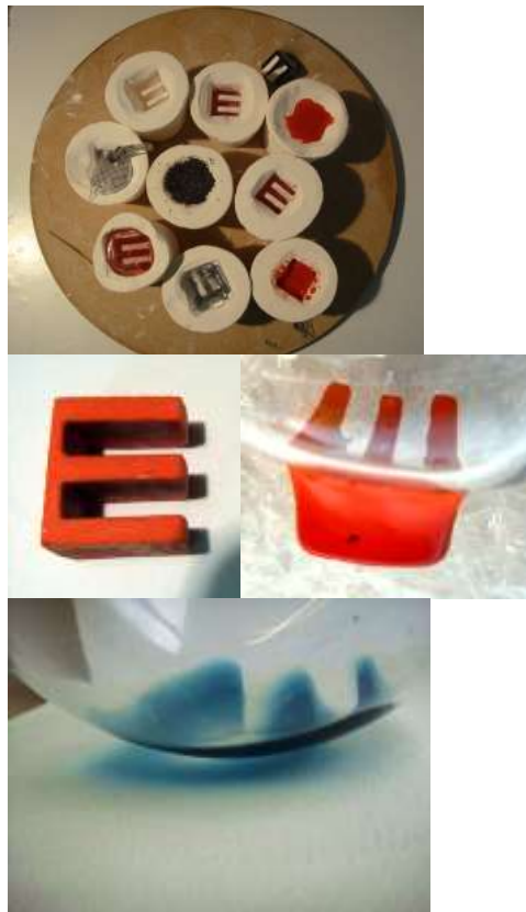
Figure 23: Casting process and result with block of red, and with 2mm slice of Kugler 'copper blue' cast rod
