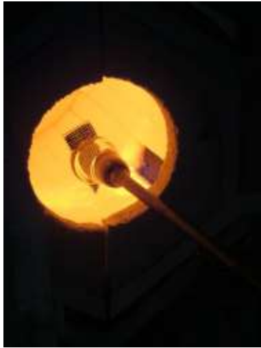
Figure 16: Glass panel entering glory hole
