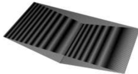
Figure 115: 'V' fold (12 degrees), under and overlays of the same frequency, fold parallel to the direction of the gratings
