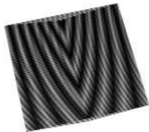
Figure 117: 'V' fold (12 degrees), under and overlays same frequency, fold perpendicular to the direction of the gratings
