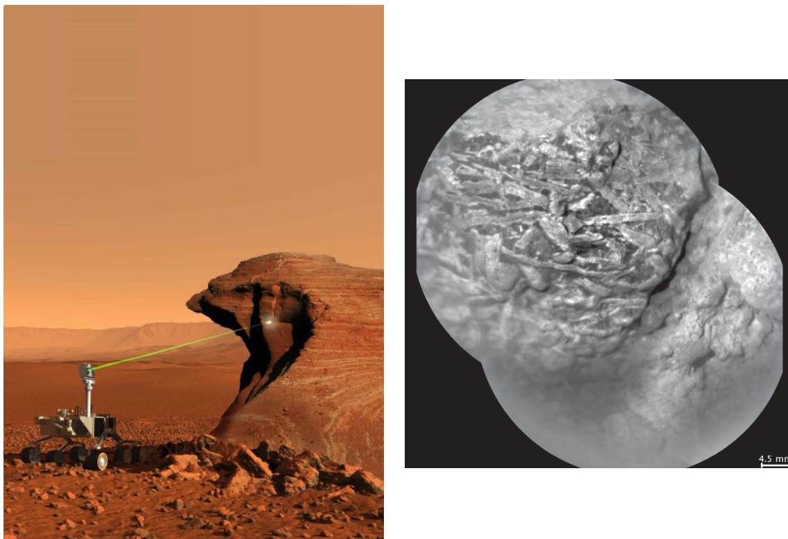
Figure 1.11. Laser-Induced Remote Sensing for the Chemistry and Micro-Imaging instrument will identify atomic elements in Martian rocks. Credit: NASA/JPL-Caltech/LANL/J.-L. Lacour, CEA.
