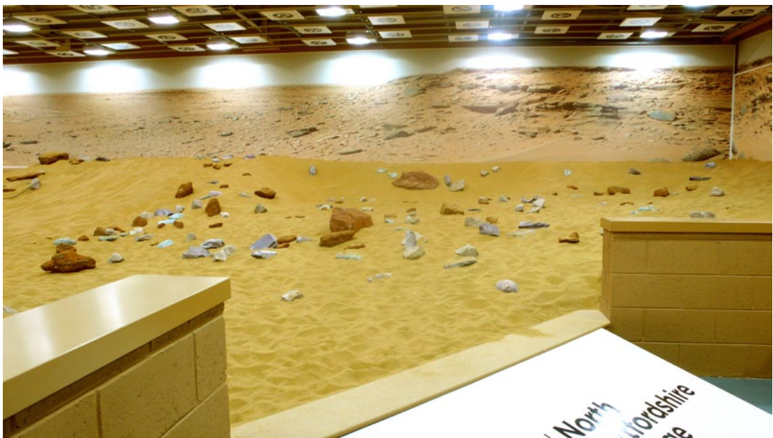
Figures 6.20 a-e. Photographs of the Mars Yard being used to test the European Space Agency's ExoMars rover's autonomous navigation system. Photographs taken on 27 August 2014 by author, courtesy of Airbus Defence and Space.
