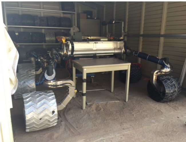
Figure 6.18. 'Scarecrow' rover, driving component of Curiosity used for testing in the Mars Yard. Photograph taken on 2 November 2015 by author, courtesy of JPL-Caltech.
