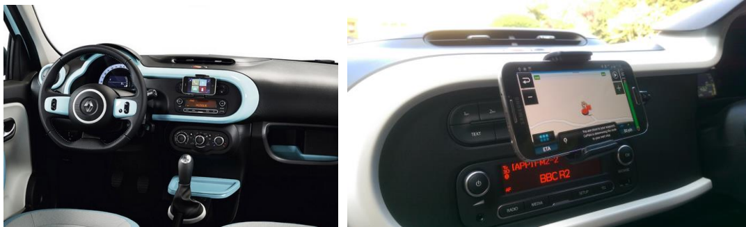
Figure 105: Renault Twingo's R&GO, enabling a driver to use their own smartphone
