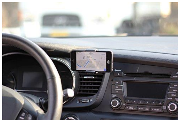
Figure 113: The smartphone is positioned on the central air vent by using a universal phone holder
