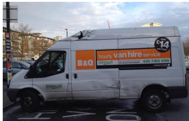
Figure 74: The damaged roof of car club van
