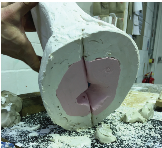
Figure E.100: Final silicone mold, showing the inlet for the liquid wax.
