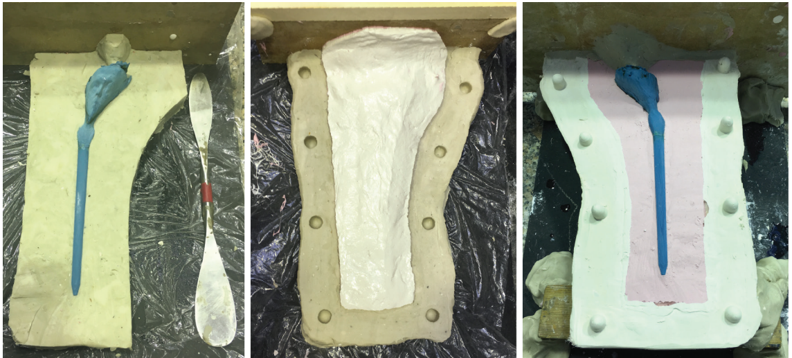
Figure E.99: Silicone mold making steps, creating two halves.
