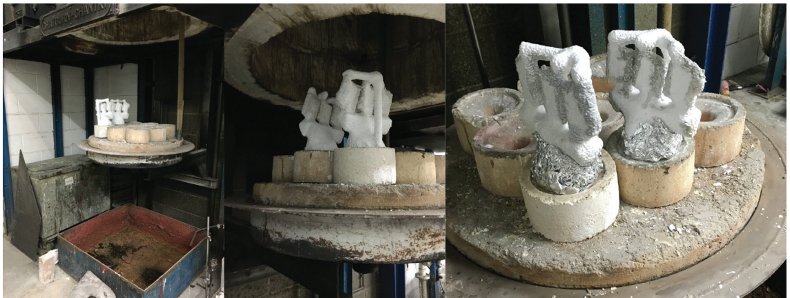
Figure E.50: (left/middle) Melting out the wax. (right) Preheating before the bronze pour.
