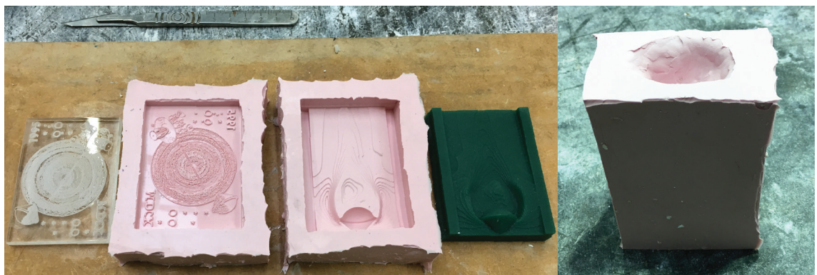
Figure E.48: (left) Front and back BAMS master models and silicone molds. Obverse side CNC machined out of chemiwood. Reverse side laser engraved into acrylic. (right) Silicone mold from the final master model, made out of a single chemiwood piece. Obverse side CNC'd, reverse side laser engraved.
