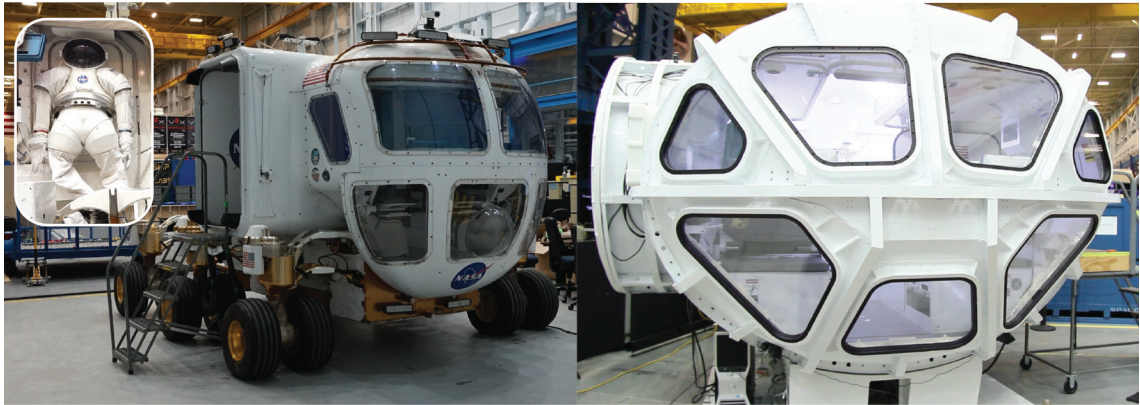
Figure 6.6: (left) First generation SEV with suitport. (right) Second generation SEV at NASA JSC.
