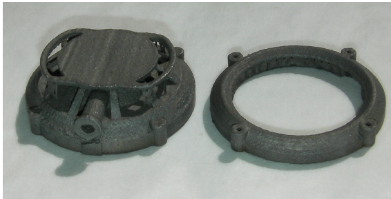
Figure E.81: SLM printed titanium parts. This sample 3D print did not provide the needed accuracy.
