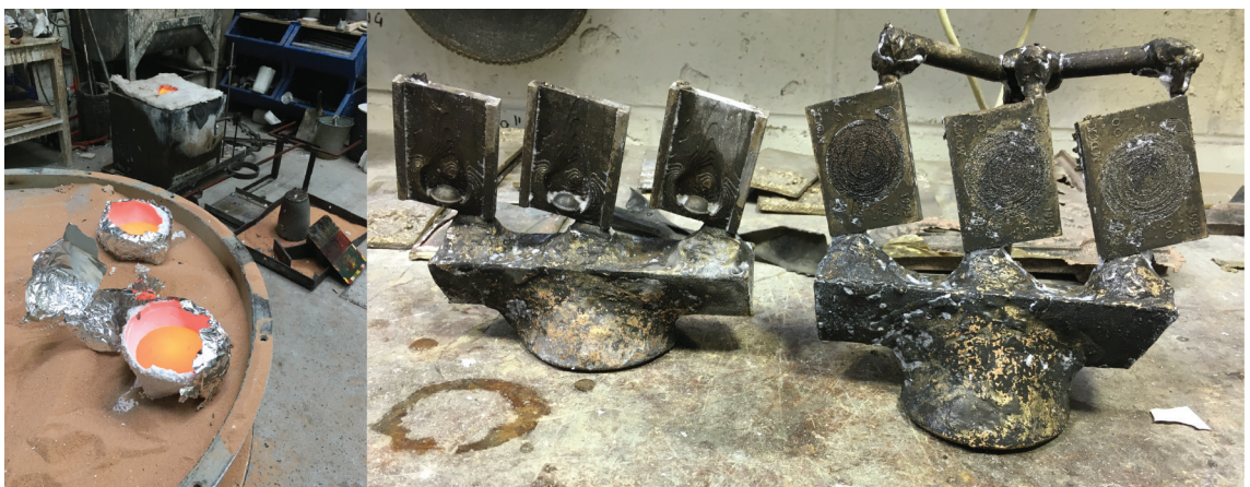
Figure E.51: (left) After the pour. (right) The six medals with runners and risers.
