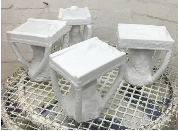
Figure E.25: Building up 8 layers of ceramic coating, layer by layer, allowing sufficient time to dry (at least 4-5 days total).
