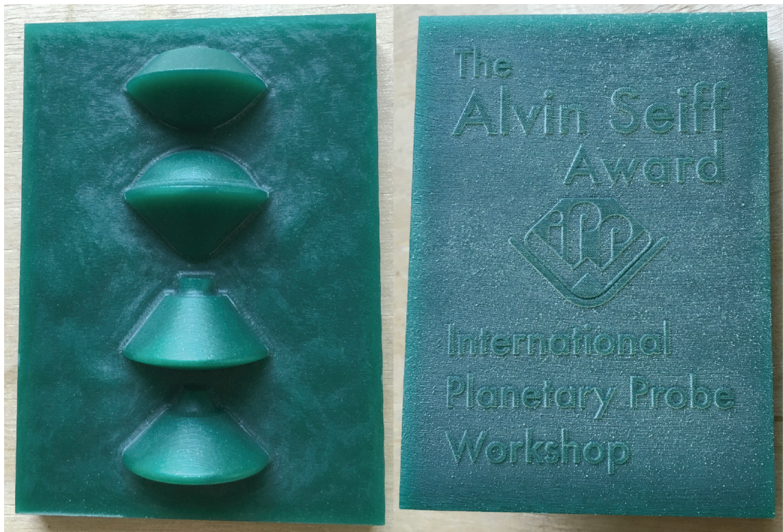
Figure E.58: IPPW medal master model. (left) Obverse side CNC machined at RCA's Digital Aided Making (DAM) workshop. (right) Reverse side, laser etched at RCA DAM.
