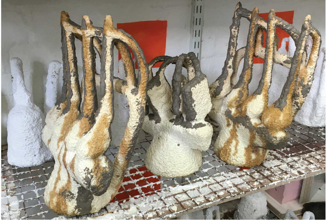
Figure E.101: Ceramic shells with cement fixes of cracks after melting out the wax.
