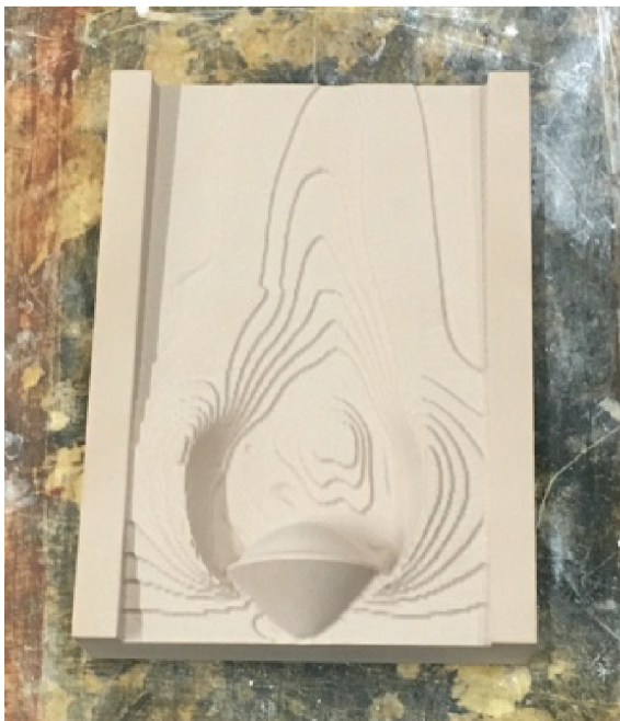
Figure E.17: CNC machined chemiwood version used as the master model for the bronze sculpture project.
