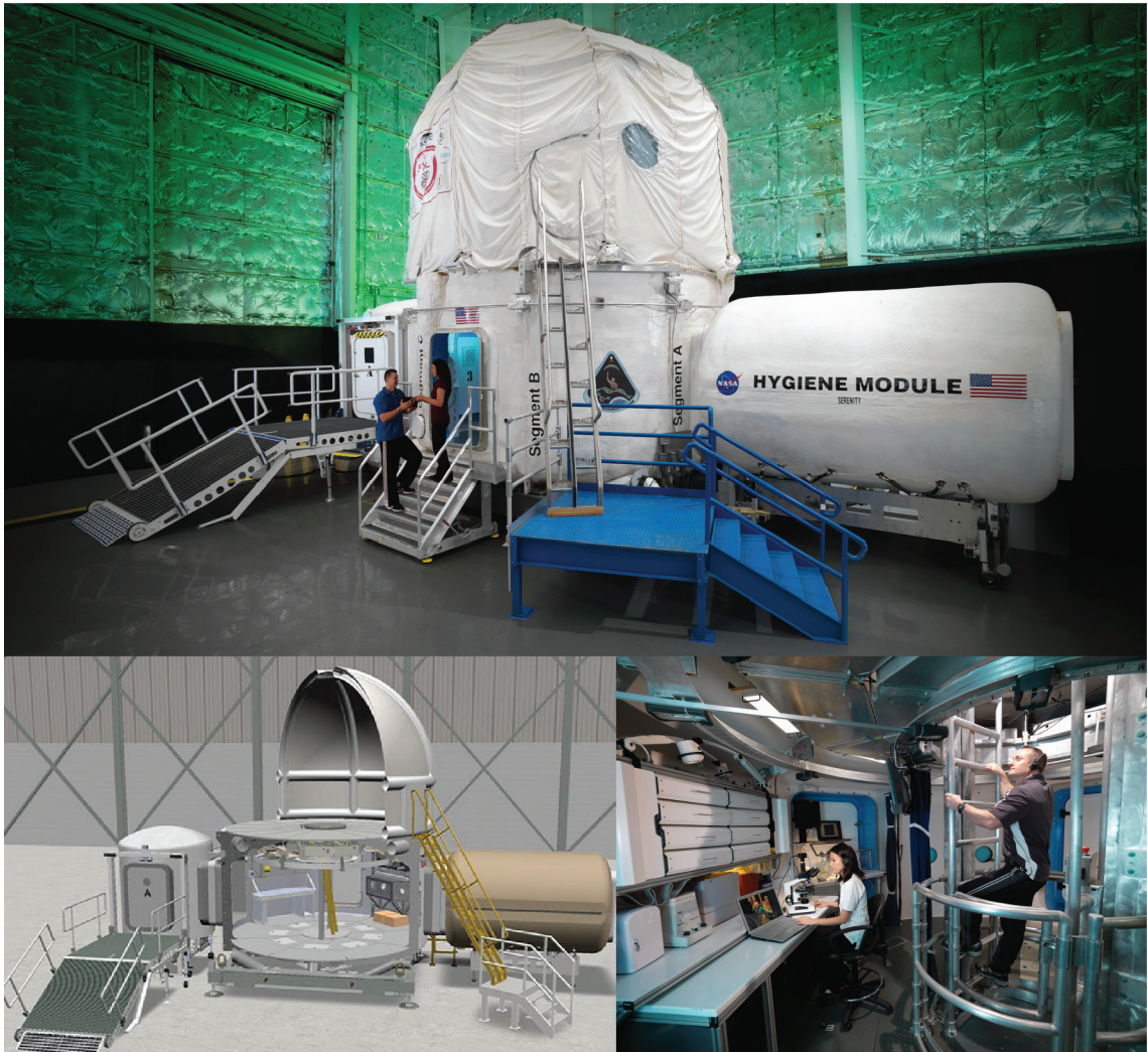
Figure 6.5: HERA/HDU analog module. Clockwise: External view, inside view, and CAD model.
