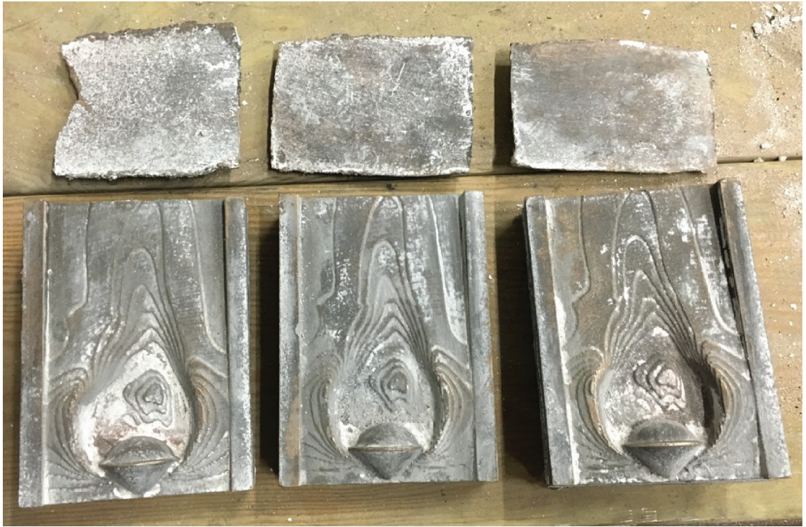
Figure E.35: Ceramic fragments, runners and risers removed (front sides & back plates).
