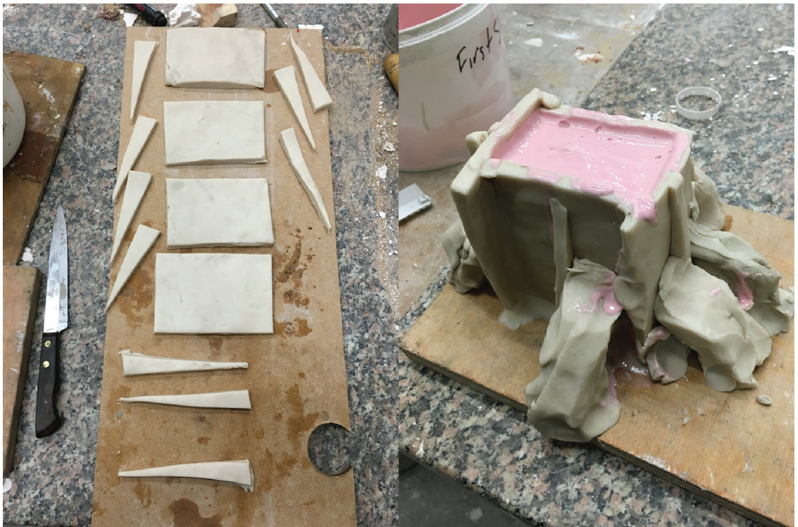
Figure E.60: Creating the silicone mold. (left) Creating the walls. (right) Pouring the silicone around the model.
