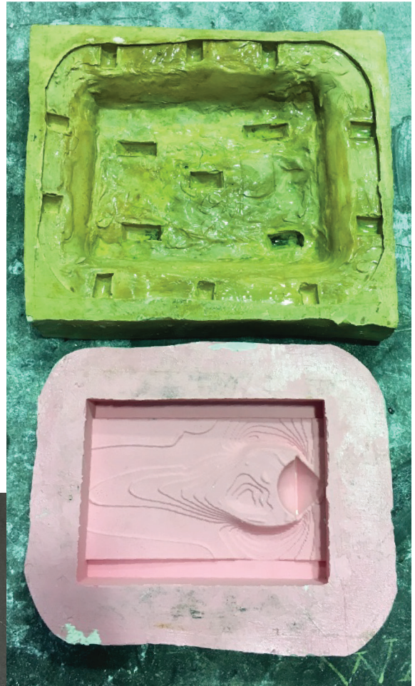
Figure E.22: Plaster shell showing the locations where the silicone mold keys fit.
