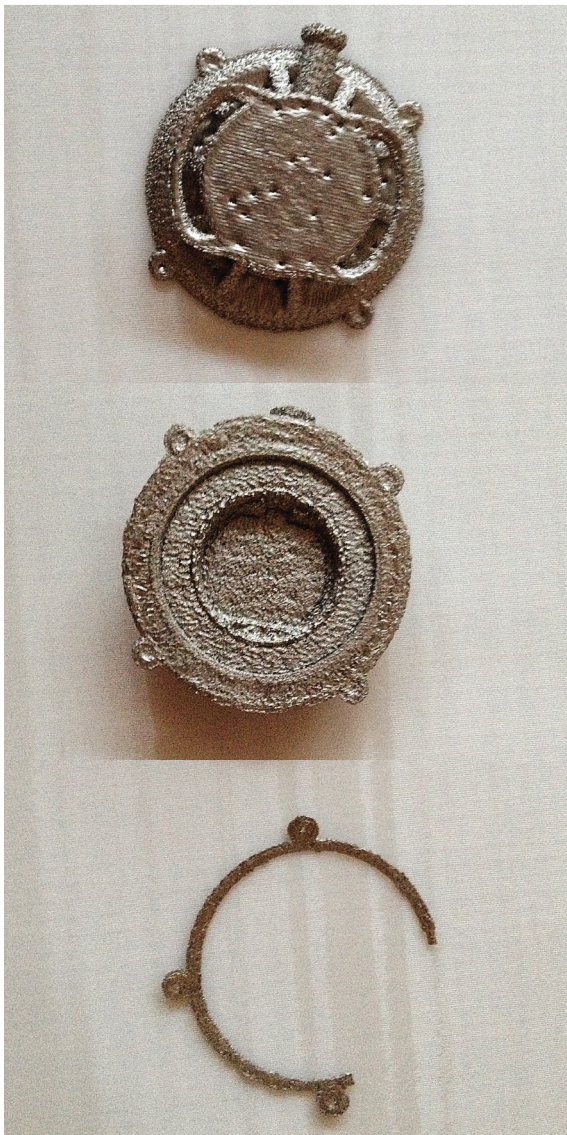
Figure E.79: 3D printed titanium parts (top and bottom housing / upside and down views). This EBM printing method did not produce the desired parts with the right accuracy.
