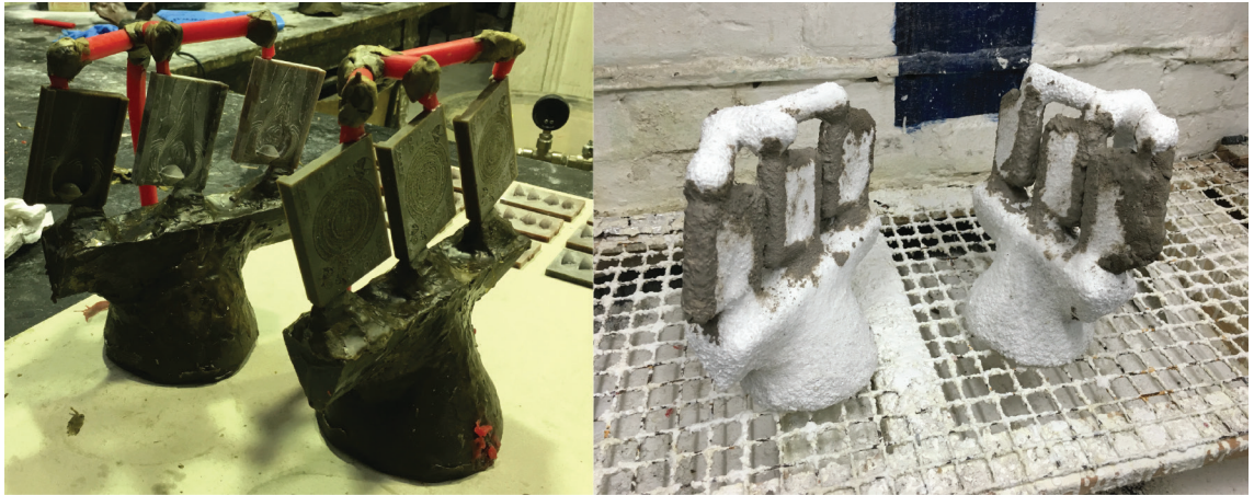
Figure E.49: (left) Building up a tree with runners and risers. (right) Building up the ceramic shell layers.
