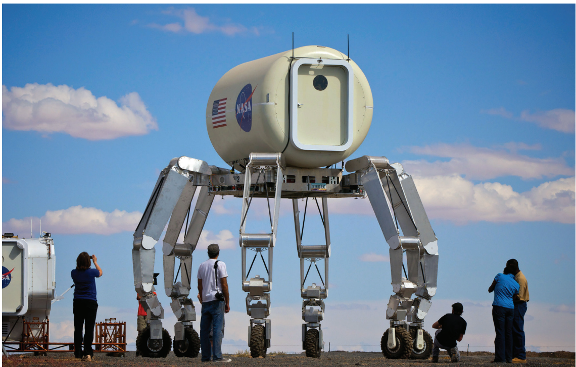
Figure 6.7: Half-scale ATHLETE rover, carrying a habitat mockup.
