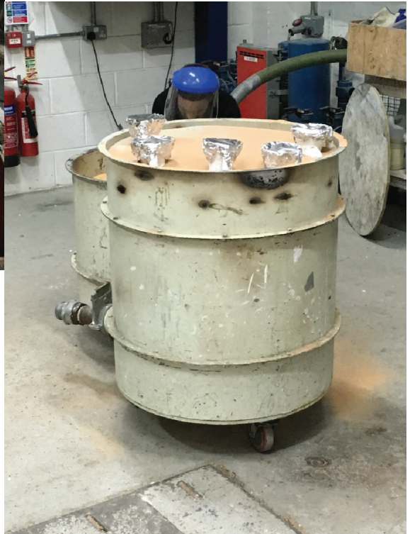
Figure E.30: Shells placed in sand for support during the pour.
