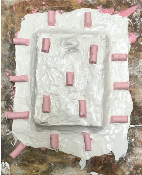
Figure E.19: Second layer of the silicone mold, with keys to fit into the plaster shell.
