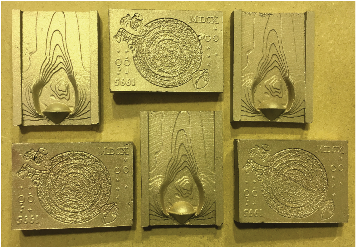
Figure E.53: The six medals after the chasing steps, including grinding and sand blasting.
