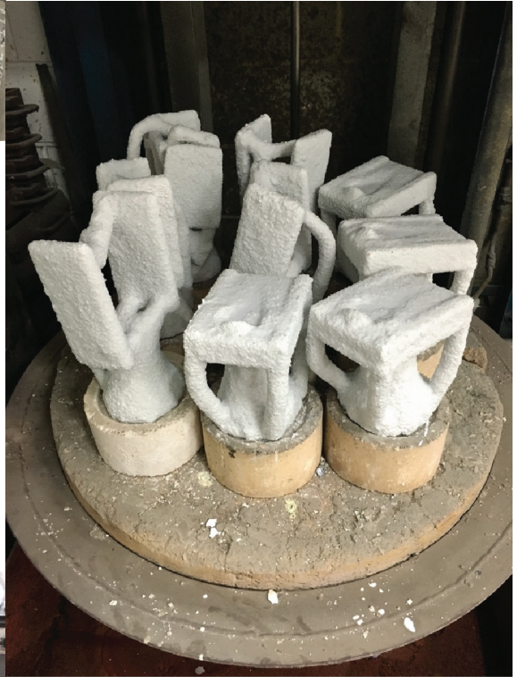
Figure E.26: Melting out the wax from the ceramic shells. (Note, the backs of the models are cut out, and will be poured separately from the front sides.
