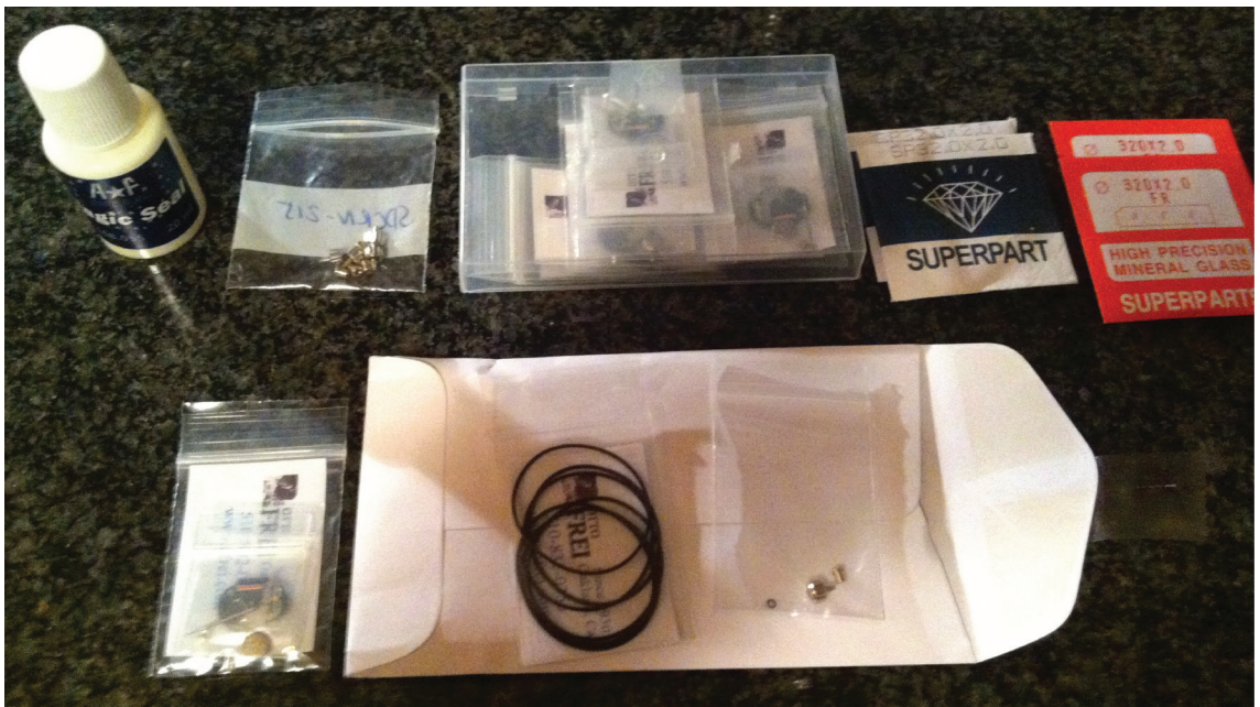
Figure E.74: Commercial off the shelf (COTS) parts; top row, from left: magic seal; screw-in crown; digital movements; artificial sapphire crystals; high precision mineral glass. Bottom row from left: more digital movements; O-rings; extra screw-in crowns for water tightness.
