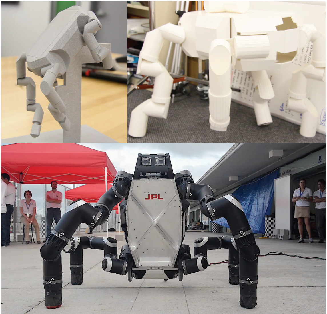
Figure 7.19: From 3D printed model, through mockup, to final build; RoboSimian, JPL's entry to the DARPA robotic challenge in 2014.
