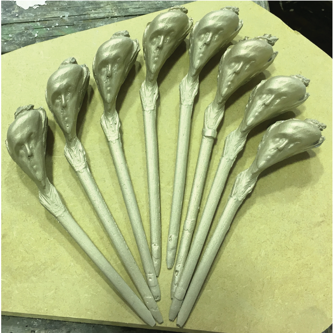
Figure E.103: The 8 letter openers after sand blasting, but prior to patination.
