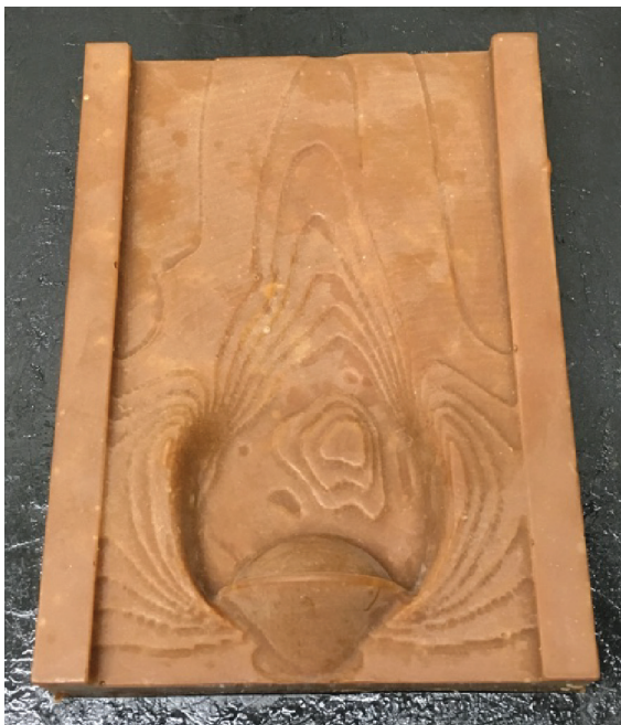
Figure E.23: Hollow wax model created using the silicone mold.
