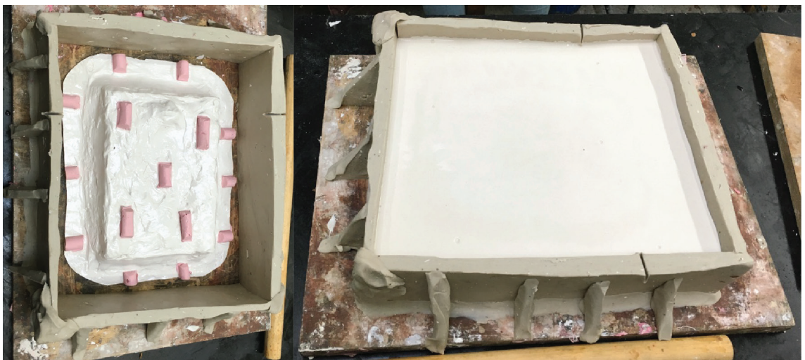
Figure E.21: Making the plaster shell around the silicone mold.
