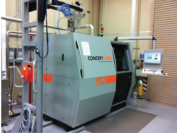
Figure E.80 M2 Cusing SLM machine, built by Concept Laser, a division of Hoffman Innovation Group of Lichtenfels, Germany.
