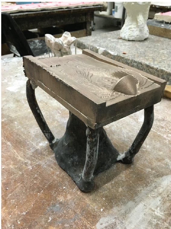
Figure E.34: Ceramic shell fragments removed, artifact sand blasted. Runners and risers still attached.
