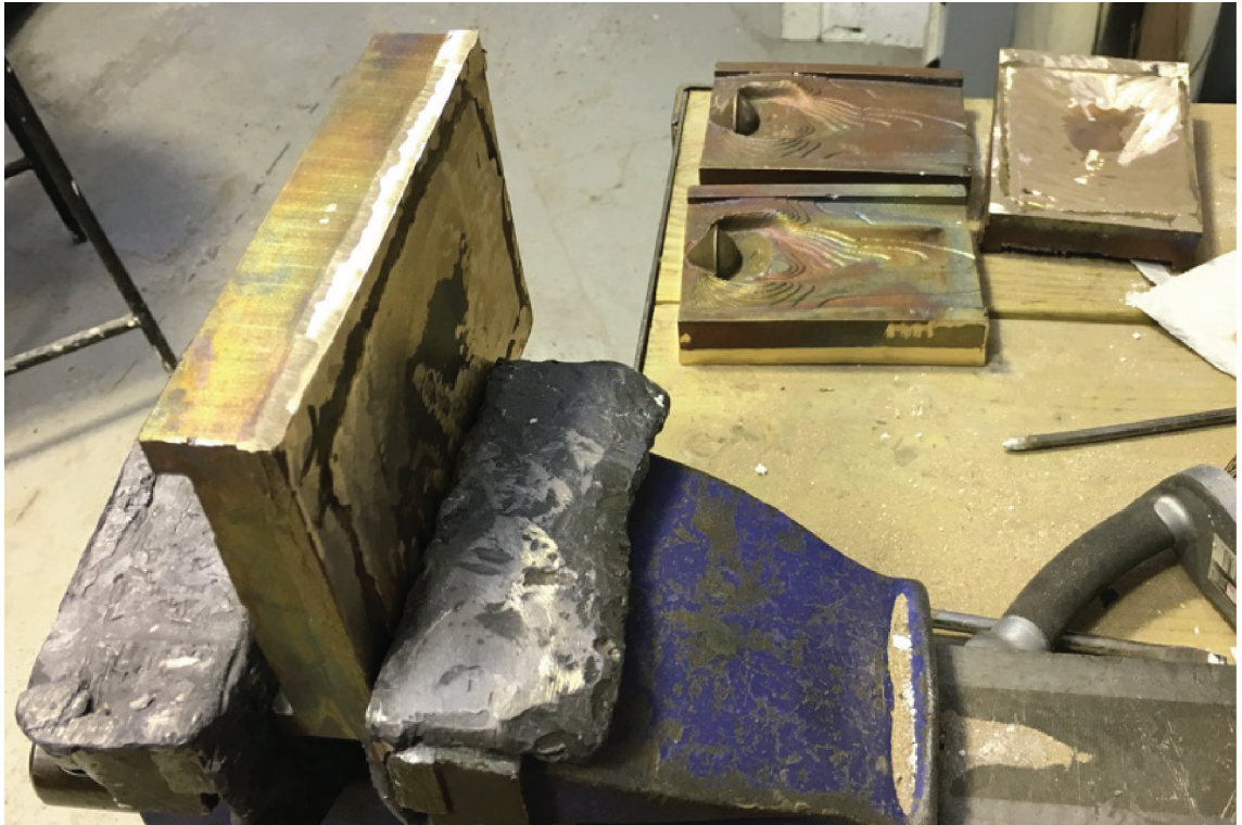
Figure E.38: Next chasing step: grinding the edges and weld marks.
