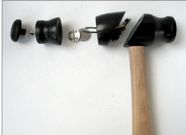
Figure 47 , Exploded view of nylon hammer with electronic components Image by © Kathryn Hinton, 2009
