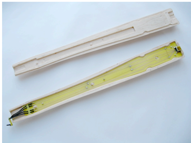
Figure 59 , Milled maple handle with PCB development board Image by © Kathryn Hinton, 2010
