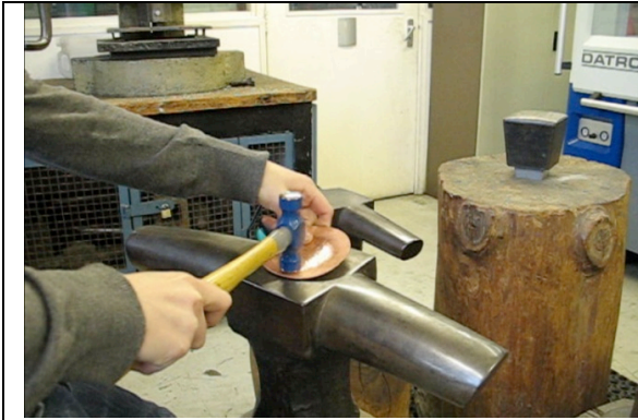
Figure 33 , Traditional hammering in the silversmithing workshop at the Royal College of Art Image by © Kathryn Hinton, silversmithing workshop in department of Goldsmithing, Silversmithing, Metalwork and Jewellery, 2009, Royal College of Art
