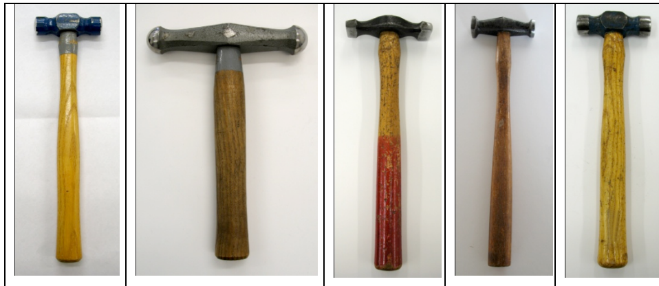
Figure 24 , Peening, blocking, raising and light and heavy planishing hammers Image by © Kathryn Hinton 2009, Royal College of Art
