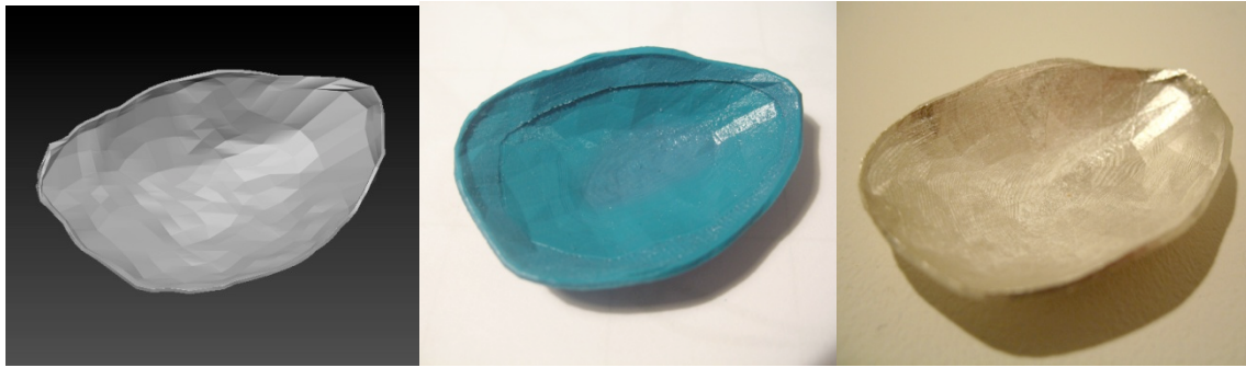
Figure 106 , Digital ZBrush® mesh, Solidscape wax, cast sterling silver Image by © Kathryn Hinton, 2010
