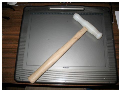
Figure 20 , Trust 1200V tablet board with digital pen housed in nylon hammer head Image by © Kathryn Hinton, 2008
