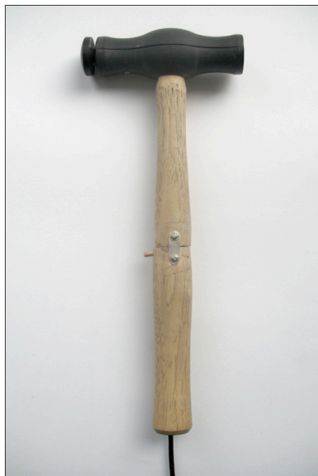
Figure 23 , Rapid prototyped black hammer head with wooden handle Image by © Kathryn Hinton, 2008
