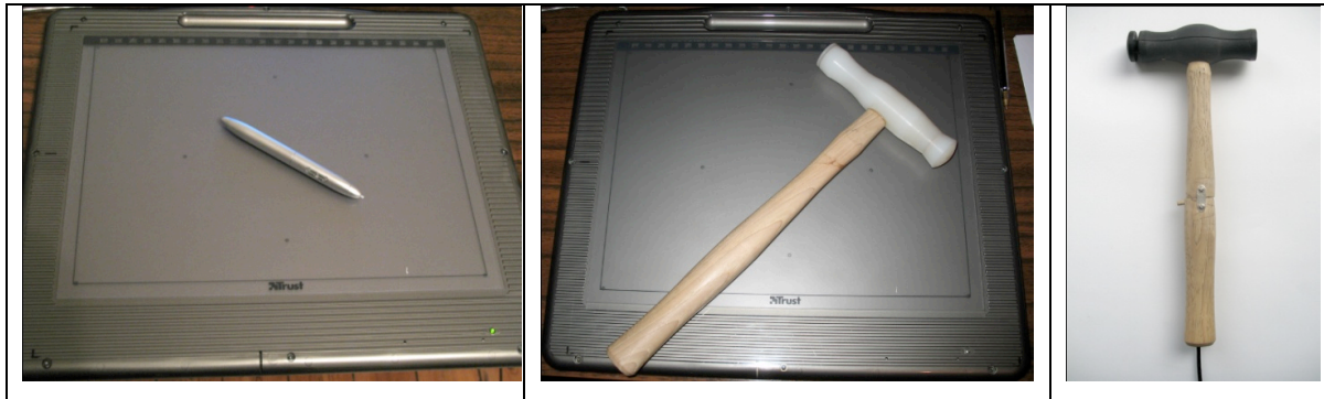
Figure 25 , Interface devices; Trust digital tablet and pen, Trust digital tablet and pen housed in nylon hammer-head, rapid prototyped hammer-head with tilt sensor. Image by © Kathryn Hinton, 2009
