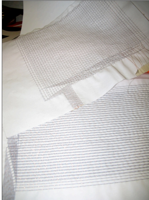
Figure 85 , Copper wire was sewn through fabric Image by © Kathryn Hinton, 2008
