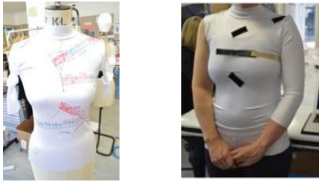
Figure 5: Dielectric electroactive polymer (DEAP) thoracic sensors project developed by A.Toomey, N.O'Connor and P. Stevenson-Keating in 2012. The thoracic muscles and anchor points were mapped onto the vest toile and used as the blueprint for the integration of the bespoke sensors.
