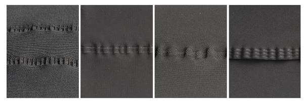
Figure 3.8 (Left, Centre Left and Centre Right) Examples of ultrasonic seams joined in a lap configuration using continuous ultrasonic welding equipment (Paine 2013)
