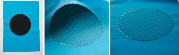
Figure 6.10 Fabric samples with zones of compression created using absorptive lower panels and TLW equipment (Paine 2014)
