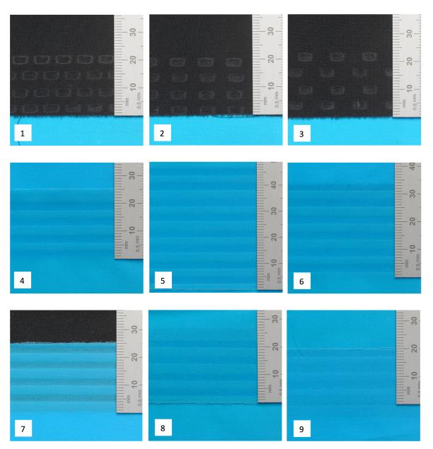
Figure 3.24 9 patterned laser welded seams included in the investigation (Paine 2014)
