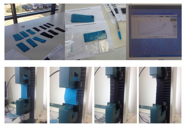
Figure 5.16 Mechanical testing of all-over surface effects at Speedo (Paine 2014)
