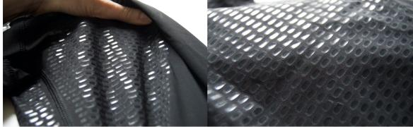
Figure 6.13 Swimsuit prototype with targeted laser-melted panels (Paine 2014)
