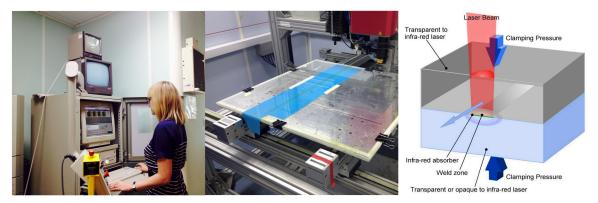
Figure 1.2 (Left) Researcher operating laser welding equipment from outside lab at TWI (TWI 2012) Figure 1.3 (Centre) Sample set up on x-y table for laser welding at TWI (Paine 2013) Figure 1.4 (Right) Material configuration for transmission laser welding (Image courtesy of TWI)
