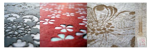
Figure 4.5 Selection of laser-treated non-woven fabrics by Faith Kane(Kane 2009)
