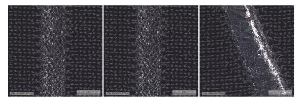
Figure 5.1 (Left) Fabric sample showing laser surface melting created using a power setting of 40W (Paine 2014) Figure 5.2 (Centre) Fabric sample showing laser surface melting created using a power setting of 50W (Paine 2014) Figure 5.3 (Right) Fabric sample showing laser surface melting created using a power setting of 60W (Paine 2014)
