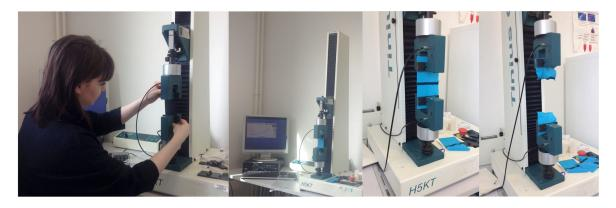
Figure 3.23 Mechanical testing of seams at Speedo (Paine 2014)
