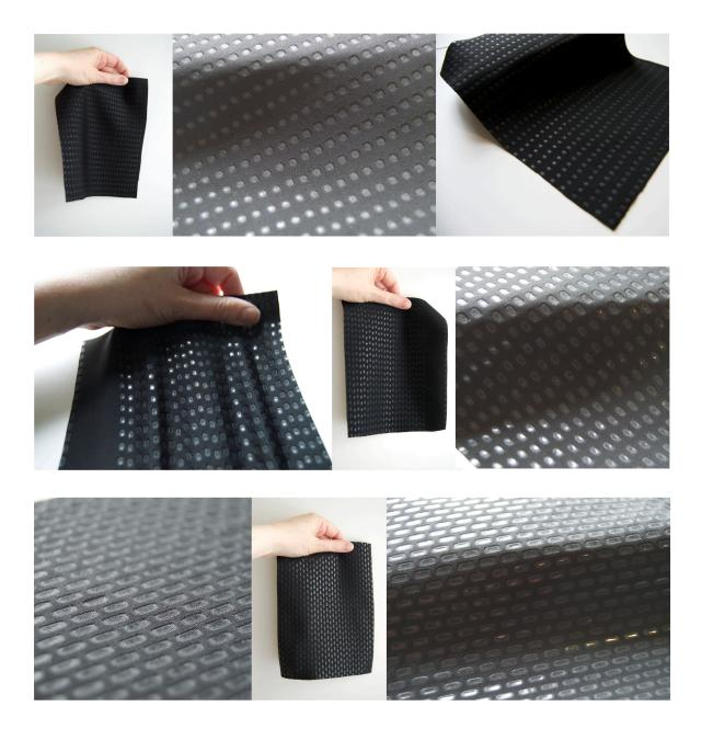
Figure 5.13 (Top) Fabric sample with laser melted spots, Tpuls 30 ms, Trep 100ms (Paine 2014) Figure 5.14 (Middle) Fabric sample with laser melted spots, Tpuls 50 ms, Trep 100ms (Paine 2014) Figure 5.15 (Bottom) Fabric sample with laser melted spots, Tpuls 70 ms, Trep 100ms (Paine 2014)
