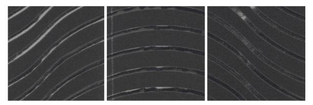
Figure 6.1 (Left) Fabric sample showing left side of curved laser melted pattern (Paine 2014) Figure 6.2 (Centre) Fabric sample showing middle section of curved laser melted pattern (Paine 2014) Figure 6.3 (Right) Fabric sample showing right side of curved laser melted pattern (Paine 2014)
