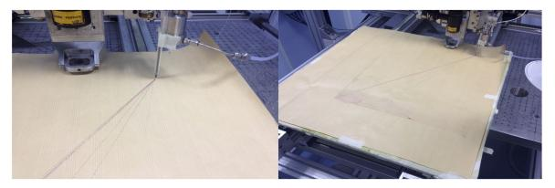
Figure 3.13 Pen attachment to TLW equipment at TWI used to assist in translating the code that moves the x-y table beneath the laser head (Paine 2013)
