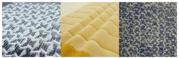
Figure 1.5 Examples of 'Laser-Finished' textile samples from Kate Goldsworthy's PhD research (Images courtesy of Kate Goldsworthy)
