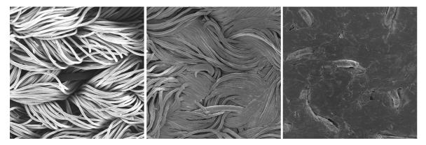
Figure 3.1 (Left) SEM image of an unwelded sample of stretchy jersey fabric (TWI 2012) Figure 3.2 (Centre) SEM image of a sample of stretchy jersey fabric welded at high speed (TWI 2012) Figure 3.3 (Right) SEM image of a sample of stretchy jersey fabric welded at slow speed (TWI 2012)
