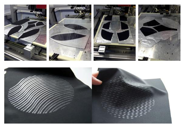
Figure 6.8 (Top) Method of creating targeted zones of compression using reflective stencils and TLW equipment (Paine 2014)
