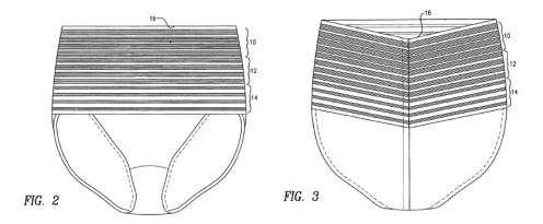
Figure 4.16 Example of application for elastic fabric with varied zones of compression (Shannon 2007, pp.2-3)
