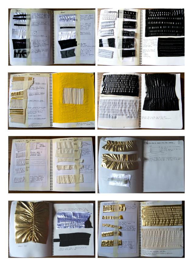
Figure 3.7 Sketchbook pages from practice-led investigation using ultrasonic welding equipment (Paine 2013)
