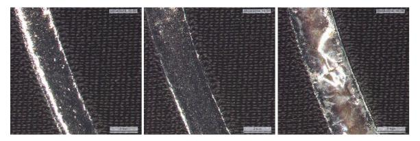
Figure 5.4 (Left) Fabric sample showing laser surface melting created using a speed setting of 3m/min (Paine 2014) Figure 5.5 (Centre) Fabric sample showing laser surface melting created using a speed setting of 2m/min (Paine 2014) Figure 5.6 (Right) Fabric sample showing laser surface melting created using a speed setting of 1m/min (Paine 2014)
