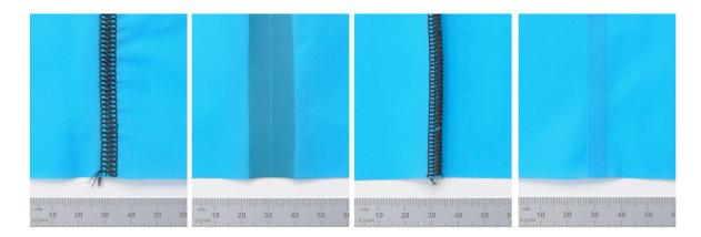
Figure 3.19 (Left) Flat-locked seam (Paine 2014) Figure 3.20 (Centre left) Adhesive taped seam (Paine 2014) Figure 3.21 (Centre right) Over-locked seam (Paine 2014) Figure 3.22 (Right) Adhesive lap seam (Paine 2014)
