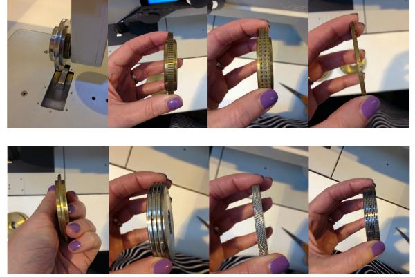
Figure 3.10 Patterned anvils from continuous ultrasonic welding machine used for seaming investigation (Paine 2013)
