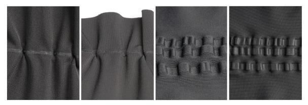
Figure 3.16 (Centre Right, Right,) Fabric samples demonstrating ruched effect created using polyurethane tape and laser welding equipment (Paine 2013) Figure 3.17 (Left, Centre Left) Fabric samples demonstrating all-over surface rippling effect created using laser welding equipment (Paine 2013)
