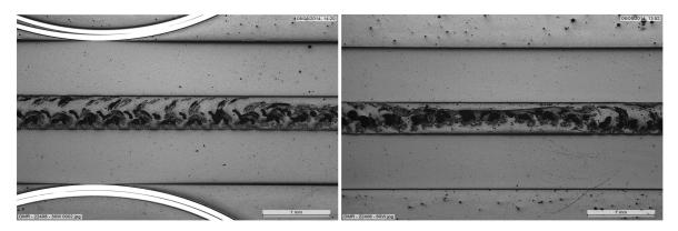
Figure 6.5 (Left) Cross section of fabric sample with surface melting created using a laser power of 30W (TWI 2014) Figure 6.6 (Right) Cross section of fabric sample with surface melting created using a laser power of 60W (TWI 2014)
