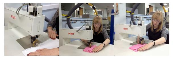
Figure 1.1 Pfaff continuous ultrasonic welding equipment at TWI (TWI 2012)
