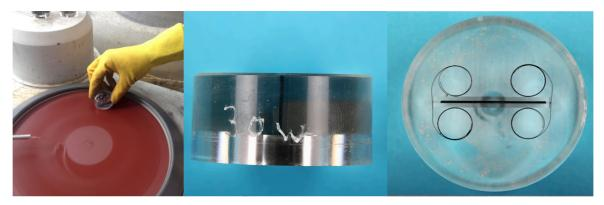
Figure 6.4 Process of mounting and polishing sample for microscopic analysis (Paine 2014)
