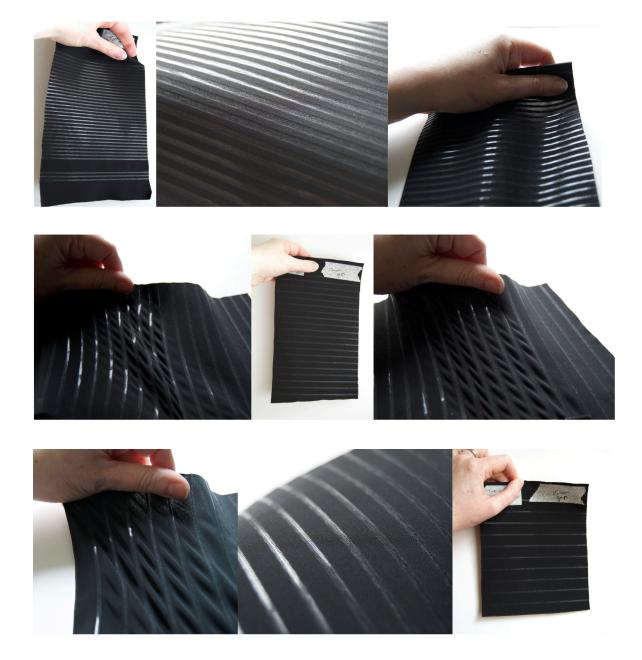
Figure 5.10 (Top) Fabric sample with laser melted lines, 5mm apart (Paine 2014) Figure 5.11 (Middle) Fabric sample with laser melted lines, 10mm apart (Paine 2014) Figure 5.12 (Bottom) Fabric sample with laser melted lines, 15mm apart (Paine 2014)
