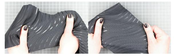
Figure 3.15 Sample demonstrating the effect of laser surface melting across the full width of a fabric sample (Paine 2013)
