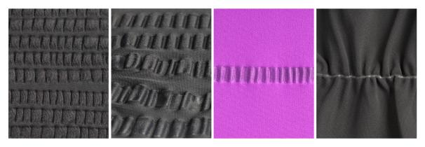
Figure 3.11 (Left, Centre Left, Centre Right) Fabric samples demonstrating all-over rippled surface effect created using ultrasonic welding equipment (Paine 2013)
