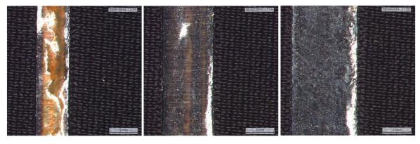
Figure 5.7 (Left) Fabric sample showing laser surface melting created with a laser height of 55mm between x-y table and laser head (Paine 2014)
