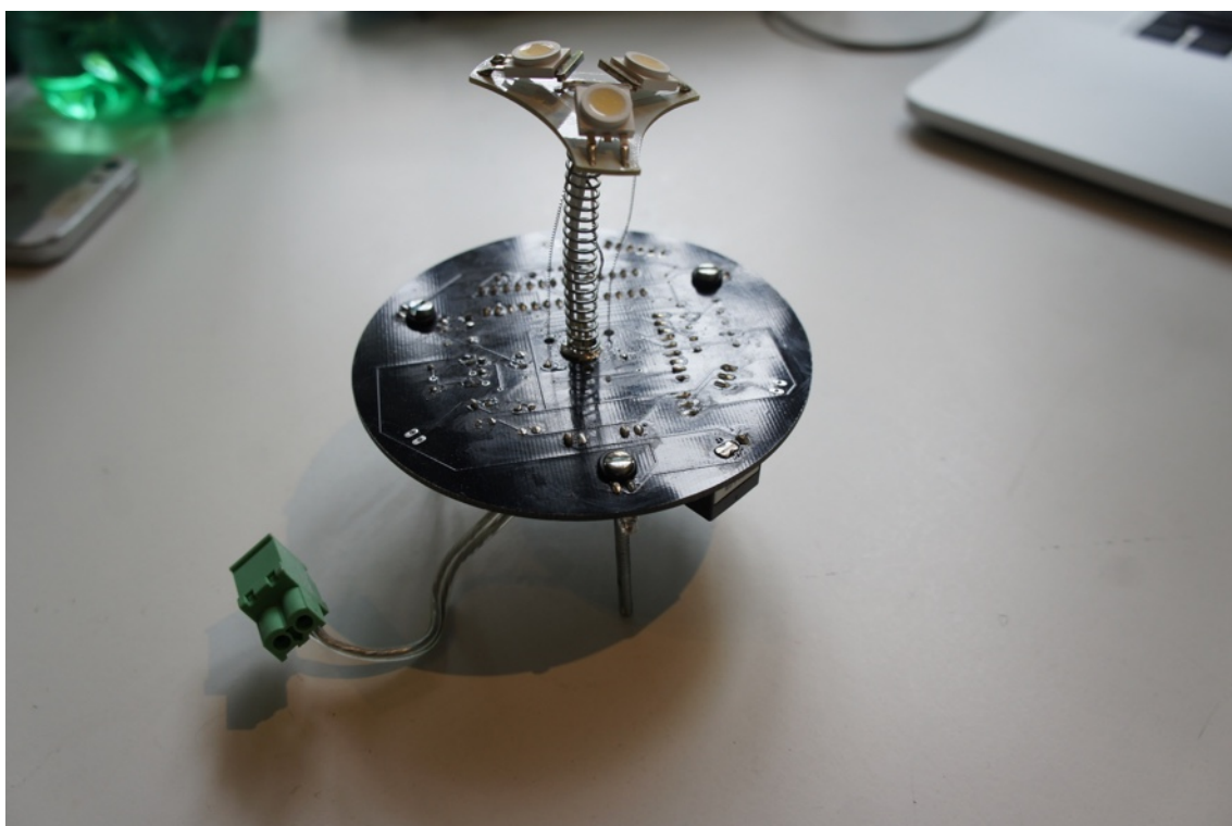
(Top) Custom-made circuit board, also working as the body of the lamp. (Bottom) An assembled Yuen lamp.
