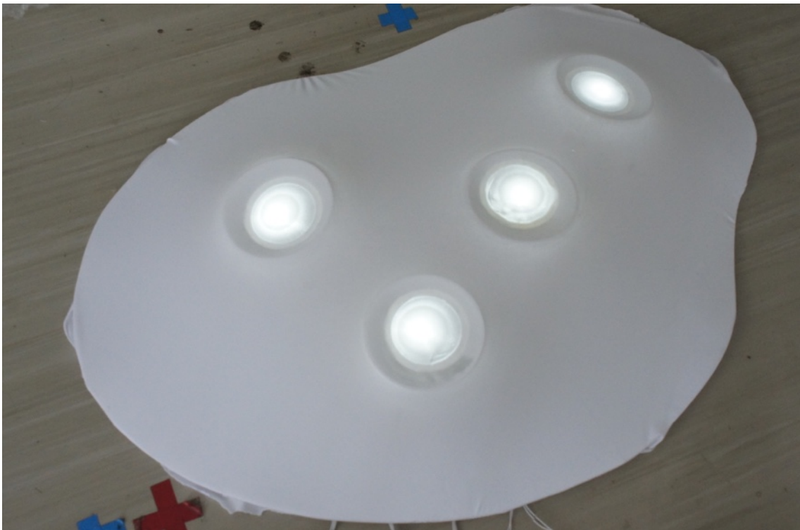
(Top) Firstly testing the idea of putting a light beneath moving elastic fabric. (Bottom) Overview of the test model.
