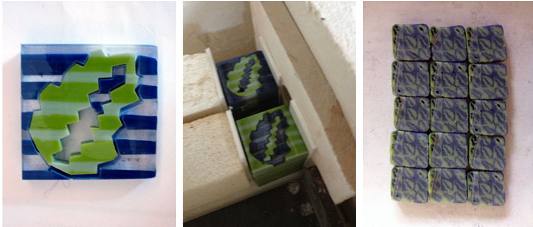
Figure 3.23: (left) Two different waterjet cut segments swapped [Photo: Owen Johnson] Figure 3.24: (middle) Two waterjet cut murrine stacks, in the kiln, [Photo: Owen Johnson] Figure 3.25: (right) Second-stage mosaic tiles from stacks, [Photo: Owen Johnson]
