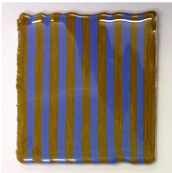
Figure 2.49: (Left) Small pieces of coloured glass ready to fuse, [Photo: Owen Johnson] Figure 2.50: (Middle) Fused glass plate, ready to fold into arch, [Photo: Owen Johnson] Figure 2.51: (Right) Two folded arches stacked into a murrine, [Photo: Owen Johnson]
