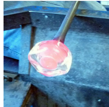
Figure 0.18: (left) The making of a 'collar' or 'post' on a blowing pipe [Sketch: Owen Johnson] (right) A finished glass collar on a glass-blowing pipe [Photo: Owen Johnson]
