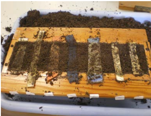
a) b) Fig 3.65 a) & b). Soil boxes after 12 weeks. Bangor University Bio-Composite Centre, 2014
