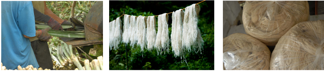
a) b) c) Fig 3.47 a) Decorticating PALF, b) PALF drying in the sun, c) stored PALF. Labo Coop., 2013
