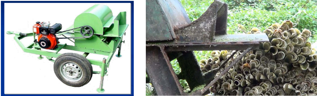
a) b) Fig. 3.44 a) FIDA decorticating machine, b) detail, decorticating machine in Labo Coop field., 2013
