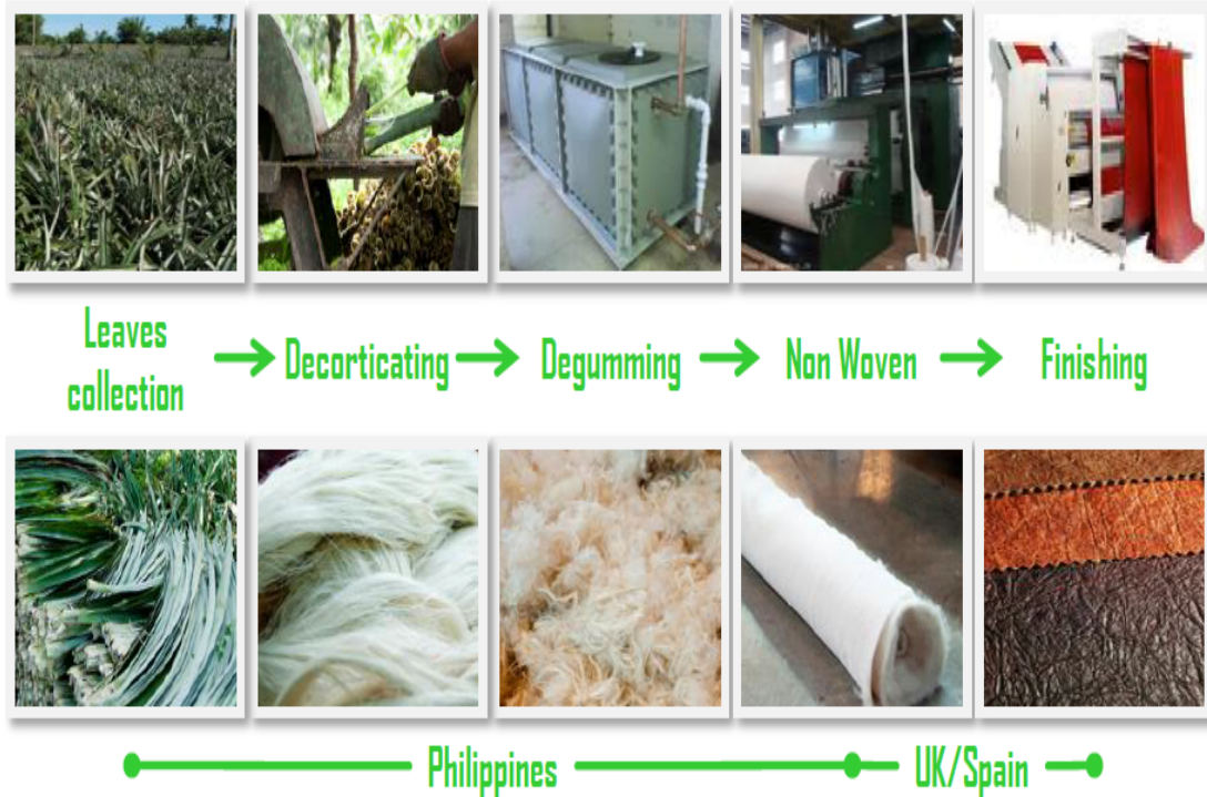
Fig 3.68 Piñatex manufacturing processes, from the field to the final product. Ananas Anam, 2014
