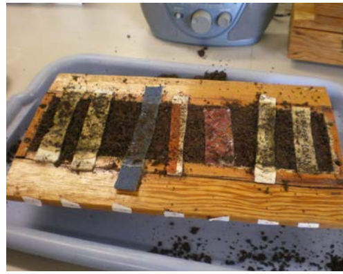
a) b) Fig 3.65 a) & b). Soil boxes after 12 weeks. Bangor University Bio-Composite Centre, 2014
