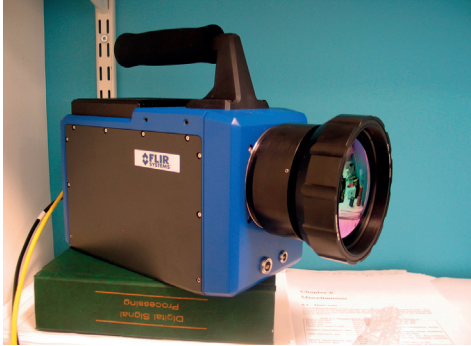
Fig.86: Thermal image camera.
