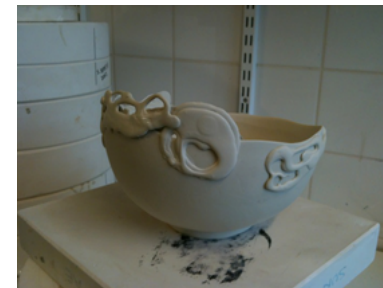
Porcelain, small punch-bowls made by the jolley machine
