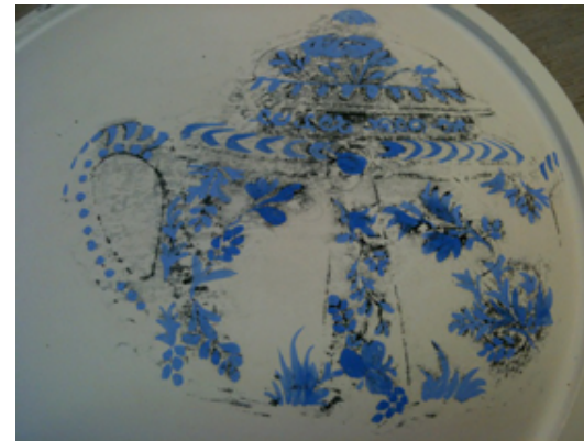
Jigger plaster mould with Flanders blue stain colour.
