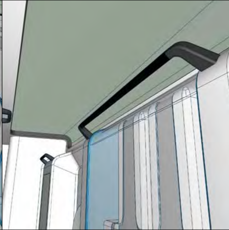
HANDRAILS ALONG ALL THE AMBULANCE
