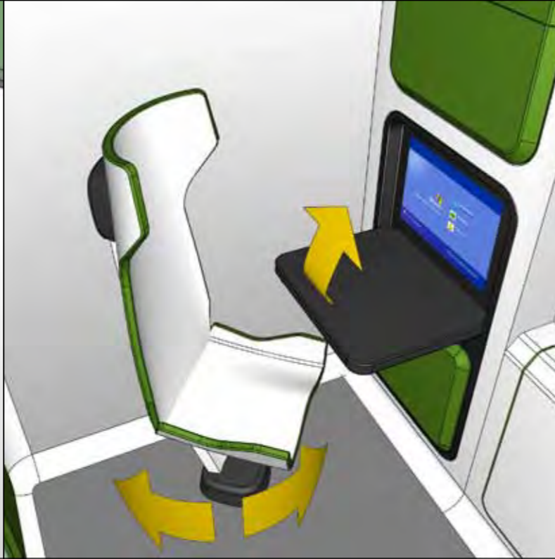
SEAT ROTATES TO FACE A DEPLOYABLE WORKTOP SURFACE AND HIDDEN SCREEN FOR ADMINISTRATIVE WORK.
