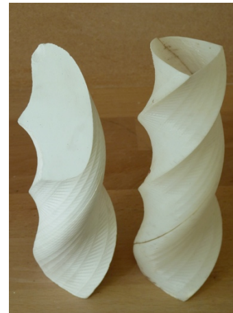
Fig 7. Plaster form (left) and FDM mould made at UCF.
