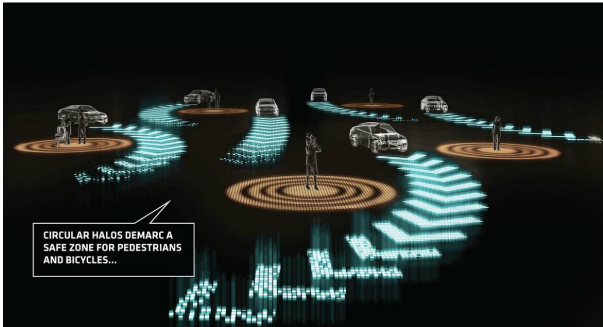
Figure 2-8. Audi project (2011), BIG architects: Based on research into inefficiency of land use as car use increases, this road-free system was proposed 43 . Blue arrows in a media floor indicate where cars can go; brown circles show the safe areas for people.
