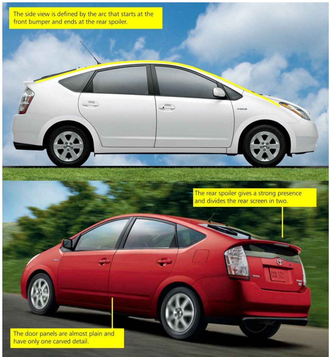
Figure 179: Design analyses of the second generation Prius.
