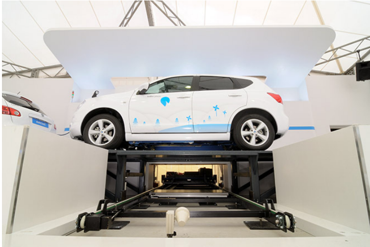
Figure 29: Better Place Electric Car Battery Swap Station (2009).
