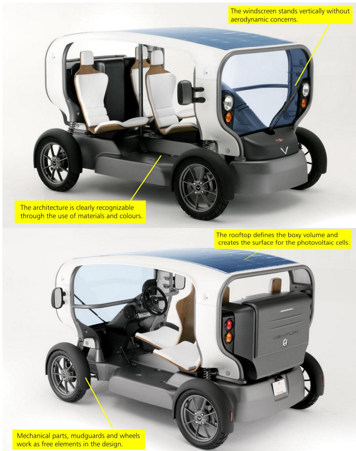
Figure 160: Design analysis of the Venturi Eclectic concept.
