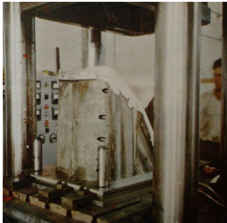
Illustrations 123 and 124. Two stage from the compression moulding process of Magistretti's fibreglass Selene chair at the Artemide factory in the Milanese hinterland, 1970.
