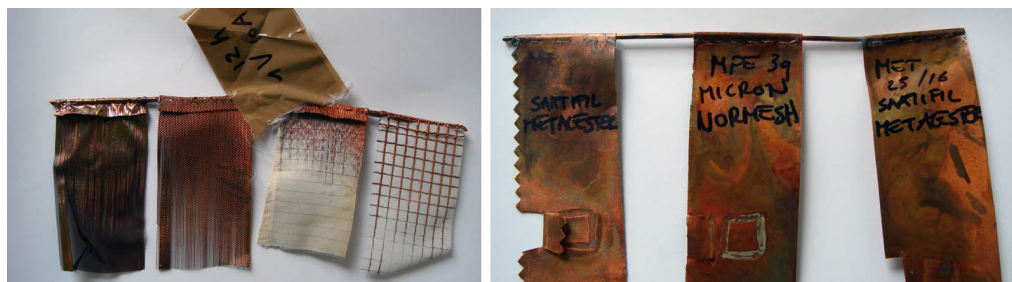
Figure 6.7: Four samples of electroformed textiles with carbon fibre mesh (left) and three samples of nickel-plated textiles (right).
