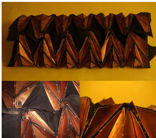
Figure 7.60: MFT bag with magnets could not be used because the platelets are peeling away at the corners.
