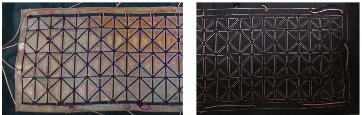
Figure 6.21: Sample of MFT, prepared with self-adhesive copper foil, front (left) and back (right).
