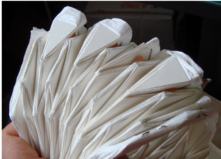
Figure 7.49: Restraints (B) from fig. 7.48 do not keep the edges folded.
