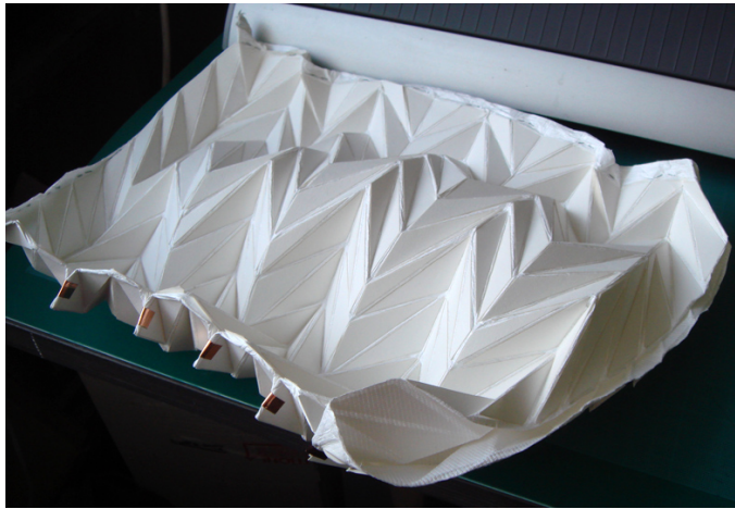
Figure 7.50: Restraints (A and B) from fig. 7.48 prevent the bag from opening properly.
