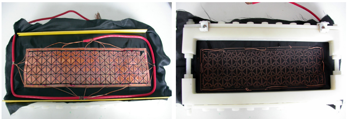
Figure 6.10: Front and back of adjustable nylon frame. The height can be adjusted by turning the bolts on the sides. Bolts on top and bottom keep the fabric in place.
