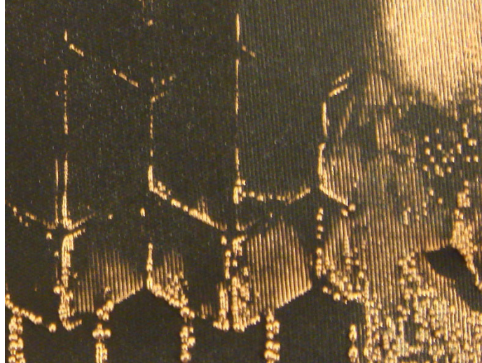
Figure 6.37: Detail: copper built up through the fabric in lines and grains.
