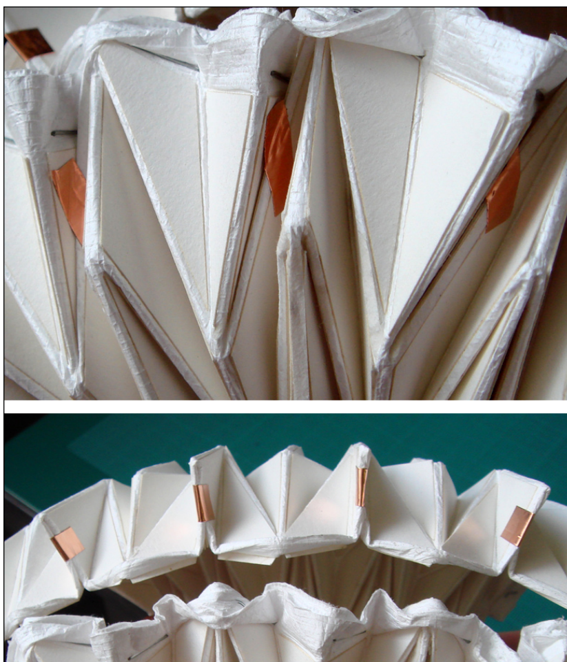
Figure 7.47: Testing restraints to stop the edges from unfolding completely. Top: Fixing two adjoining platelets together (A). Bottom: Making a connection across the edge (B)
