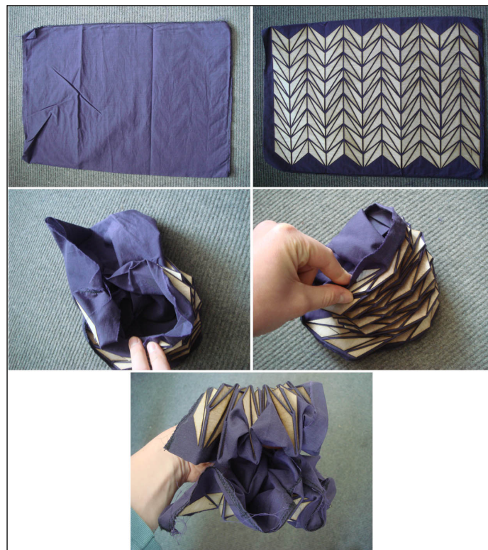
Figure 7.53: Testing edges with removed platelets, third variation (2 platelet removed from each row on either side on the front & all platelets removed from the back of the bag). Plywood on textile.
