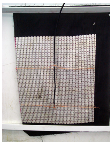
Figure 6.5: Clamping fabric at top and bottom to immerse in solution.
