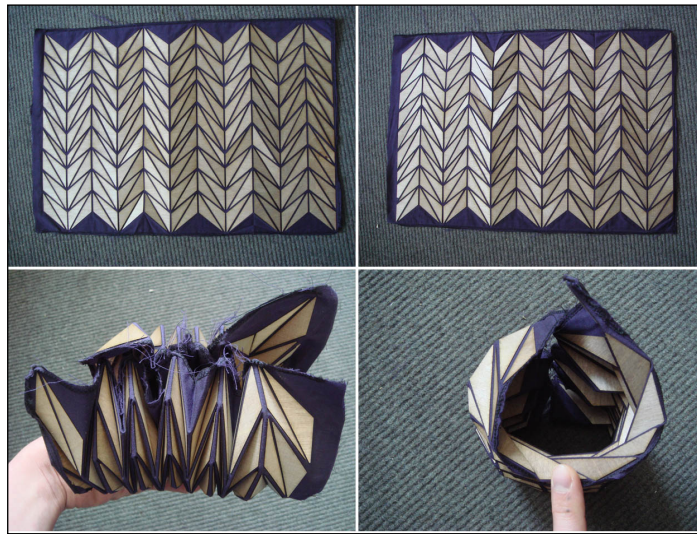
Figure 7.52: Testing edges with removed platelets, second variation (2 platelets removed from each row on either side, front and back identical). Plywood on textile.
