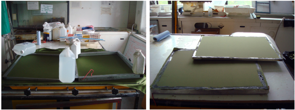
Figure 6.11: The fabric is pre-stretched on a screen stretcher (yellow frame in left image), and electroforming frames are glued on the stretched fabric (left). Weights are applied to keep a good contact between the frames and the fabric. When the glue has dried, the frames are cut out, and are ready to receive a pattern (right).
