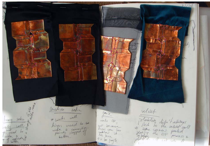
Figure 7.24: Samples of electroforming on a range of fabrics (heavy satin, medium satin, gauze and velvet).
