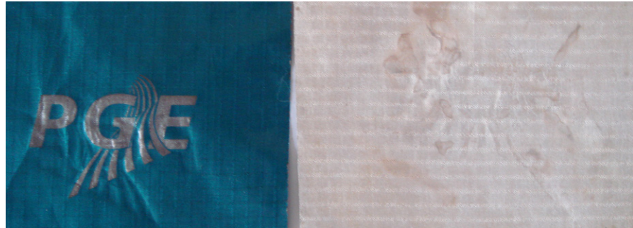
Figure 6.26: Sample of PGE-Adenco before and after electroforming.
