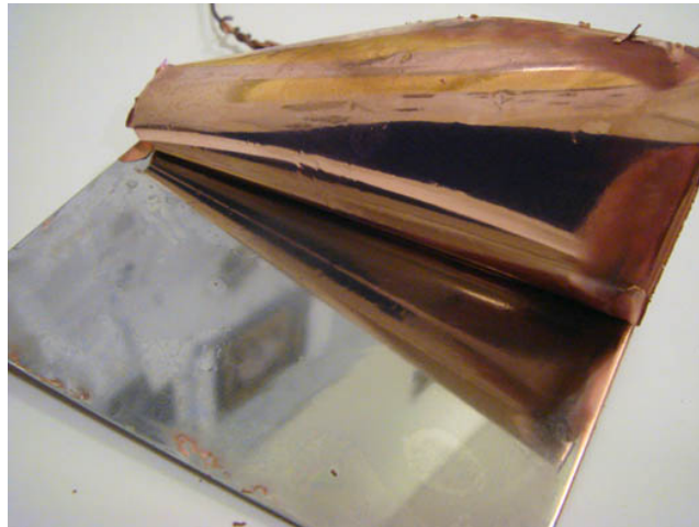
Figure 6.34: Initial test on stainless steel: a thin copper foil is easily removed.
