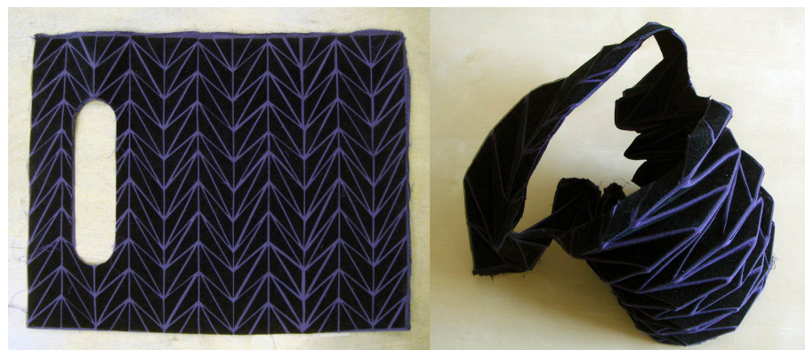
Figure 7.46: Model to test cut-out handle, flat and folded. The handle does not fold well. Iron-on flock and cotton.
