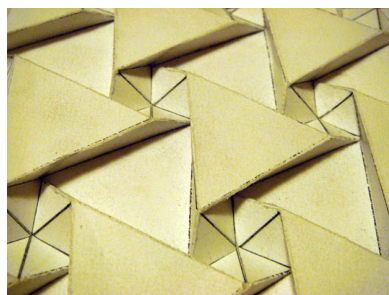
Figure 5.18: Hexagonal platelets are divided into smaller platelets to allow the pattern to be folded in MFT. In paper this is not necessary since the hexagons could flex through the folding process.
