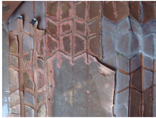
Figure 6.3: Sample of fabric made conductive with dag, and hinges stopped off with wax and marker pen.
