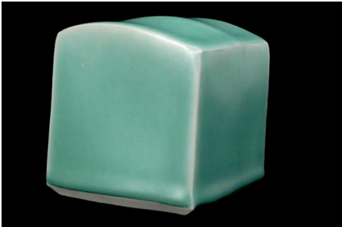
70 + 1% Cu, neutral firing, Cobblestone Nr. 73
