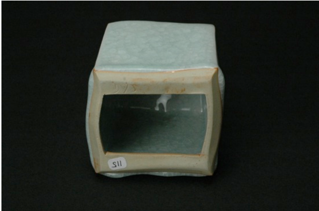
201 + 0.15 Fe, reduction firing 1, stained porcelain body, Cobblestone Nr. 115
