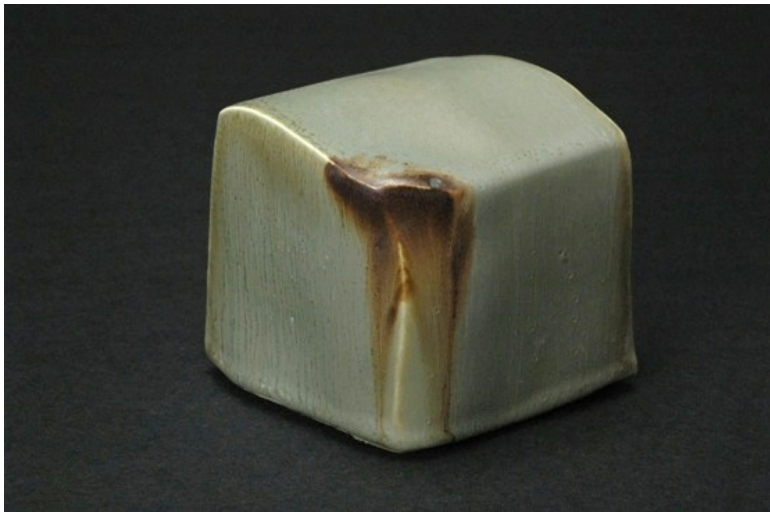
NSD 07/04/2 5Ti 1Fe 0.5 CoCO3 0.25 CrO (new) + iron slip, neutral firing, Cobblestone Nr. 59
