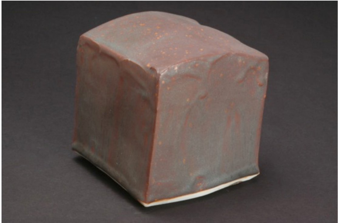
TNSCB 16 5Ti 10Fe, reduction firing, Cobblestone Nr. 154
