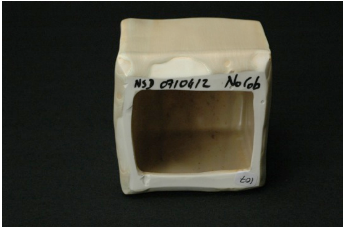
NSD 07/04/2 5Ti 1Fe 0.25 CrO no cobalt, neutral firing, Cobblestone Nr. 107
