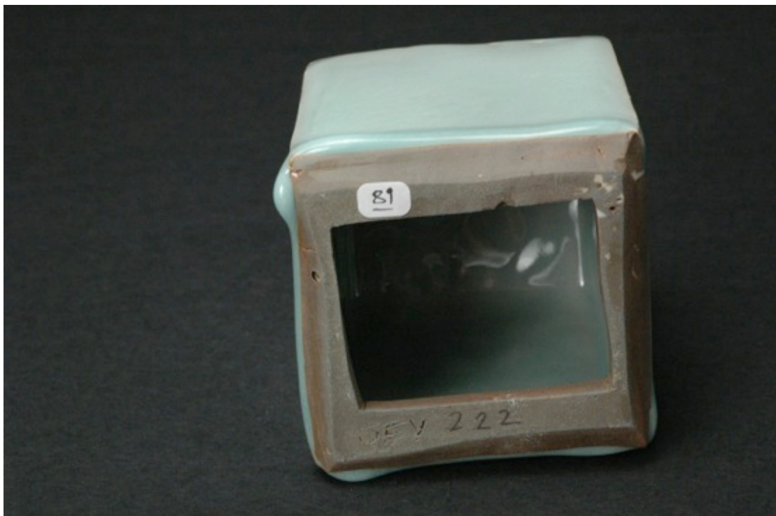
222, reduction firing, stained porcelain body, Cobblestone Nr. 89
