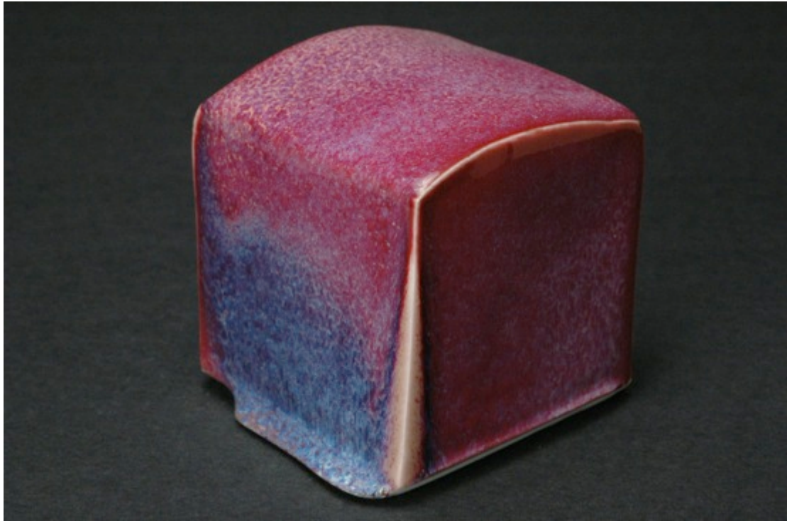
Sam's red (no mistake), ball-milled 30 min, reduction firing, Cobblestone Nr. 24
