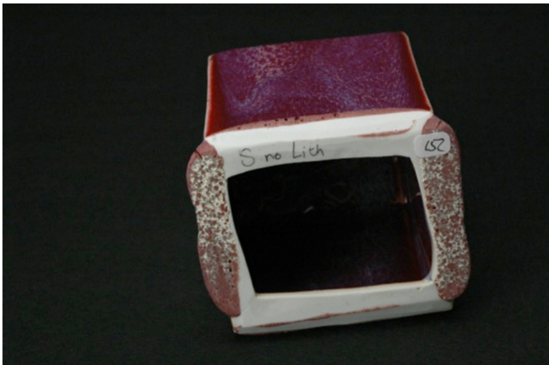
Sams's red no lithium, reduction firing, Cobblestone Nr. 152
