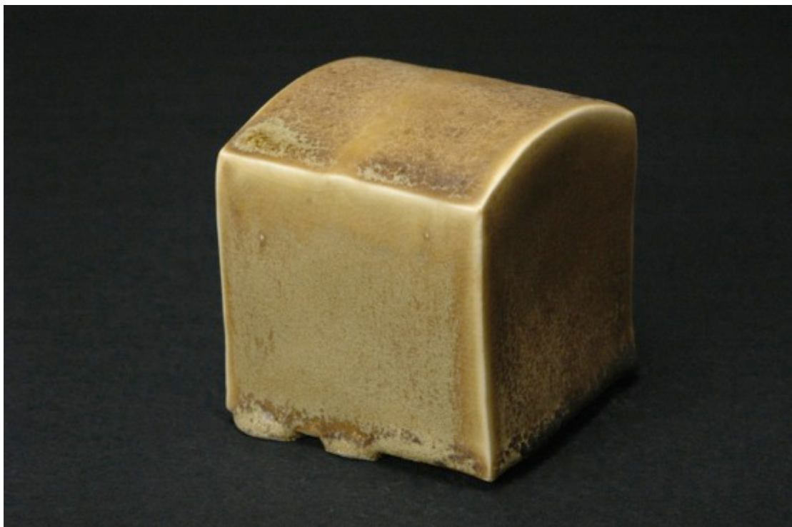
TNSCB 16 3Fe, neutral firing, Cobblestone Nr. 44
