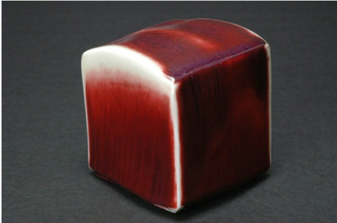
Sams's red no iron, double reduction firing, Cobblestone Nr. 66
