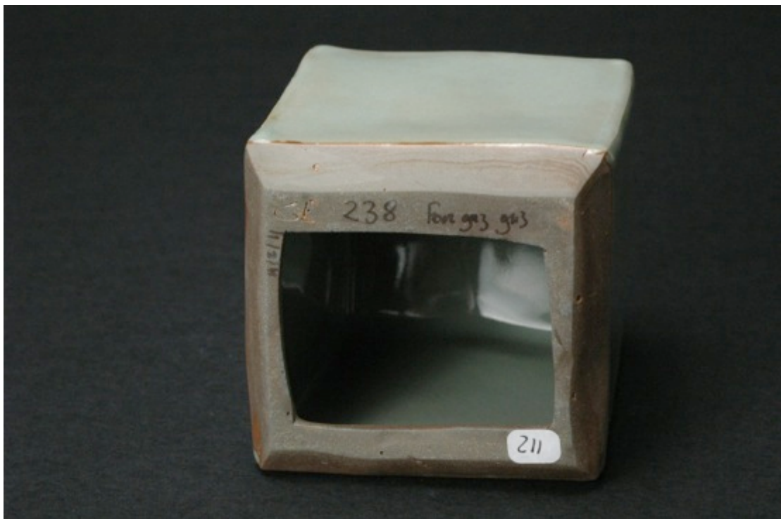
238, reduction firing, stained porcelain body, Cobblestone Nr. 112
