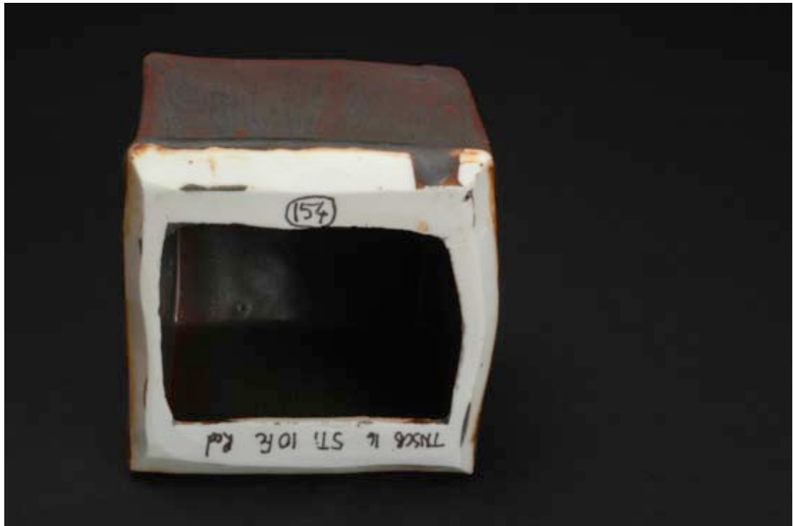
TNSCB 16 5Ti 10Fe, reduction firing, Cobblestone Nr. 154
