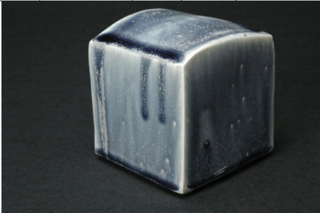
NSD 07/04/2 5Ti 1Fe 0.5 CoCO3 no chrome, neutral firing, Cobblestone Nr. 109
