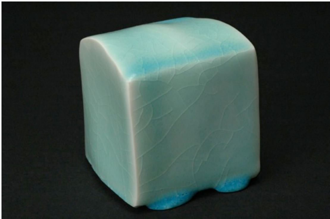
Sams's red no iron, neutral firing, Cobblestone Nr. 9
