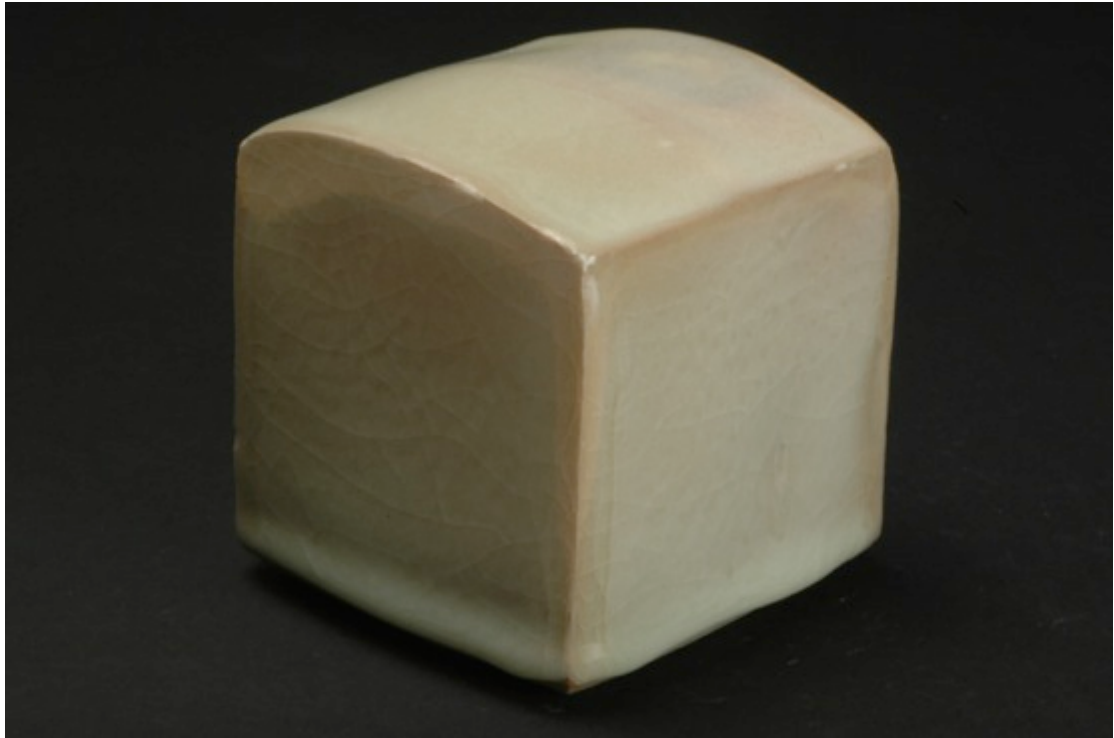
242, light reduction, stained porcelain body, Cobblestone Nr. 175
