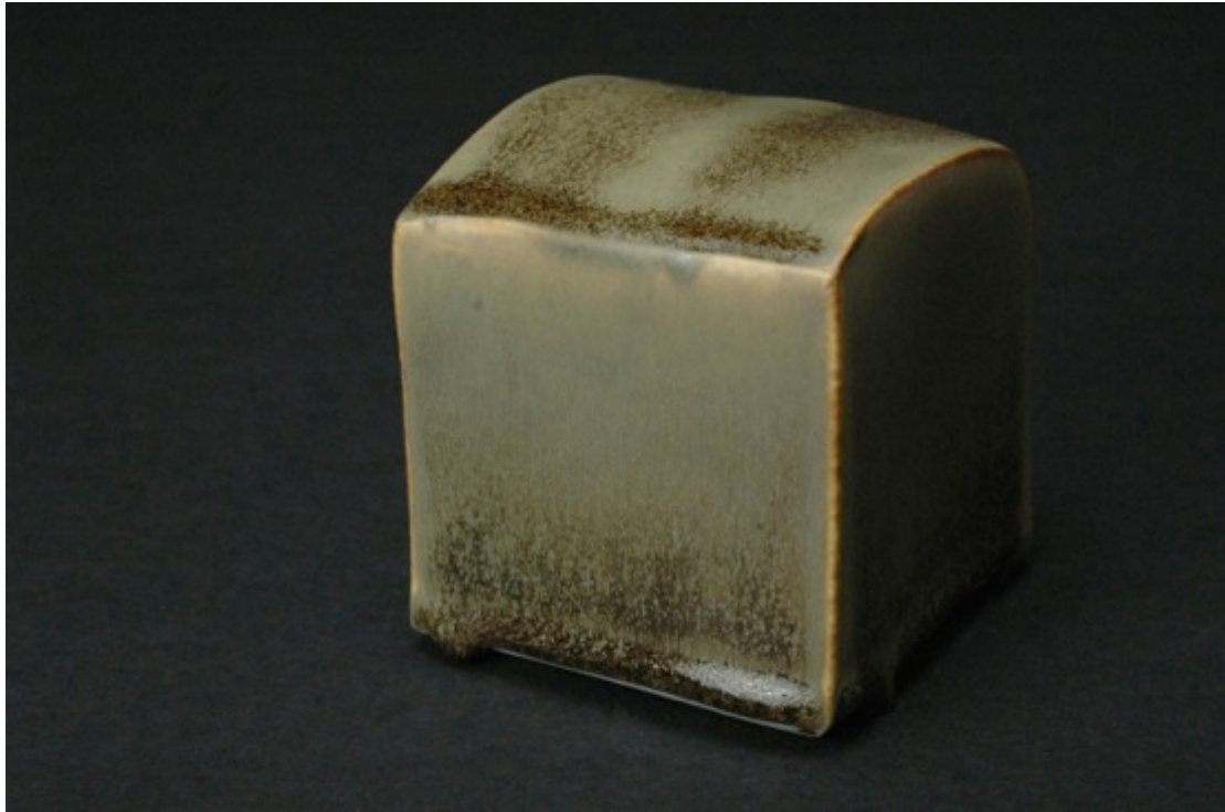
CA 13, reduction firing, Cobblestone Nr. 4
