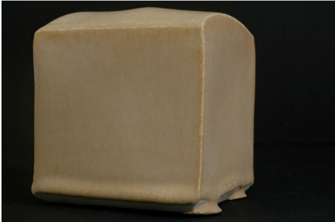
CA 21, reduction firing, Cobblestone Nr. 53
