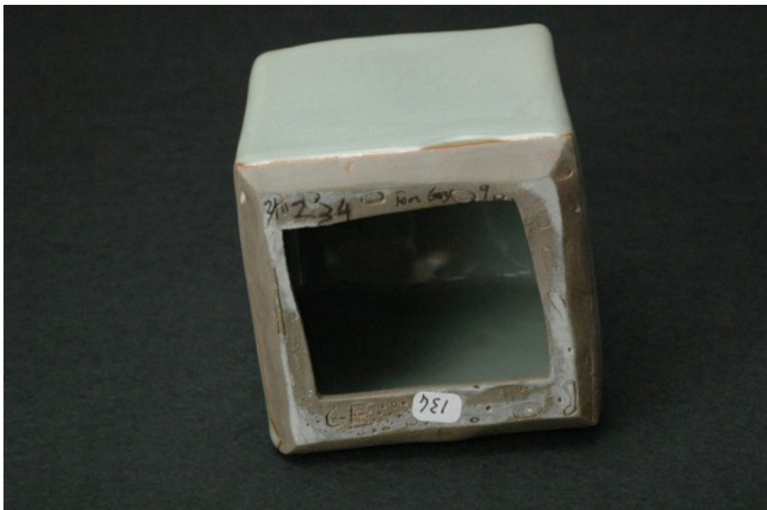
234, reduction firing, stained porcelain body, Cobblestone Nr. 134
