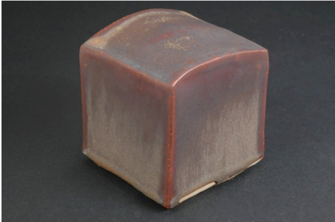
TNSCB 16 5Ti 10Fe, reduction firing, Cobblestone Nr. 136
