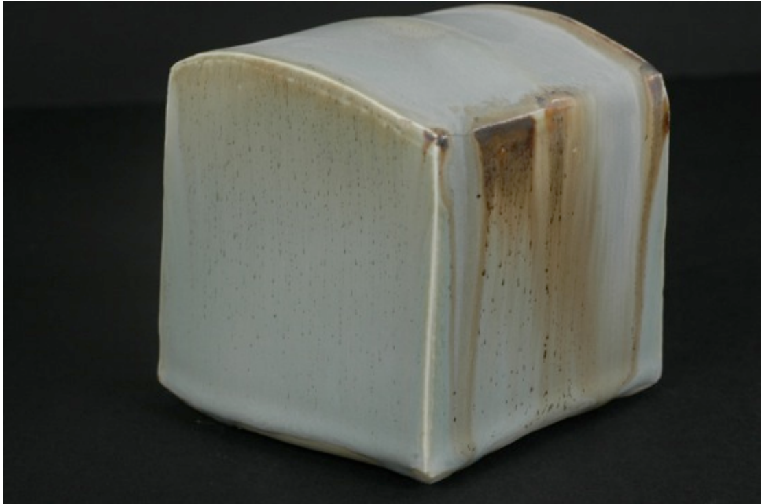
NSD 07/04/2 5Ti 1Fe 0.5 CoCO3 0.25 CrO + iron slip, neutral firing, Cobblestone Nr. 23
