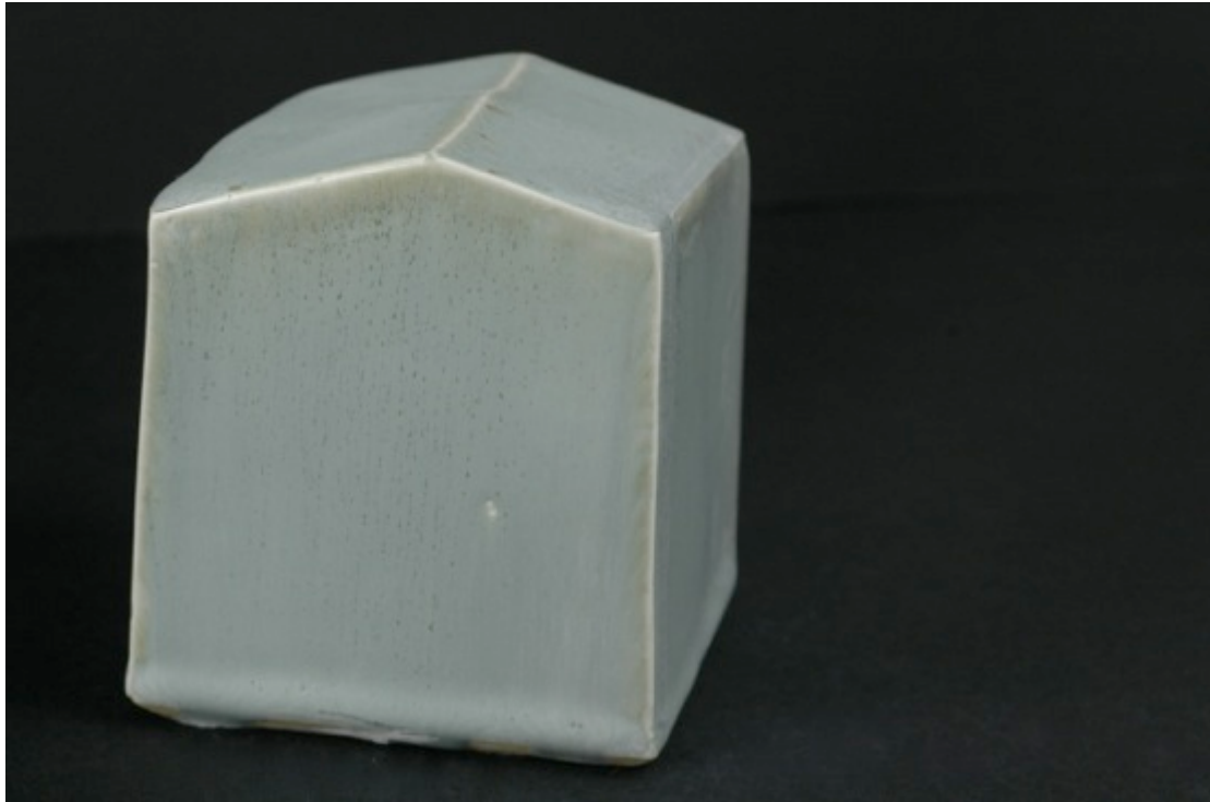
NSD 07/04/2 5Ti 1Fe 0.5 CoCO3 0.25 CrO, neutral firing, Cobblestone Nr. 176
