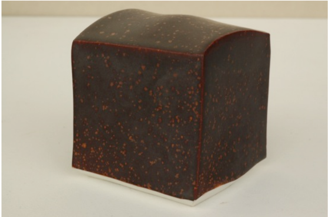
TNSCB 16 5Ti 10Fe, reduction firing, Cobblestone Nr. 200
