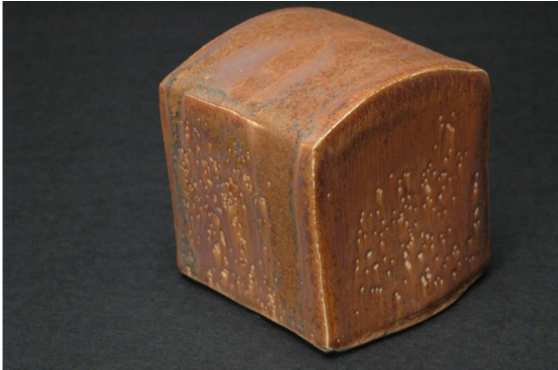
TNSCB 16 5Ti 10Fe, neutral firing, Cobblestone Nr. 27
