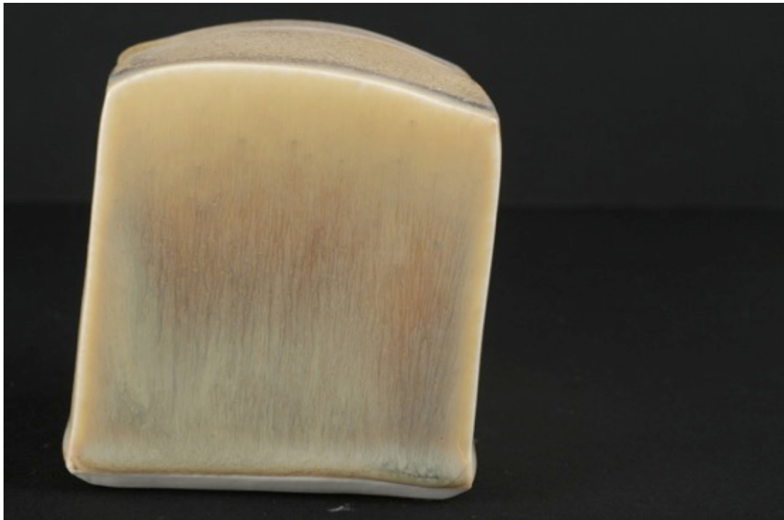
TNSCB 16 3Ti 3Fe, neutral firing, Cobblestone Nr. 96
