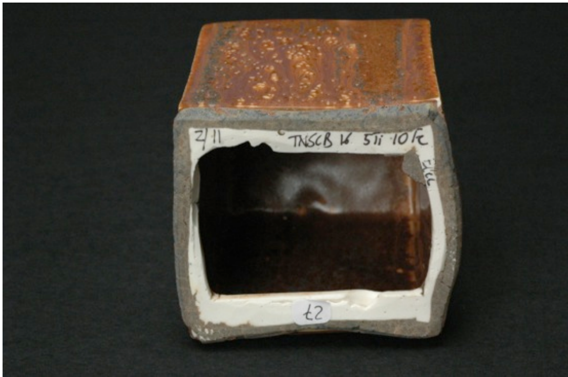
TNSCB 16 5Ti 10Fe, neutral firing, Cobblestone Nr. 27
