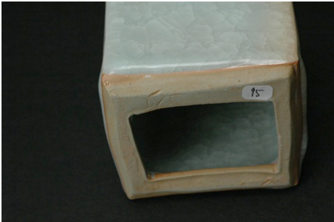
201 + 0.15 Fe, reduction firing 2, stained porcelain body, Cobblestone Nr. 95
