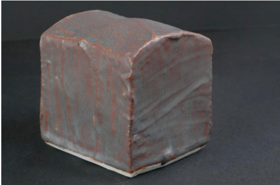
TNSCB 16 5Ti 10Fe, reduction firing, Cobblestone Nr. 78
