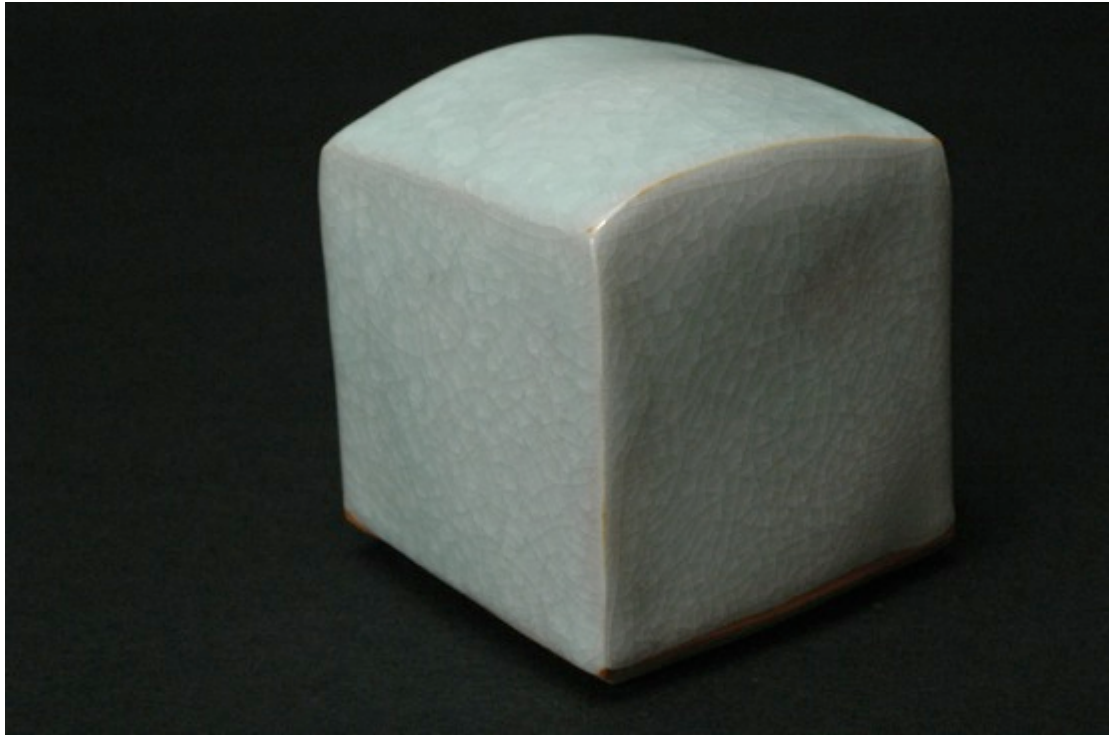
201 + 0.15 Fe, reduction firing 1, stained porcelain body, Cobblestone Nr. 92
