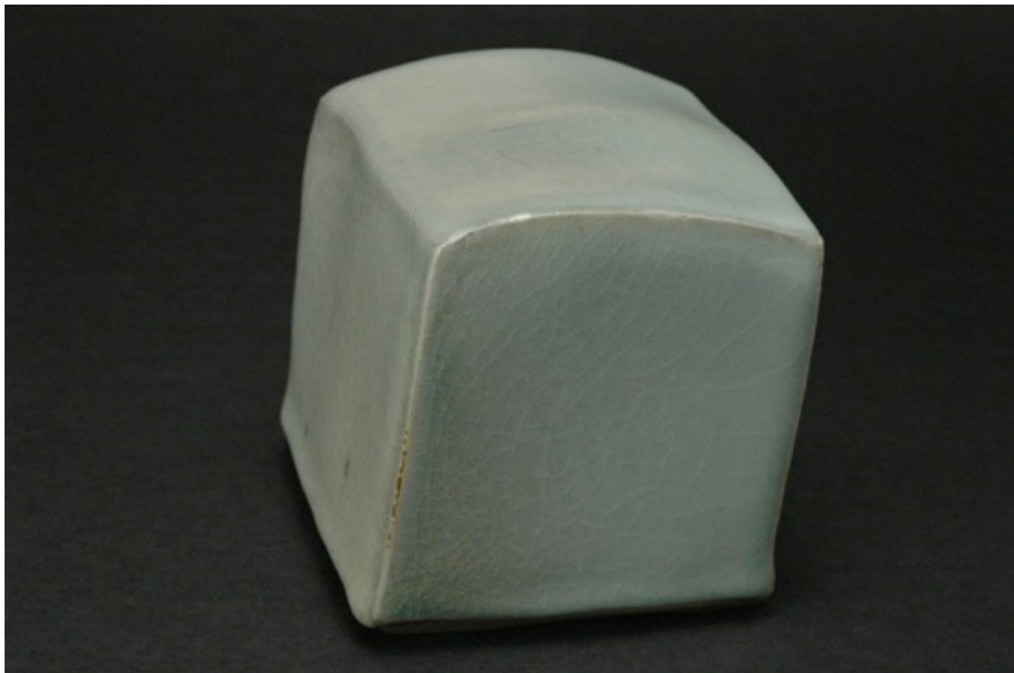
241, light reduction, stained porcelain body, Cobblestone Nr. 195
