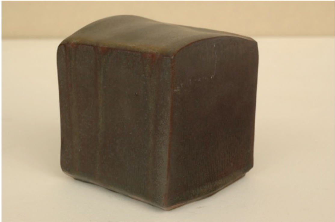
TNSCB 16 5Ti 10Fe, reduction firing, stained porcelain body, Cobblestone Nr. 185
