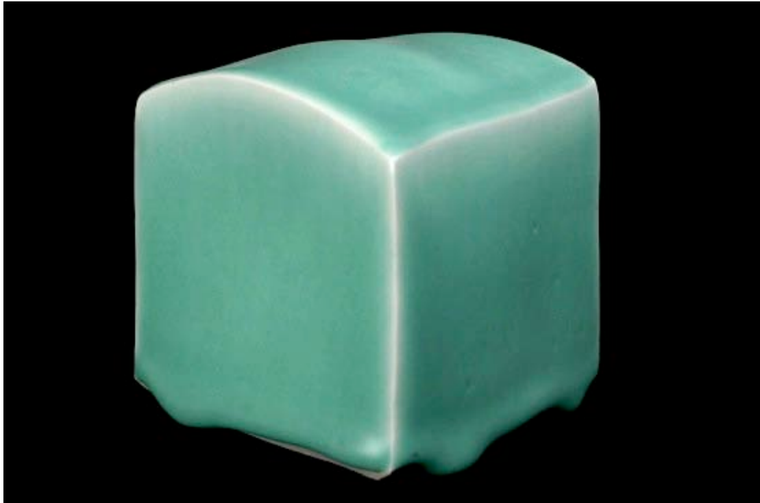
70 + 1% Cu, neutral firing, Cobblestone Nr. 73
