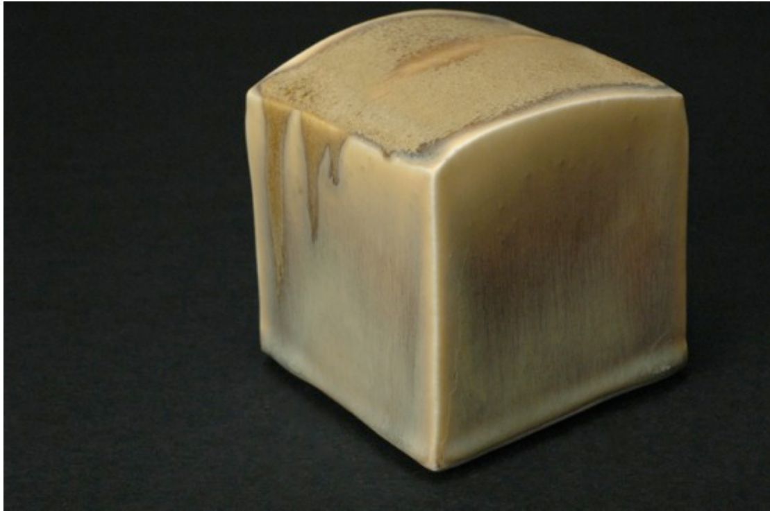
TNSCB 16 3Ti 3Fe, neutral firing, Cobblestone Nr. 96
