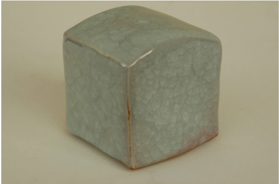
201 + 0.15 Fe, reduction firing 1, stained porcelain body, Cobblestone Nr. 191
