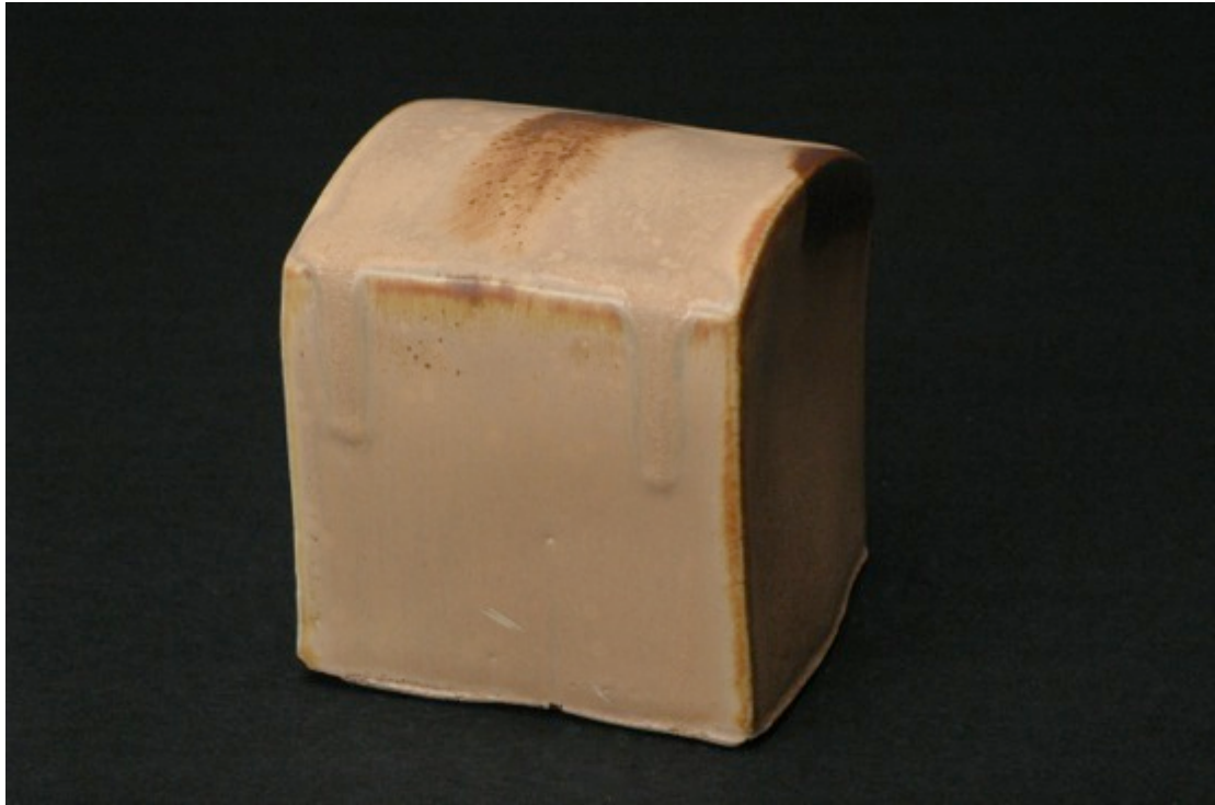
TNSCB 16 5Ti 7Fe + iron slip, neutral firing, Cobblestone Nr. 6
