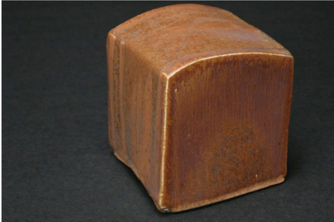
TNSCB 16 5Ti 10Fe, neutral firing, Cobblestone Nr. 27
