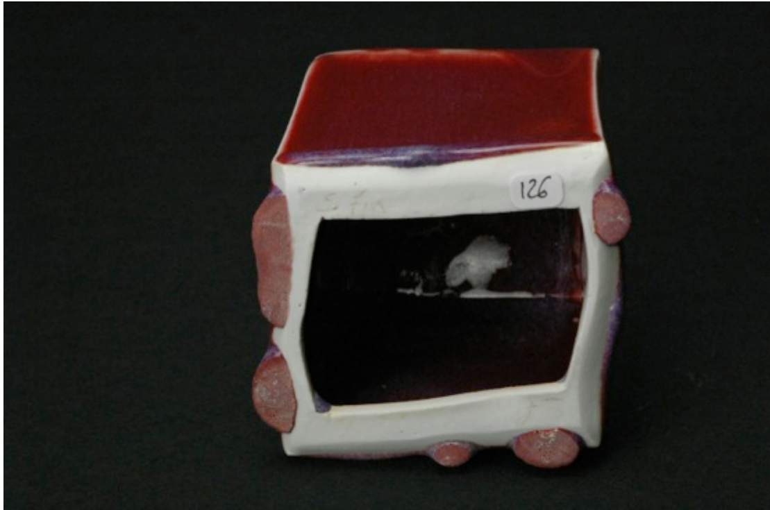
Sam's red (no mistake), thin layered glaze, reduction firing, Cobblestone Nr. 126
