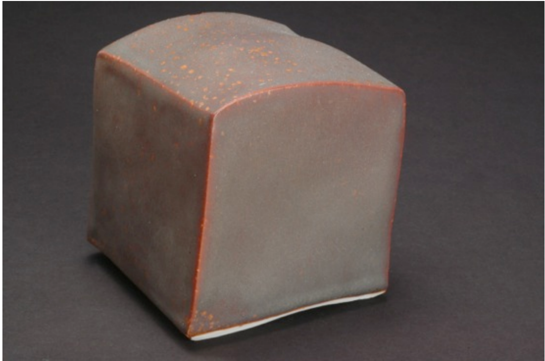
TNSCB 16 5Ti 10Fe, reduction firing, Cobblestone Nr. 41
