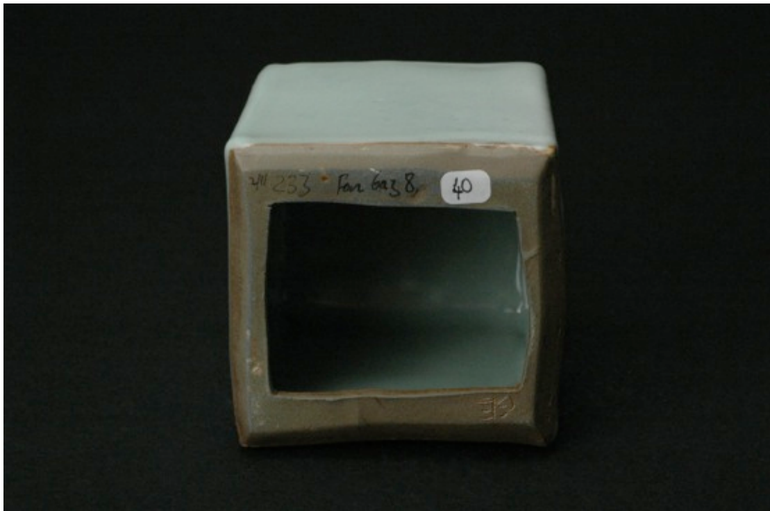
233, reduction firing, stained porcelain body, Cobblestone Nr. 40
