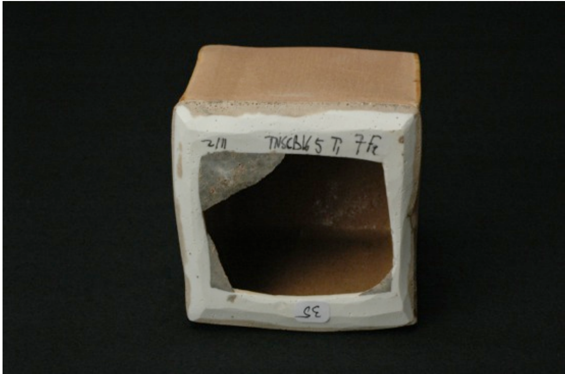
TNSCB 16 5Ti 7Fe, neutral firing, Cobblestone Nr. 35
