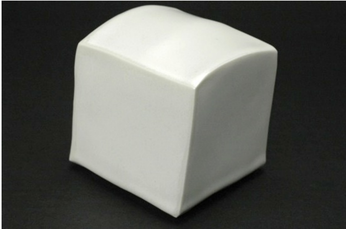
TKWT 50, weak reduction firing, Cobblestone Nr. 189
