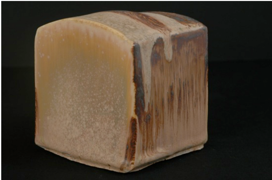
TNSCB 16 5Ru 5Fe + iron slip, neutral firing, Cobblestone Nr. 75
