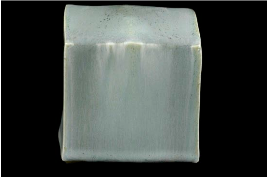
NSD 07/04/2 5Ti 1Fe 0.5 CoCO3 0.25 CrO, neutral firing, Cobblestone Nr. 116
