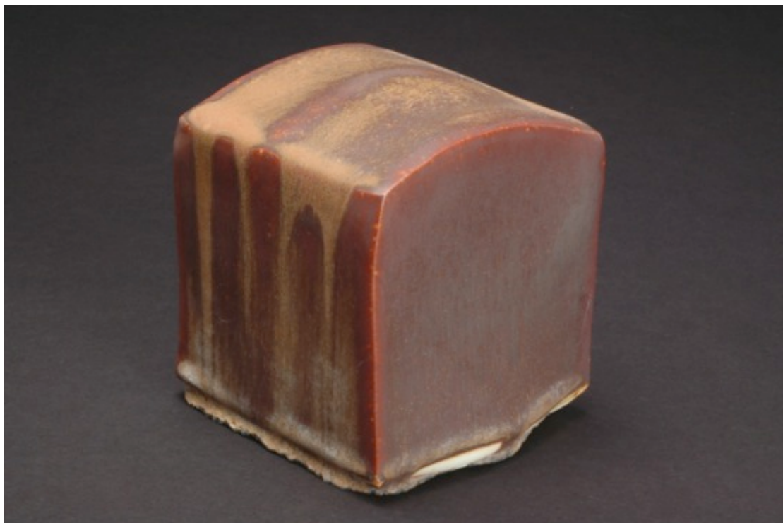
TNSCB 16 5Ti 10Fe, reduction firing, Cobblestone Nr. 36
