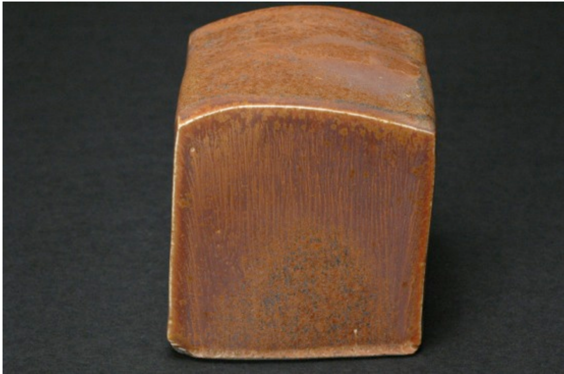
TNSCB 16 5Ti 10Fe, neutral firing, Cobblestone Nr. 27
