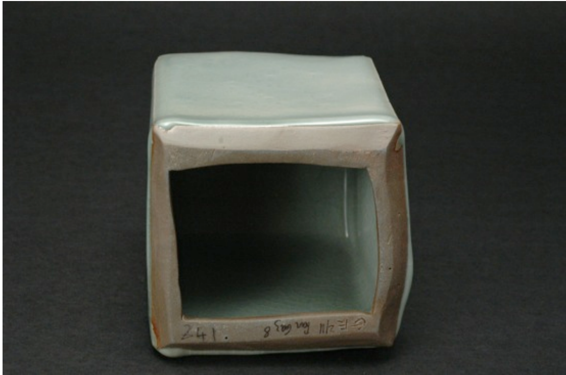
241, light reduction, stained porcelain body, Cobblestone Nr. 195
