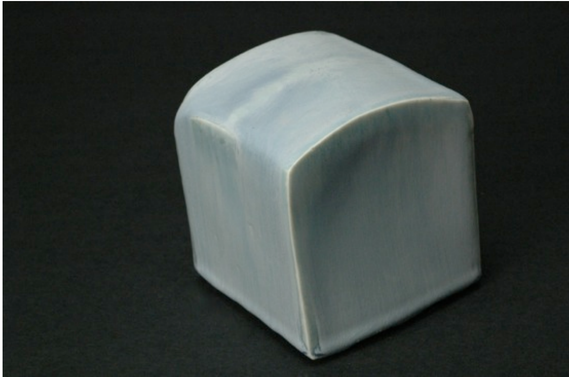
NSD 07/04/2 5Ti 0.5 CoCO3 0.25 CrO no iron, neutral firing, Cobblestone Nr. 137
