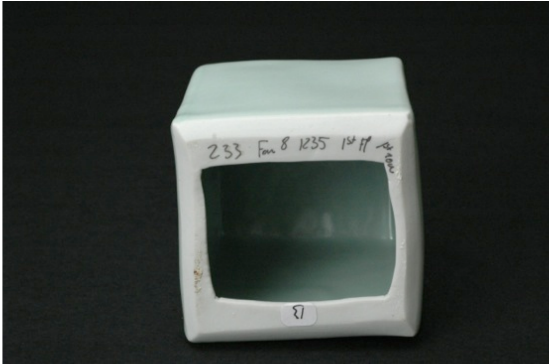
233, reduction firing, white porcelain body, Cobblestone Nr. 13
