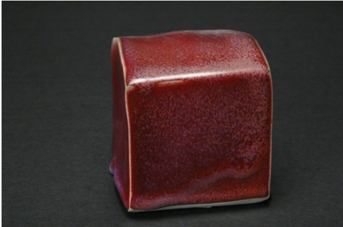
Sam's red (no mistake), medium layered glaze, reduction firing, Cobblestone Nr. 158
