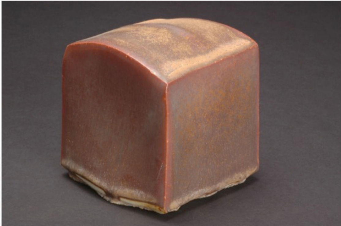
TNSCB 16 5Ti 10Fe, reduction firing, Cobblestone Nr. 36
