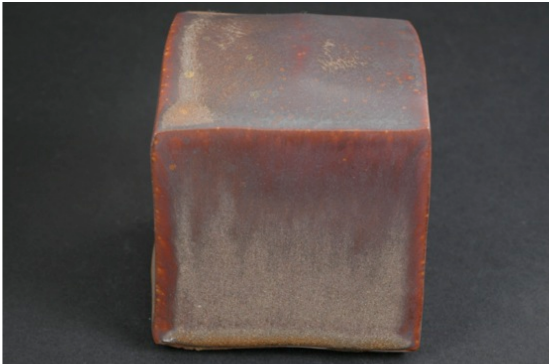
TNSCB 16 5Ti 10Fe, reduction firing, Cobblestone Nr. 136
