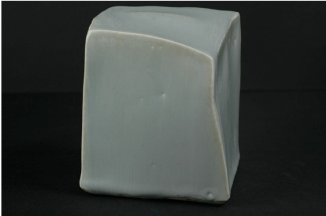
NSD 07/04/2 5Ti 1Fe 0.5 CoCO3 0.25 CrO, neutral firing, Cobblestone no Nr.
