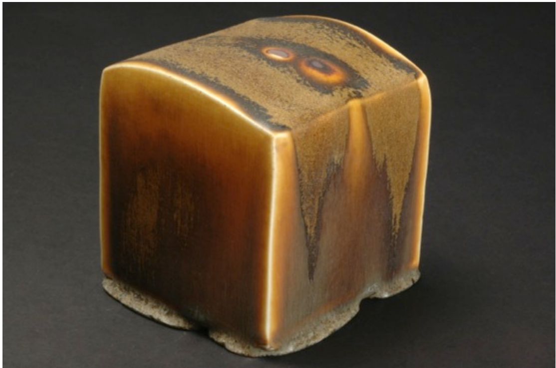
TNSCB 16 7Fe, neutral firing, Cobblestone Nr. 88
