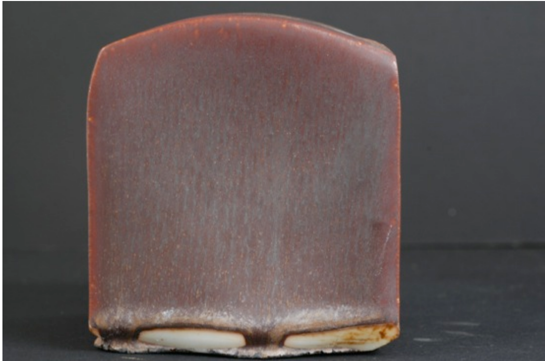
TNSCB 16 5Ti 10Fe, reduction firing, Cobblestone Nr. 36
