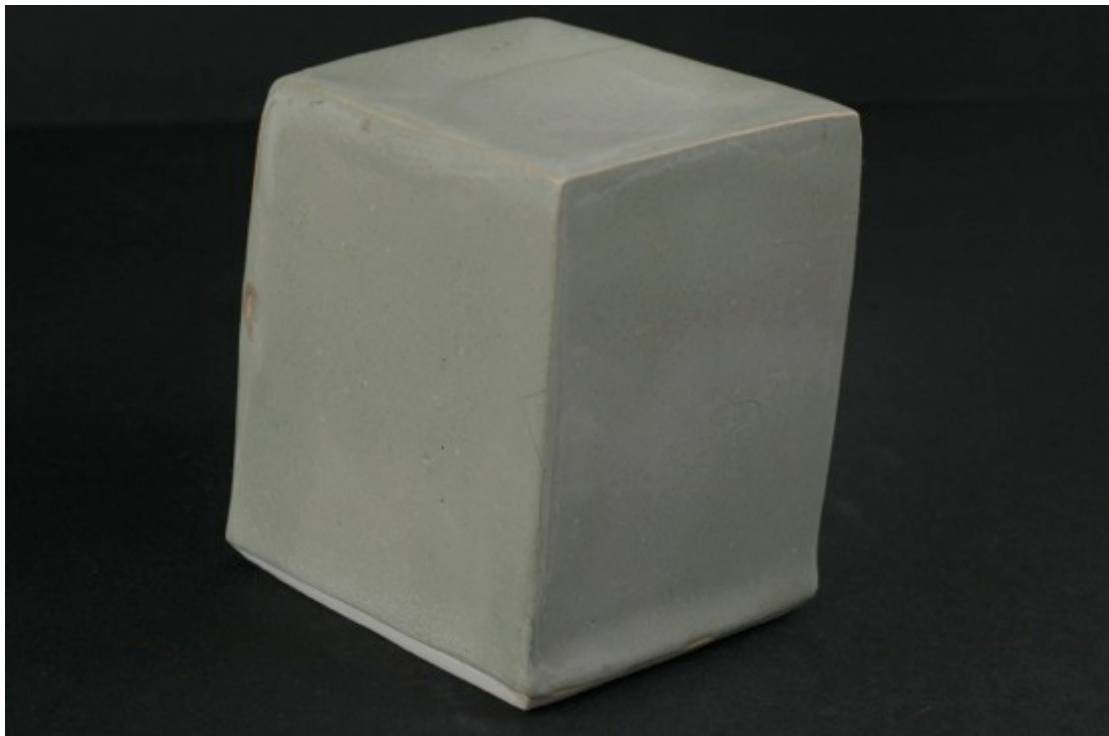
NSD 07/3 3Ti 3Cr, neutral firing, Cobblestone Nr. 68
