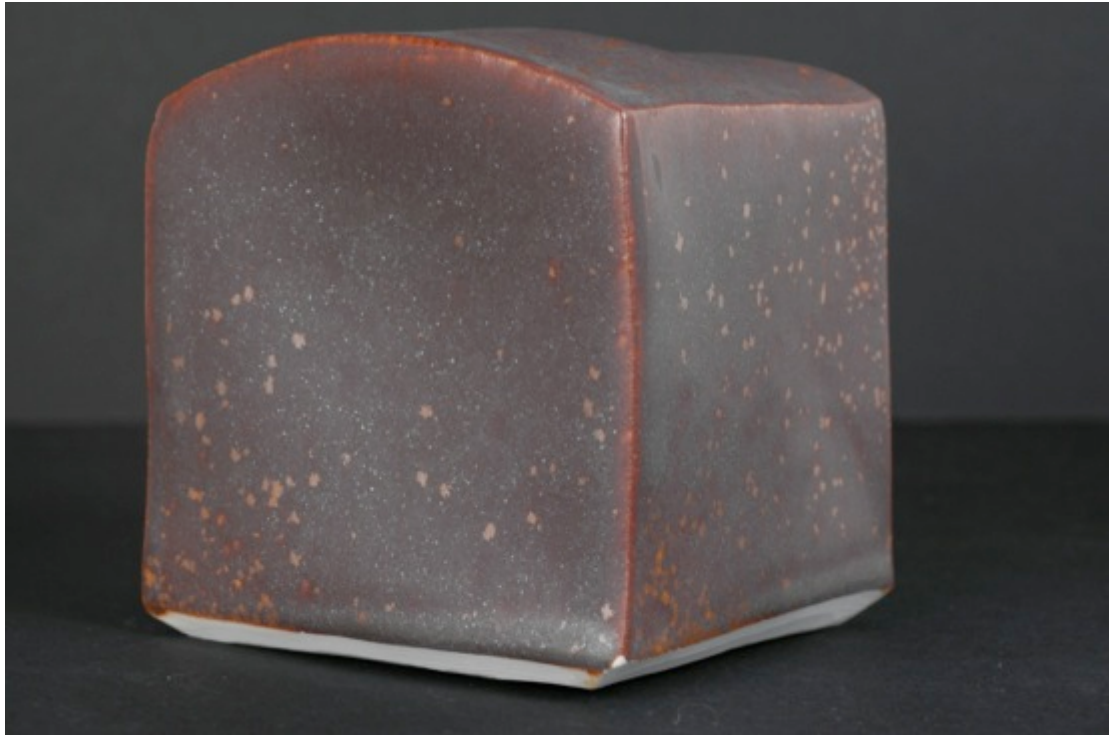
TNSCB 16 5Ti 10Fe, reduction firing, Cobblestone Nr. 22
