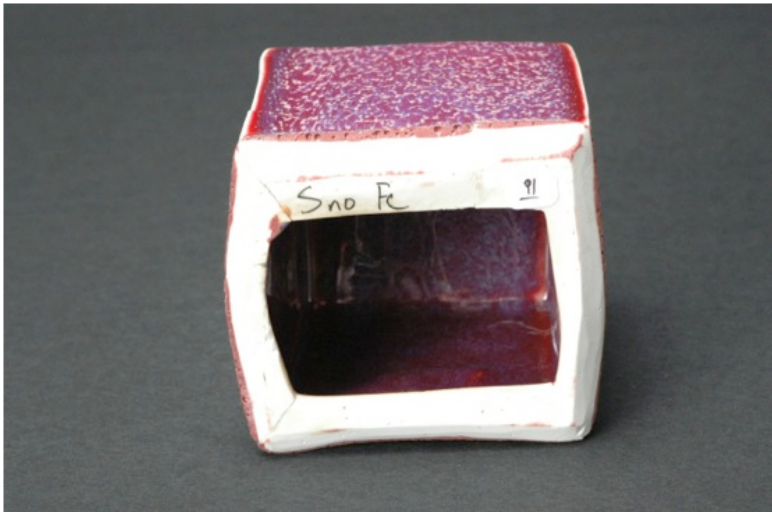
Sams's red no iron, reduction firing, Cobblestone Nr. 91
