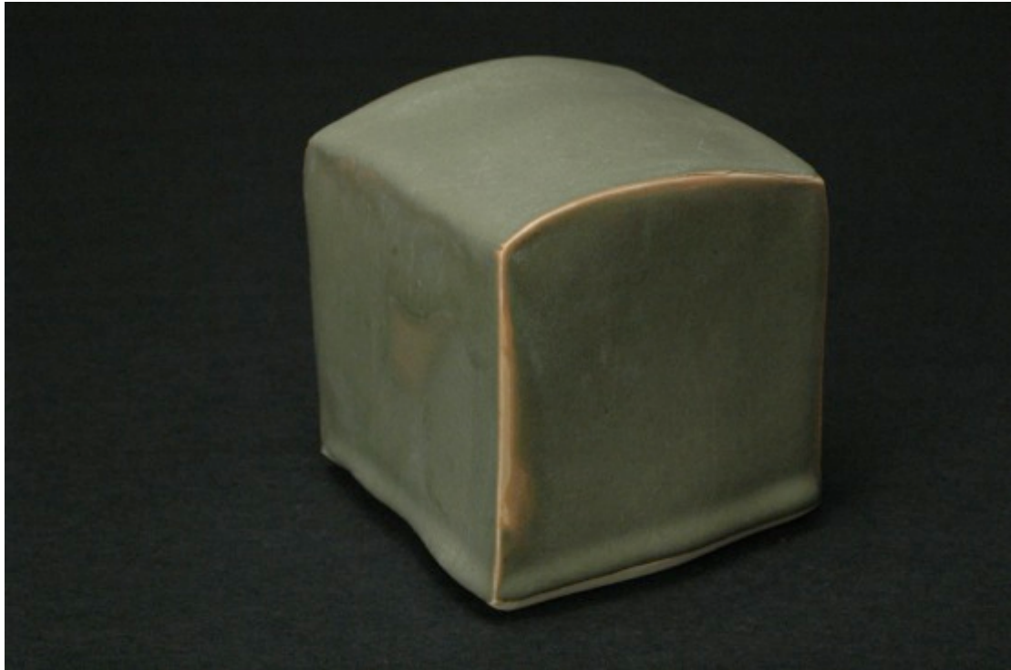
NSD 07/3 3Ti 3Cr, neutral firing, Cobblestone Nr. 57
