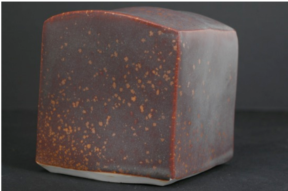
TNSCB 16 5Ti 10Fe, reduction firing, Cobblestone Nr. 22
