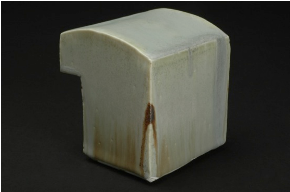
NSD 07/04/2 5Ti 1Fe 0.5 CoCO3 0.25 CrO, neutral firing, Cobblestone Nr. 178
