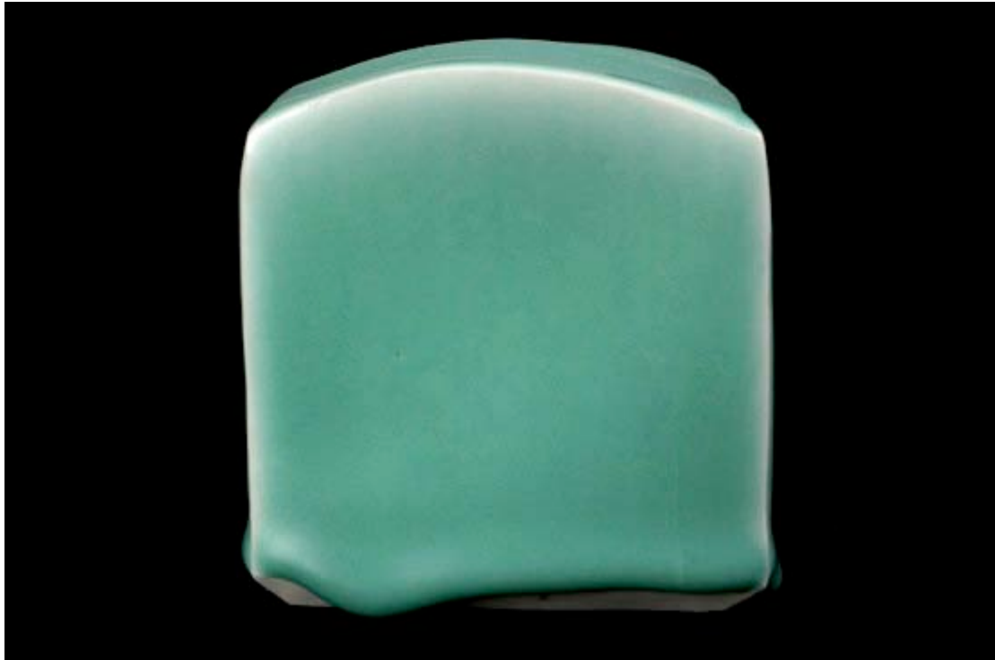
70 + 1% Cu, neutral firing, Cobblestone Nr. 73
