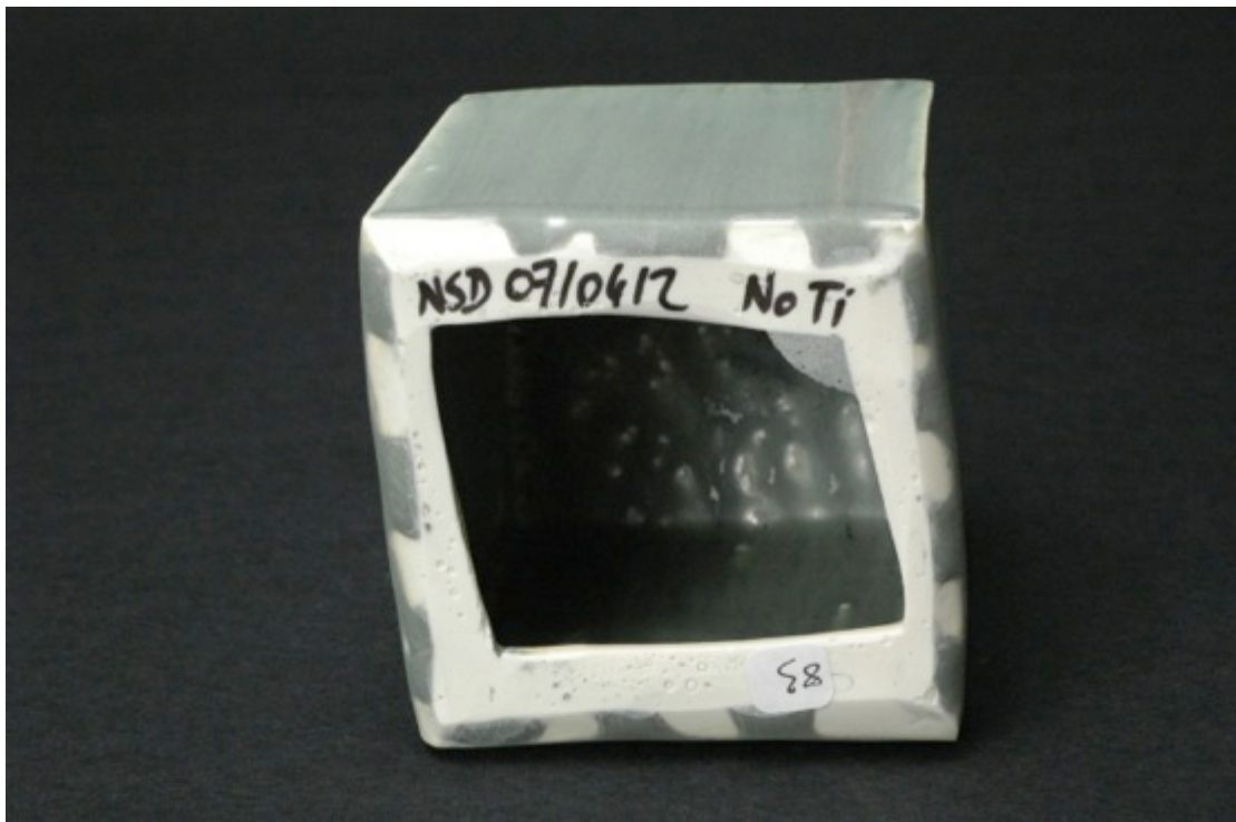
NSD 07/04/2 1Fe 0.5 CoCO3 0.25 CrO no titanium, neutral firing, Cobblestone Nr. 83
