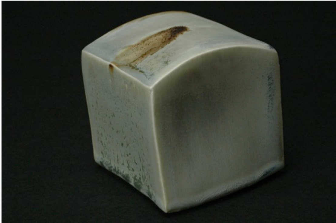
NSD 07/04/2 5Ti 1Fe 0.5 CoCO 3 0.25 CrO + iron slip, neutral firing, Cobblestone Nr. 105
