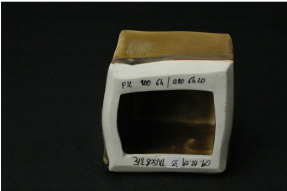
TNSCB 16 3Fe, neutral firing, Cobblestone Nr. 38
