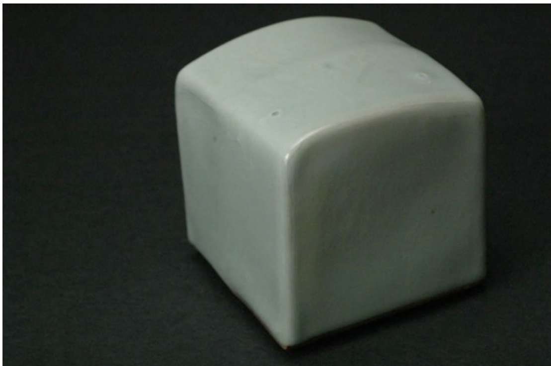
234, reduction firing, stained porcelain body, Cobblestone Nr. 134
