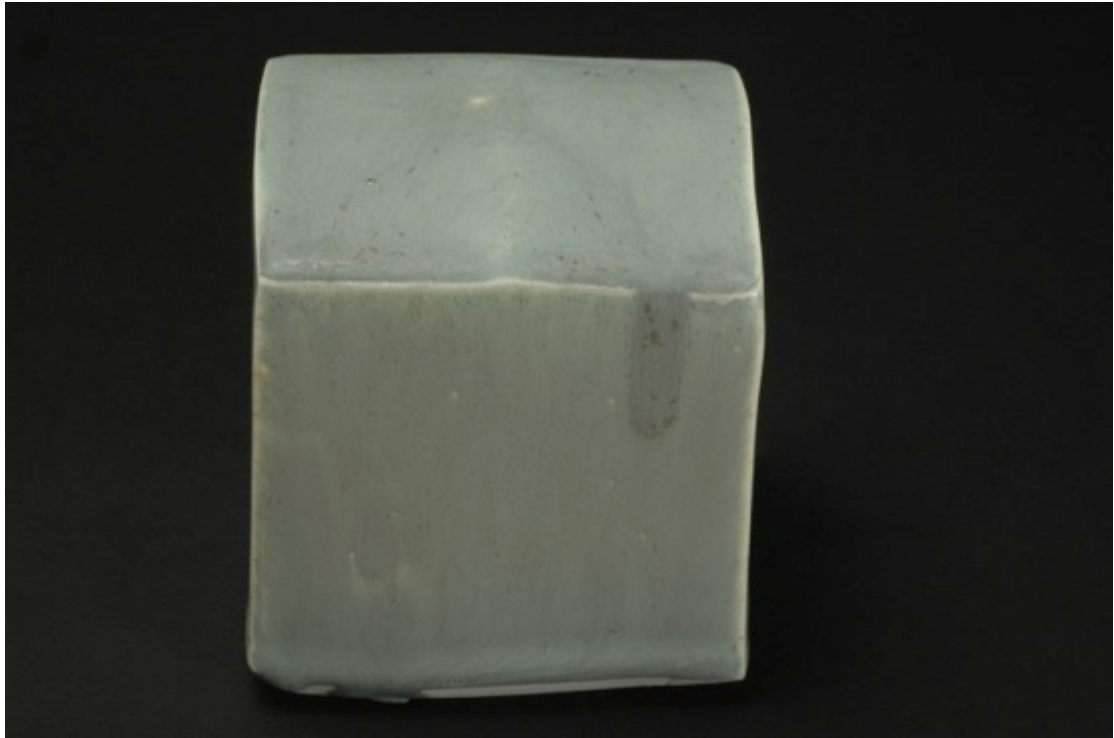
NSD 07/04/2 5Ti 1Fe 0.5 CoCO 3 0.25 CrO, neutral firing, Cobblestone Nr. 42
