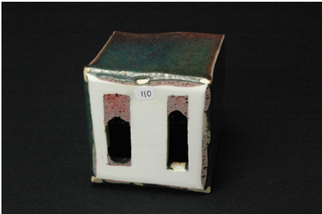
Sam's red 5 Cu, reduction firing, Cobblestone Nr. 110
