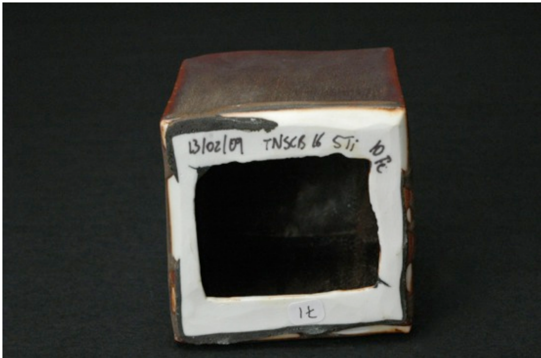
TNSCB 16 5Ti 10Fe, reduction firing, Cobblestone Nr. 71
