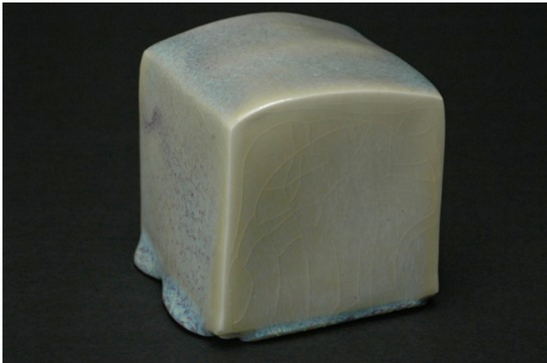
Sam's red (no mistake), light reduction firing, Cobblestone Nr. 170
