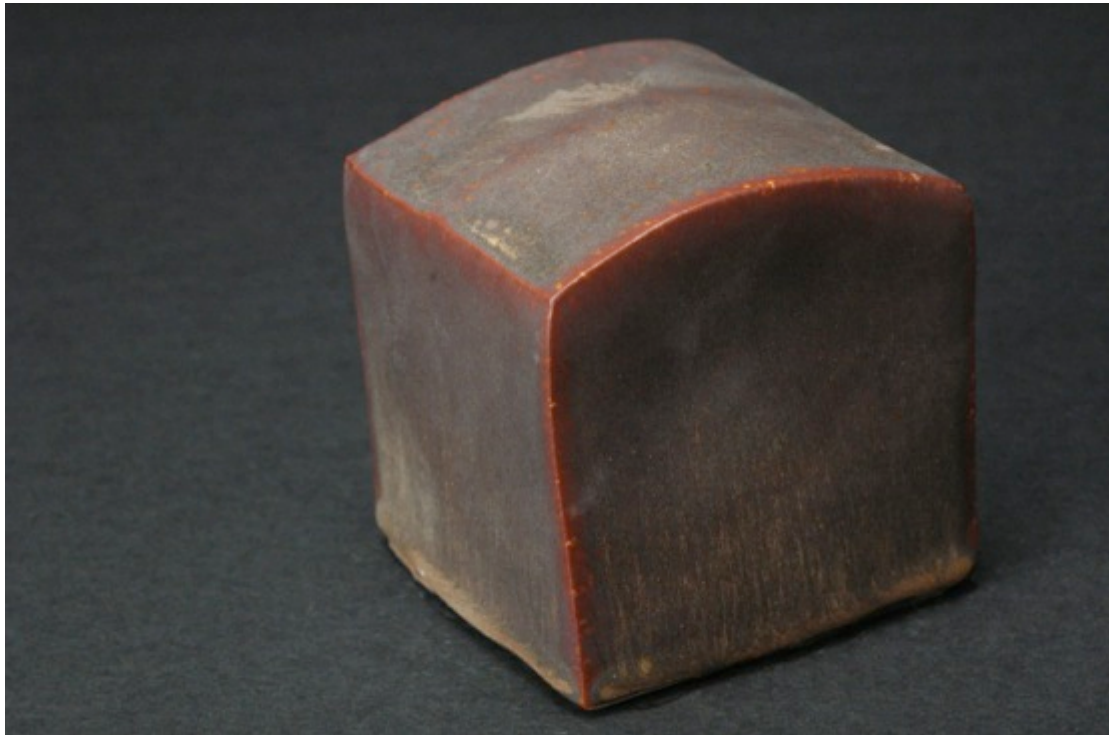
TNSCB 16 5Ti 10Fe, reduction firing, Cobblestone Nr. 71
