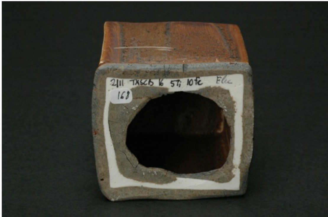
TNSCB 16 5Ti 10Fe, neutral firing, Cobblestone Nr. 168
