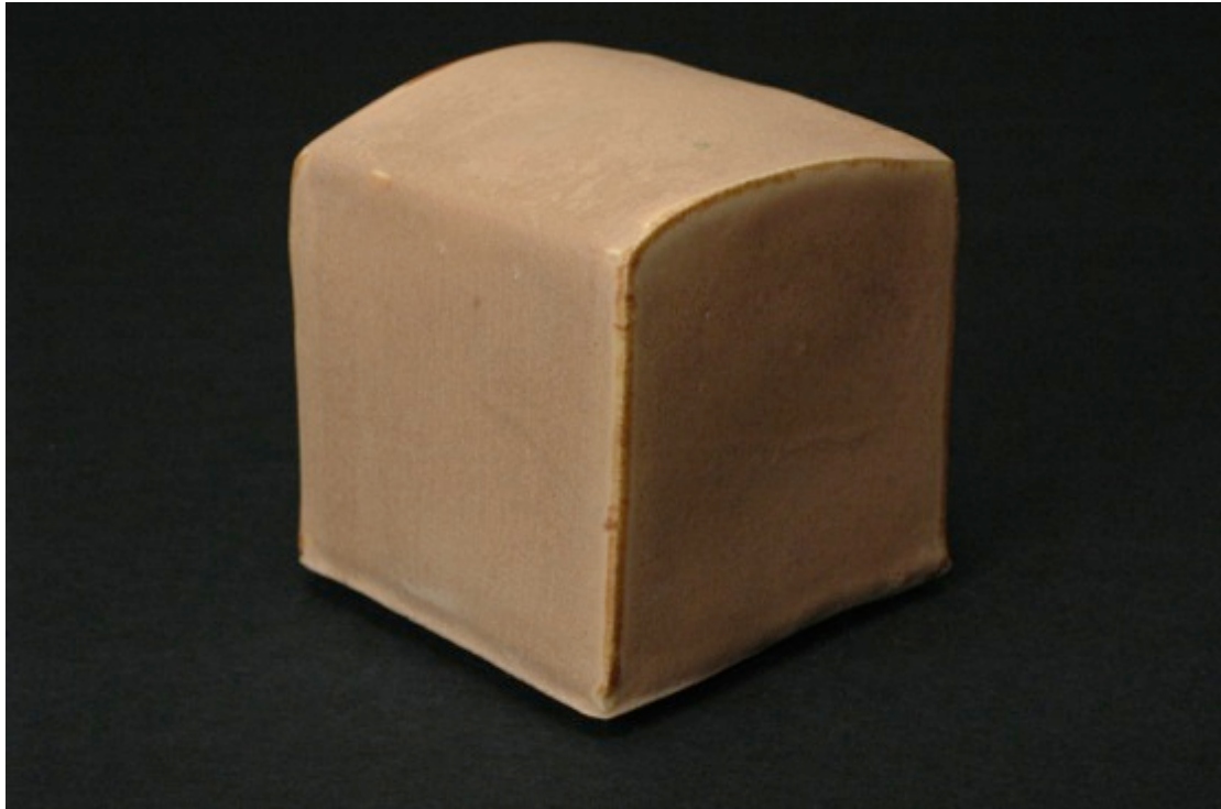
TNSCB 16 5Ti 7Fe, neutral firing, Cobblestone Nr. 35
